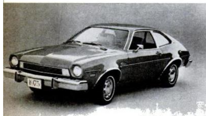
Pinto has 2.4-liter, four-cylinder engine, solid-state ignition and steel-belted radial tires as standard.
