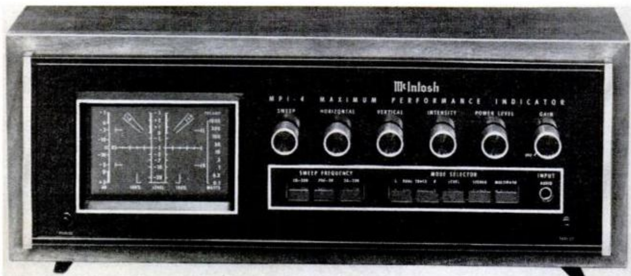
McIntosh MP1-4 , $600, is stereo only, but has dual-trace viewing, direct power readout, other unique features.
