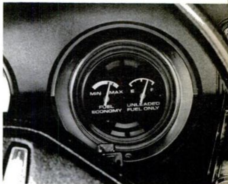
GM fuel economy meter is engine vacuum gauge, with readout in the dashboard instrument panel.
