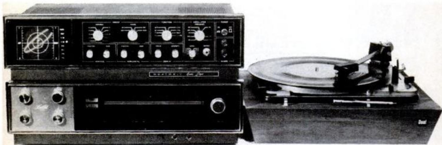
Audio scope styling blends well with stereo gear; Heath scope and receiver shown are close match. Test shown here is tone-arm antiskating adjustment.
