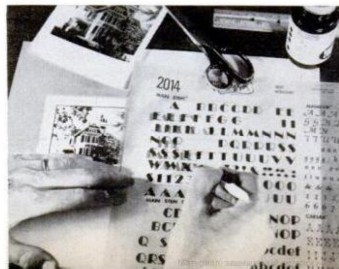
Combining greetings and photo on one negative for easy, one-step printing takes time in the beginning, saves it in the end. Here, greetings are lettered with Prestype onto high-contrast print (see text); reshooting on high-contrast film results in negative (above) from which you can make as many prints as you like.
