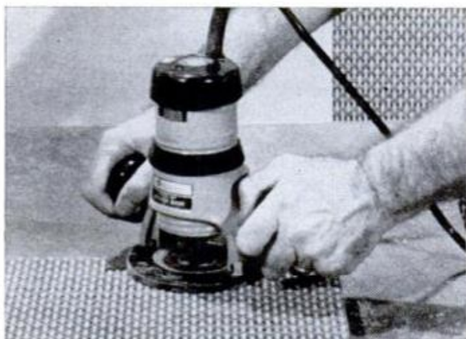
Router equipped with carbide-tipped straight cutter is used to trim overhang. Edges are then beveled.
