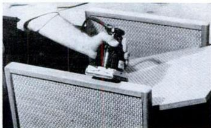
11. Final sanding of trim is done with trim on chair. Start with 120-grit paper; finish with 220 grit.
