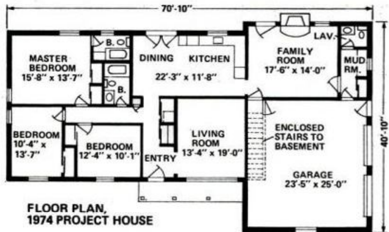
Three-bedroom ranch house was built by class over period from fall 1972 to spring 1974. Features include double-glazed windows, electric appliances and heat, French doors at rear, fireplace.
