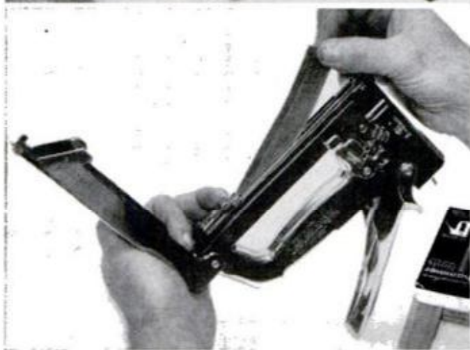
Casing can be applied using gun. Notice left-hand position to keep gun's shoe flat against the work surface.
