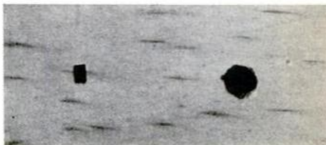
Test comparing countersunk Whammer nail and 4d finishing nail set with nailset. Former is less obvious.
