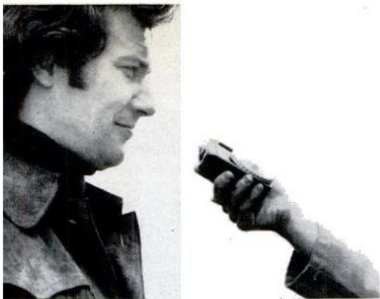
Meter reading taken from face gives maximum detail, but darkens skin. Usually it pays to open up 1-2 stops.
