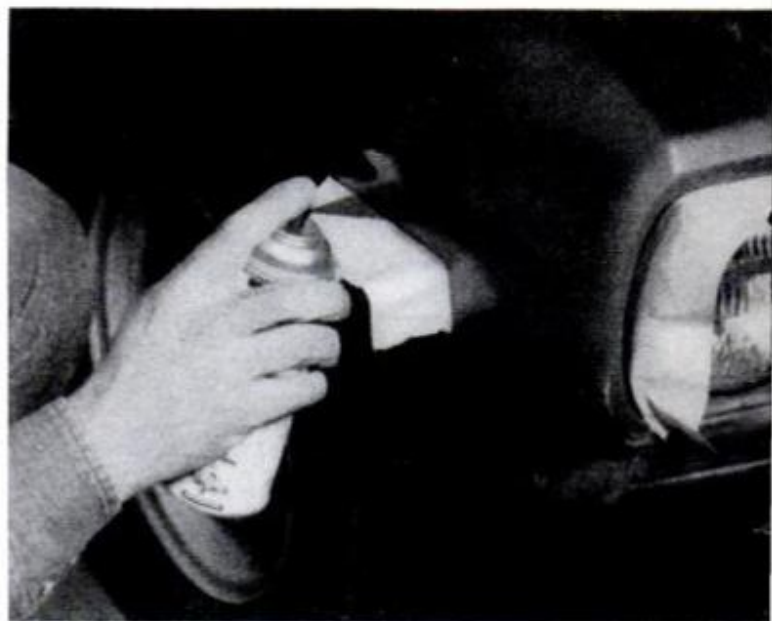
10. Apply primer to the repair area. It's a good idea to practice your spraying technique on a tin can first.
