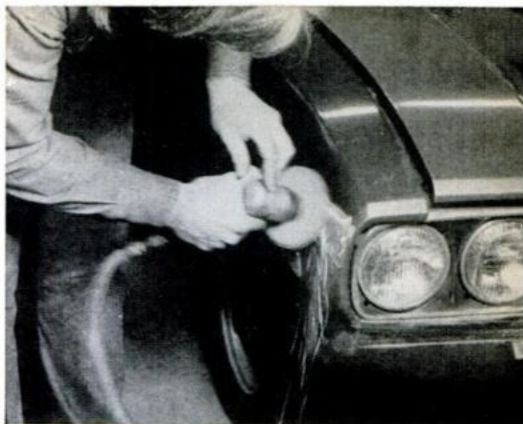
3. Grind area around dent down to the bare metal with electric drill; here pro uses compressed air grinder.
