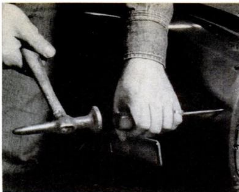
1. Punch a hole in the dent for special tool if there's no other way you can get behind it to push it out.
