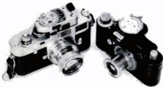
Clip-on meters can also be hand-held; $87 Leicameter (left) couples to M-model Leicas, $19 Vivitar 24 fits any camera with accessory shoe (but too loosely).
