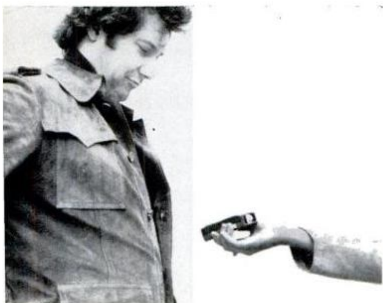
Incident reading (note meter pointed back toward the camera) usually provides balanced overall results.
