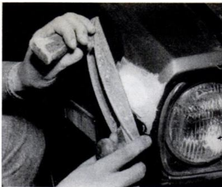
7. Shaping tool such as a Surform is then used to remove the excess filler before sandpapering the spot.
