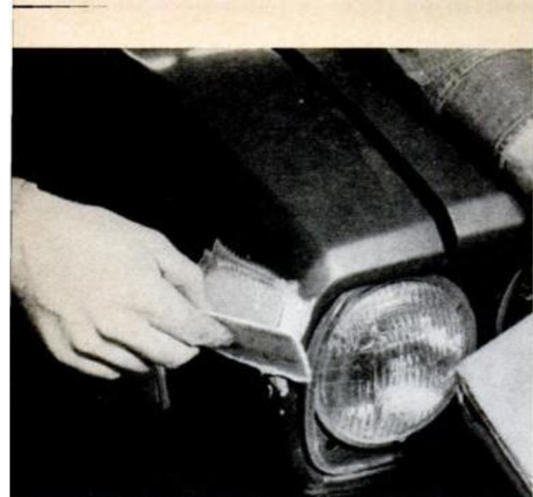
6. Plastic filler should be applied one layer at a time, and built up until it is slightly higher than the body.
