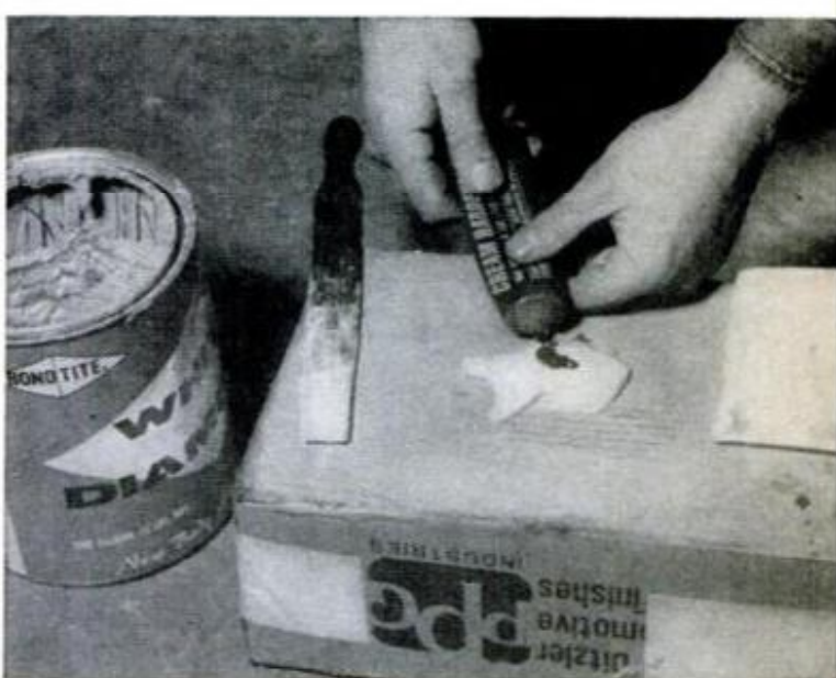
5. Add cream hardener to the plastic filler, and mix them thoroughly. The applicator comes with filler kit.
