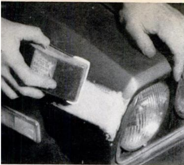
8. Sand the repaired area until the plastic filler is brought down to the level of the surrounding area.
