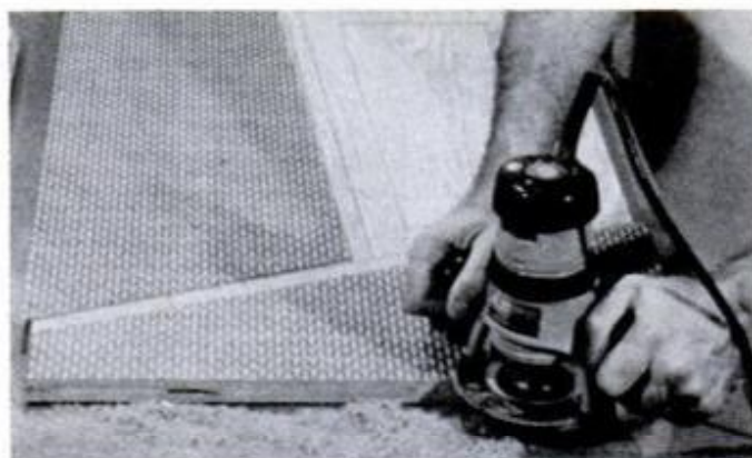
4. Last disassembly is made so that the router can be used to trim overhanging laminate from all parts.
