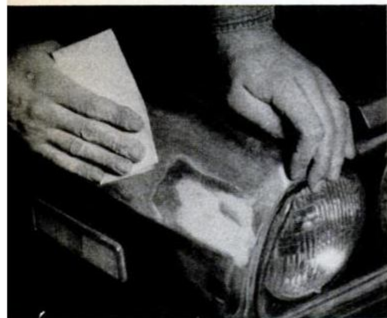
9. To feather-edge the repair, sand from body paint into the repair area. Don't press down too hard!
