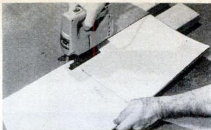
2. Laminate is cut from the back using taped-on pattern as a saw guide. Notice the pattern orientation.
