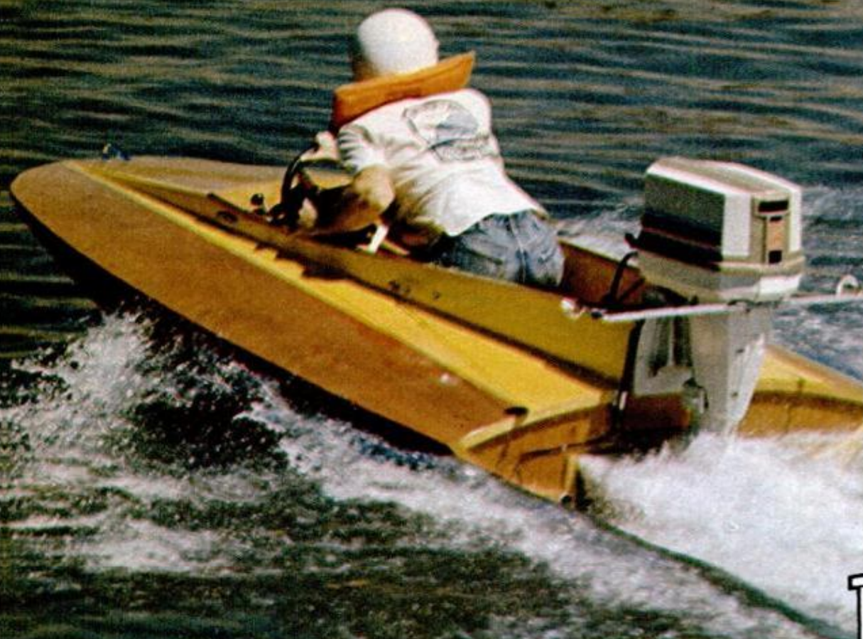
Slot-riding on a center channel of air, the tunnel hull planes on both hydro and aerodynamic lift for minimum wetted surface drag, maximum speed on flat water.
