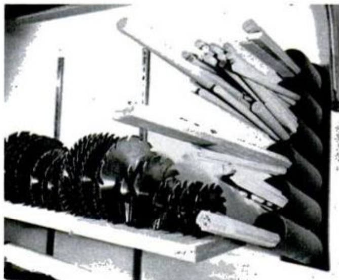
Two storage tricks: Blades lined up in kerfs in shelf; dowels stored in wall-mounted cardboard mailers.
