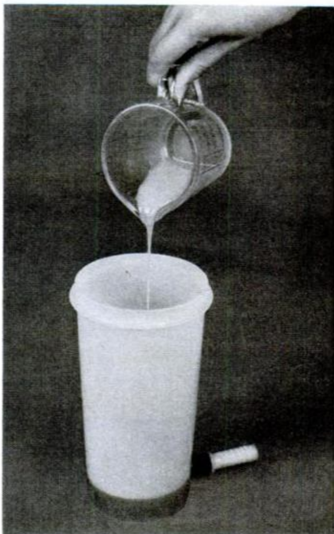
Container here has pipe and nails installed and properly positioned, hole sealed and coupling inserted into pipe. Epoxy will later cover this assembly.
