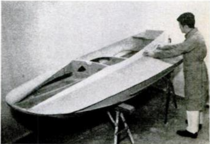
Final decking panels are fitted in same manner as hull panels. Inner contour which butts cockpit coaming is marked to fit along carling before coaming goes on.
