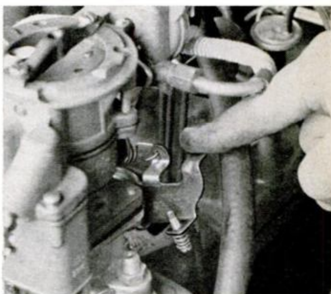
Choke plate may not move because it is engaged by the choke unloader. Pull back on tang to check.
