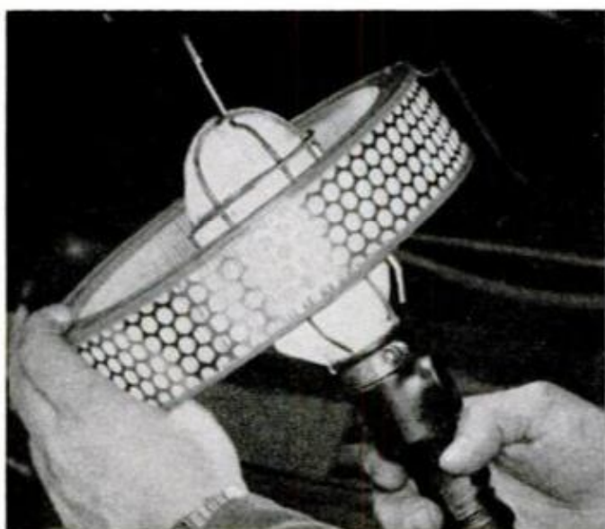
Air cleaner should be your first check, and, as shown on opposite page, choke plate should move freely.
