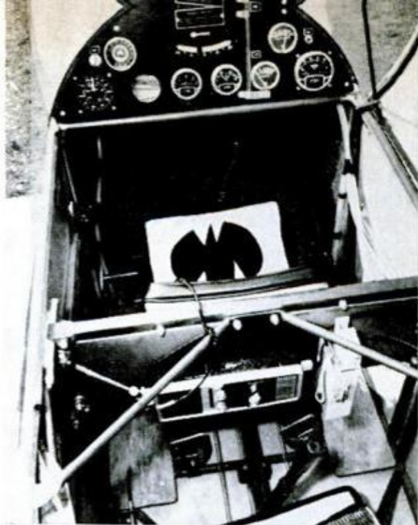
Rear cockpit of two-seater version (above) has no instruments except radio. Ship is flown solo by pilot looking over bulkhead at front instrument panel. At left is single-seater cockpit.
