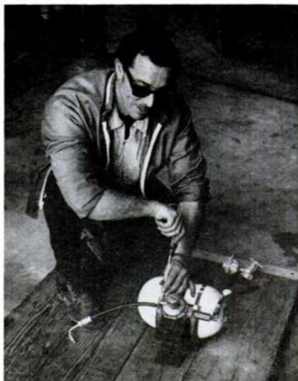
Dick Gotelli's clean machine started life as a conventional Honda street bike. Photo of the bike (left) shows propane tank where gasoline tank would normally be. Below: Dick removes tank from the cradle he fabricated for it.
