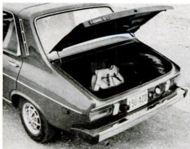
Trunk is roomy with flat floor; spare stands upright and is neatly covered to keep luggage clean.
