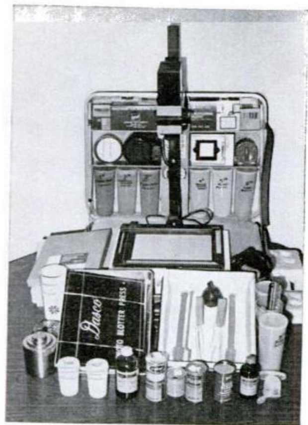
Unbelievable amounts of darkroom gear can fit; compact, take-apart enlarger is the key item.
