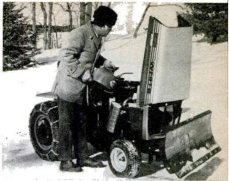
Author refuels the Yard Boss GT-1650 during cleanup of his driveway. Gas tank, battery and air cleaner are all easy to get at under tractor's hood.
