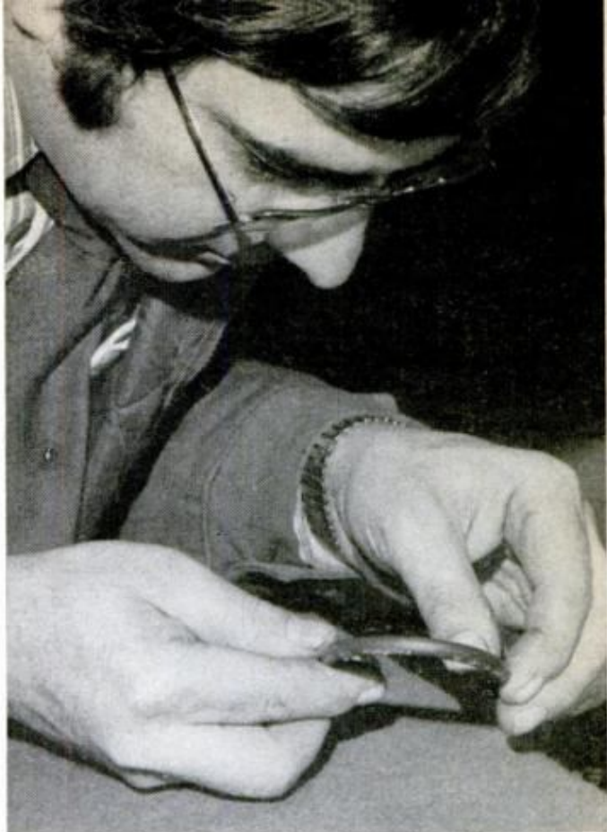
Look closely at cables for cracks and frayed areas, and gently bend them to check for brittleness.
