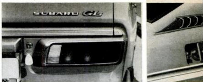
Same key fits all locks, including the off-center trunk; as well as the gas filler and doors. Flow-through vents exhaust via louvered ports in C-pillars.
