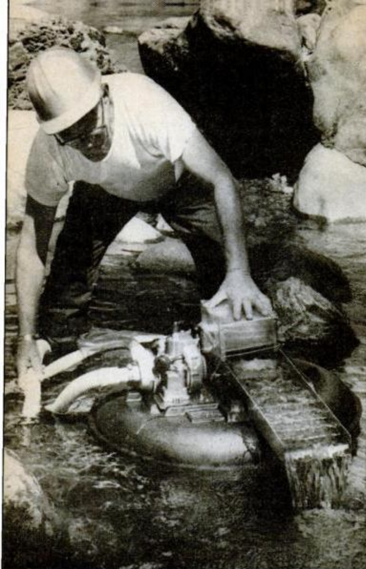
Mini-Dredge , from Keene Engineering, is light enough at 28 pounds to backpack in. Vacuumed gravel washes down riffle gratings of flume.
