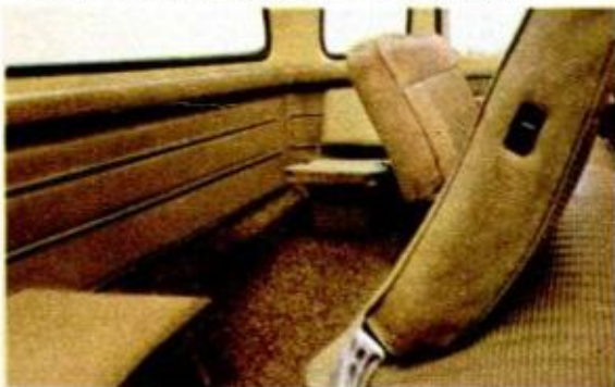
Jump seats (optional) have foam-padded cushion and back, fold out of the way.
