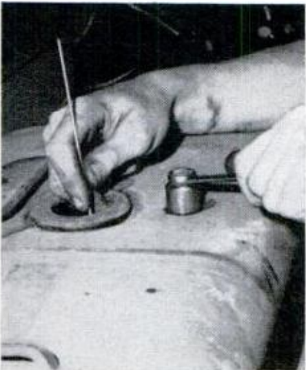
Chassis punch is mounted in position ready for cut by using the fuel-gauge hole for access.
