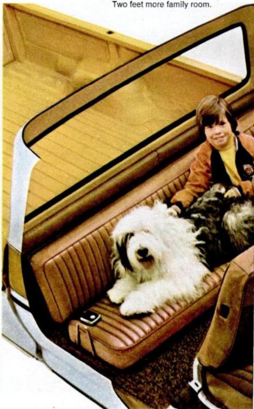
Jump seats (optional) have foam-padded cushion and back, fold out of the way.
