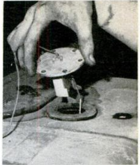
Remove the sending unit that transmits fuel level to gas gauge.
