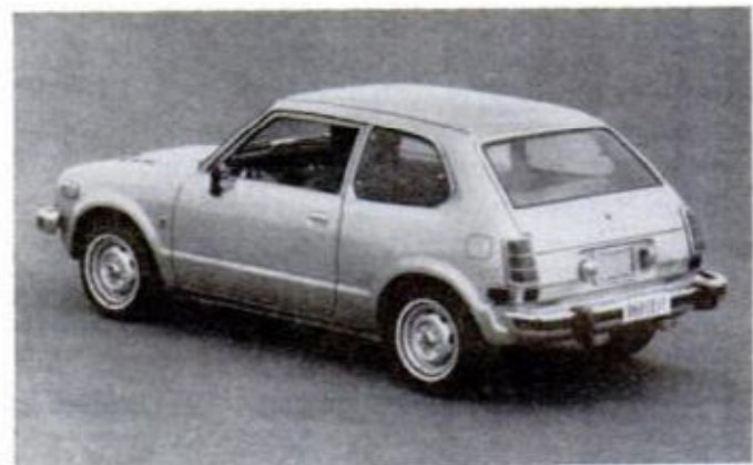
Rear quarter pane flips out for better ventilation; drip rail keeps rain from coming in. Airconditioning may be ordered, as may semiautomatic transmission, but performance and fuel economy suffer with these items.
