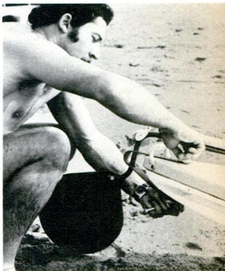
Single bolt attaches the rudder to the tiller. When rudder strikes the ground, it pivots upward without damage, lets you ride sailboat right up onto beach.
