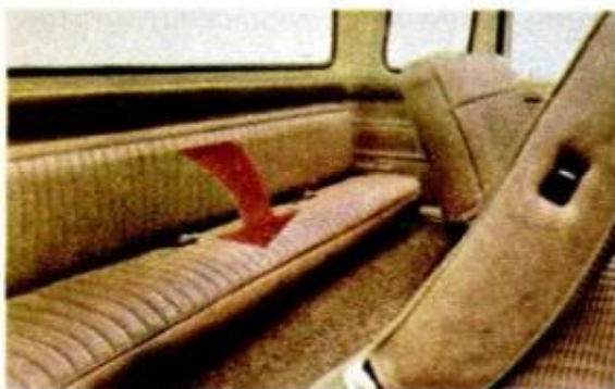
Foam-padded rear seat (optional) folds down to make a flat floor for cargo.
