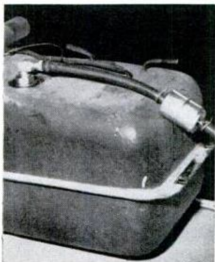
Gas line and fuel filter are connected to Pacemaker before the tank is replaced on car.
