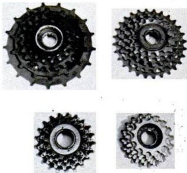
Gear-ratio comparison: Top left is wide-ratio Shimano 14-34-tooth freewheel. Top right: medium-high-ratio Maeda 14-28-tooth freewheel. Lower left: Cyclo medium-low-ratio freewheel, 14-21 teeth. Lower right: Regina six-speed, low-ratio cluster with 13 to 19 teeth.
