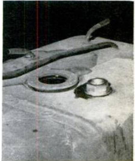
The Pacemaker valve is shown mounted in place. Follow technique shown below left for installing.
