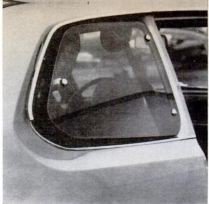
Rear quarter pane flips out for better ventilation; drip rail keeps rain from coming in. Airconditioning may be ordered, as may semiautomatic transmission, but performance and fuel economy suffer with these items.
