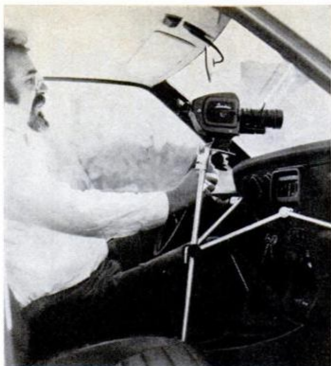
Bolex Minipod again, here braced against a car dashboard for over-the-hood shots. Adjusted differently, it can hook over bumper for low-angle dolly shots.
