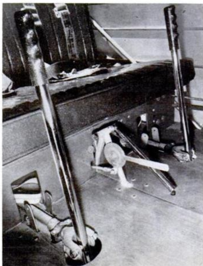
Wide cockpit seat and twin sticks are shown above and at right. Center lever between sticks is trim control. Instrumentation looks skimpy, but actually includes everything needed for VFR daylight flying.
