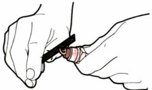
Make several passes with a file to get rid of deposits and to brighten the two electrodes.
