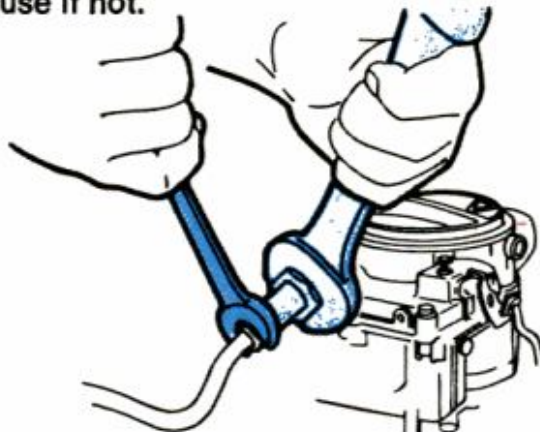
To remove an integral fuel filter, disconnect fuel line and filter nut. Filter lies in the inlet.
