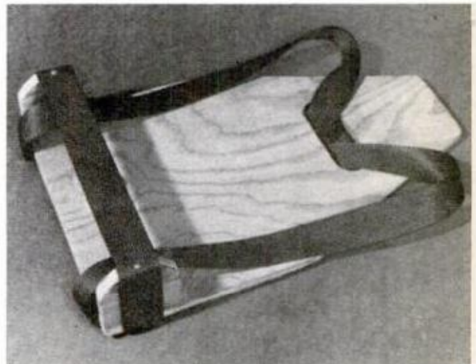
Body side of pack board shows hip strap stretched tightly across cleats and attached with roundhead screws. Shoulder strap passes under hip strap.
