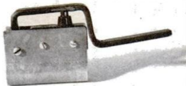
Switch handle is bent from 1/4-in.-sq. steel so that it will pass around microswitch. Pivoting hole is made by soldering a short length of brass tubing to the steel handle.
