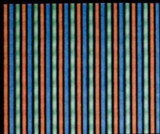
Sony Trinitron's phosphor stripes show no shadows since mask has only vertical strips. Tube face curves only in one plane, an antireflection plus, Sony says.
