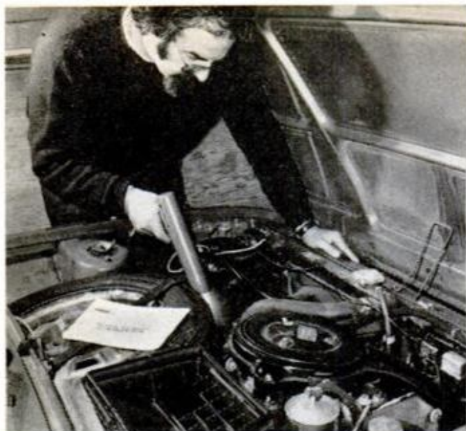
Stroboscopic timing light , flashing in sync with spark, "freezes" moving timing marks.
