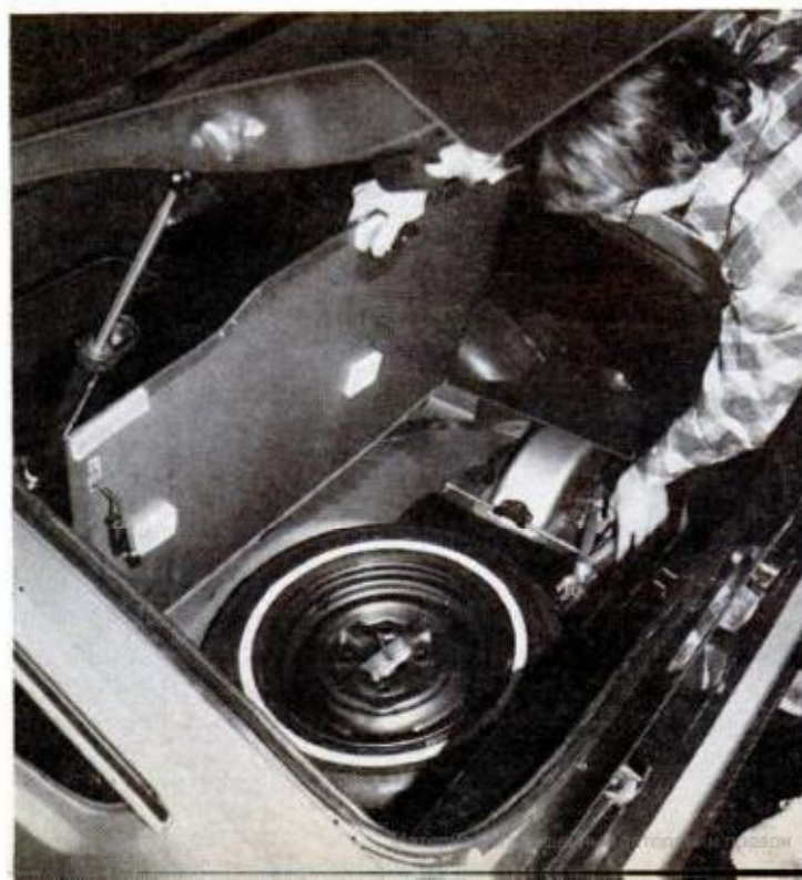
B-210 engine is ohv Four, displaces 1288 cc and nets 67 bhp. Torque works well with manual transmission, is weak for automatic. Spare tire and tools rest under floor of hatch compartment.
