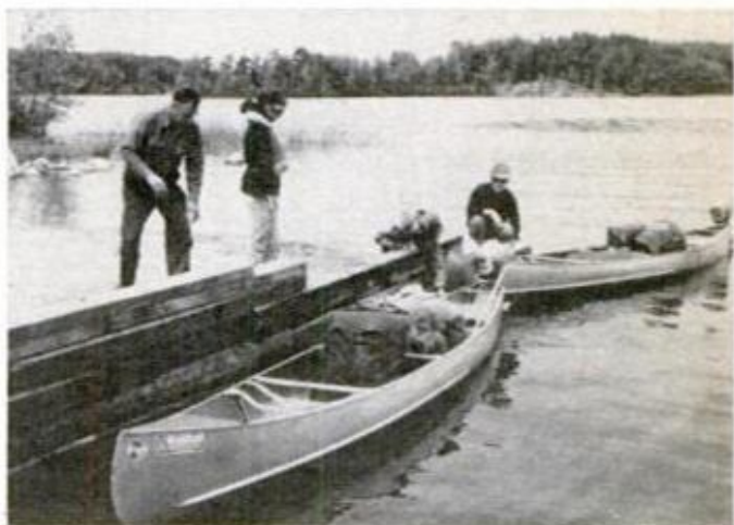
Rushton (above) from Old Town Canoes, is 18-pound fiberglass copy of old classic one-man pack model of only 10½-foot length. Grumman rental square-stern aluminum canoes (below), packed for camping, have Y-shaped transoms for mounting small outboards. Old Town 16-foot Wahoo (bottom) is shown rigged with sliding rowing seat; sails with leeboards or daggerboards may be added.
