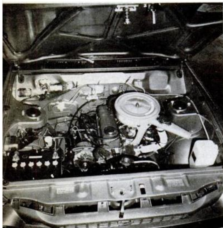
B-210 engine is ohv Four, displaces 1288 cc and nets 67 bhp. Torque works well with manual transmission, is weak for automatic. Spare tire and tools rest under floor of hatch compartment.
