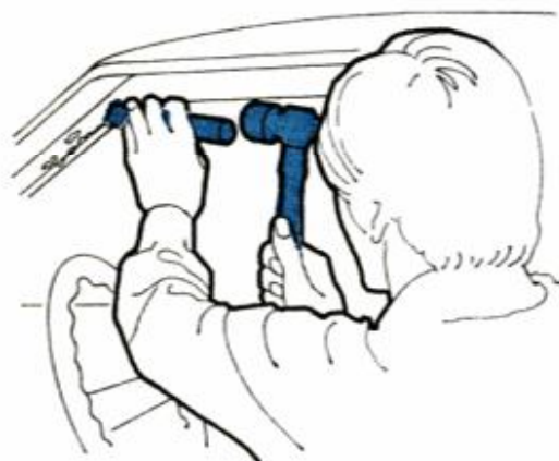
Cut off solder lumps and high spots that keep weatherstripping from sealing with chisel.
