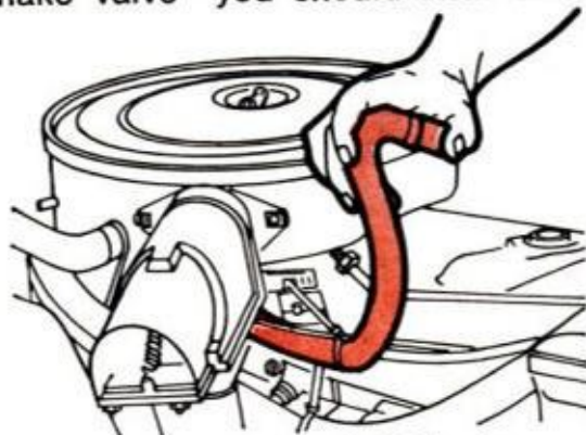
Check operation of PCV valve.
