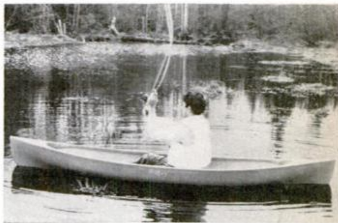
Rushton (above) from Old Town Canoes, is 18-pound fiberglass copy of old classic one-man pack model of only 10½-foot length. Grumman rental square-stern aluminum canoes (below), packed for camping, have Y-shaped transoms for mounting small outboards. Old Town 16-foot Wahoo (bottom) is shown rigged with sliding rowing seat; sails with leeboards or daggerboards may be added.
