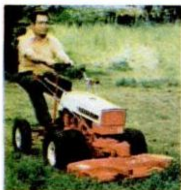
Instant forward-neutral-reverse. Detachable sulky attachment for convertible tractor lets you walk or ride.
