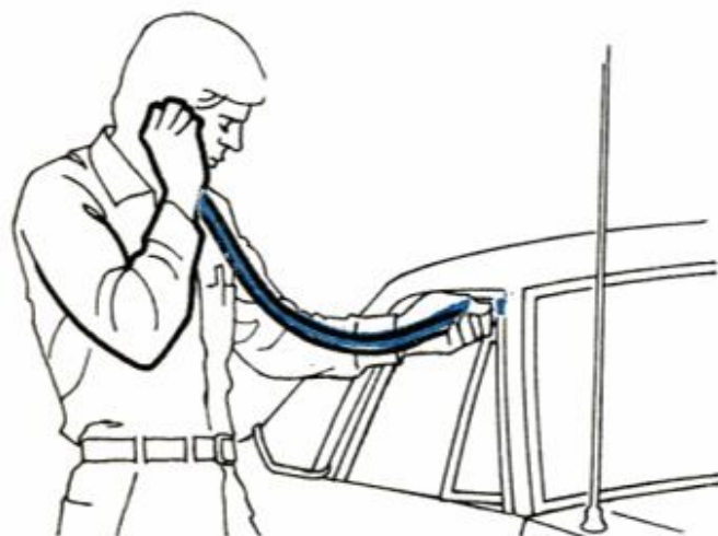
If air is leaking from inside to outside, you will hear hiss with improvised stethoscope.
