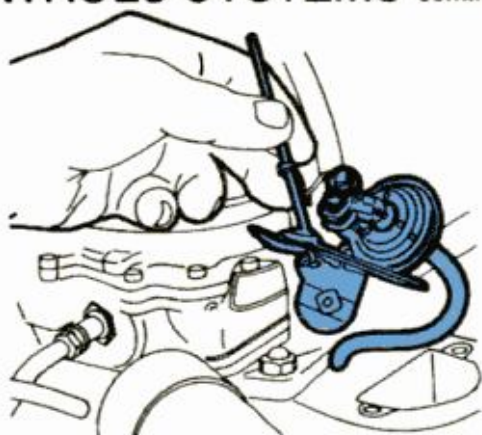
Control of manifold-type choke is found inside the well housing.
