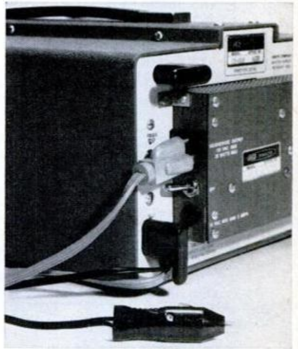
Bolt-on inverter kit lets a.c.-powered Heath scope run from car battery via lighter socket.
