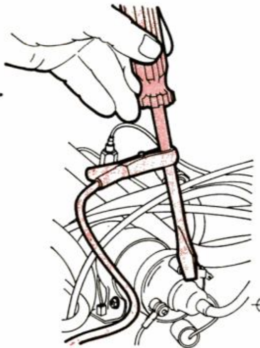
Use jumper to test distributor-to-coil and sparkplug cables.
