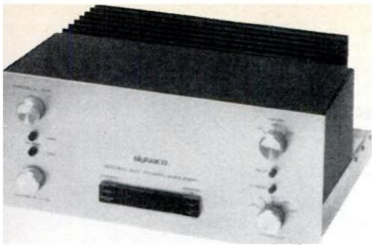
Clean-styled Dyna is massive (note 6-inch ruler, for scale), with heat sinks so deeply finned Dyna warns not to use them as a record rack. Shelf at side of heat sink can hold accessory fan in close quarters.
