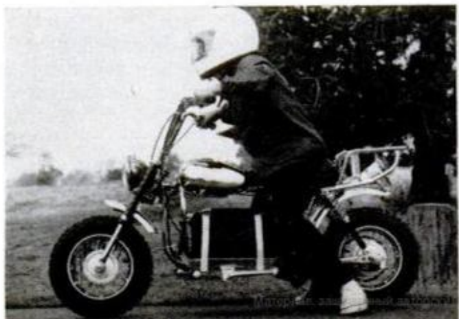
The Charger electric cycle is quiet, pollution-free and, best of all, needs no gas. The $500 machine is 62 inches long on a wheelbase of 45 inches, is 37 inches high overall and weighs 210 pounds with batteries.
