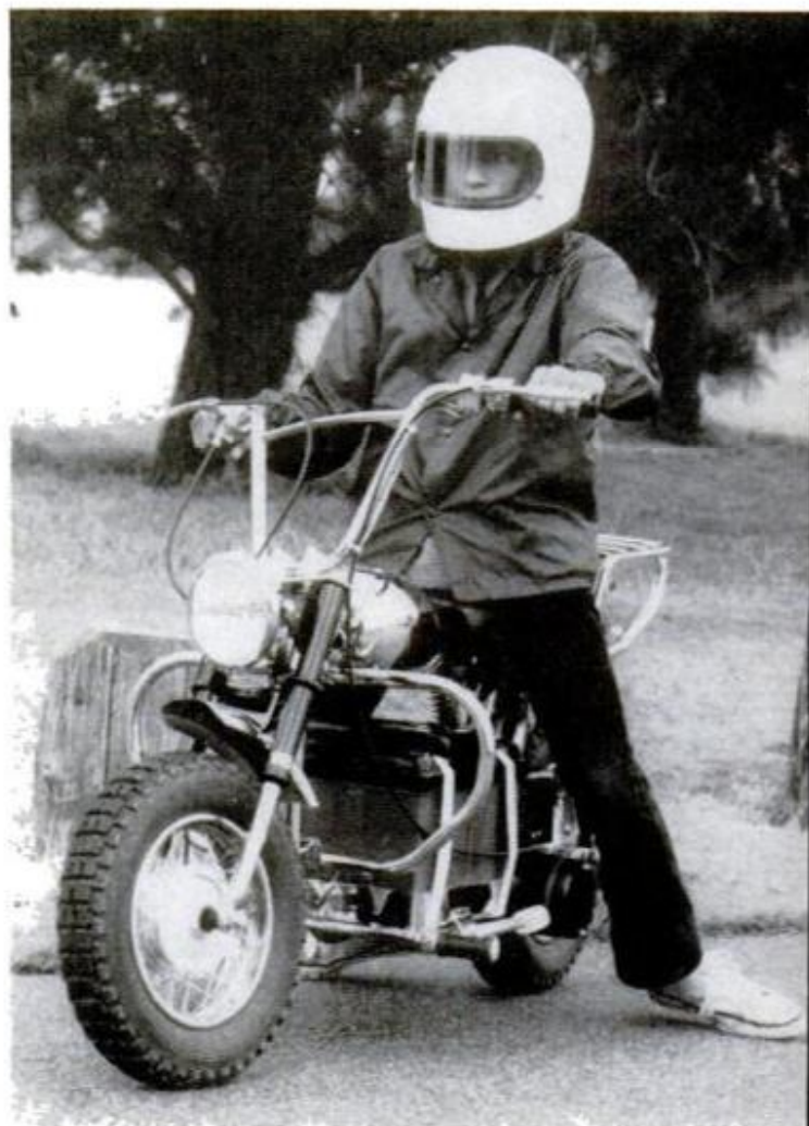
The Charger electric cycle is quiet, pollution-free and, best of all, needs no gas. The $500 machine is 62 inches long on a wheelbase of 45 inches, is 37 inches high overall and weighs 210 pounds with batteries.
