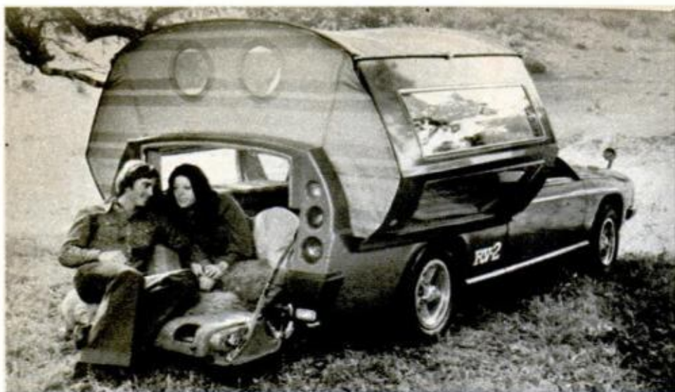
Futuristic experimental station wagon "Camp(or) Car RV-2" from Toyota makes its Mark II into a prototype that opens into a test model with interior eating or sleeping space for four. With sides swung out, tent top and sides enclose compact camping area. Unit may suggest models for future marketing.
