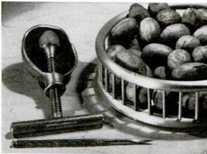
Basket made from \frac{3}{8} -in. seamless aluminum tubing and aluminum nails makes attractive server.
