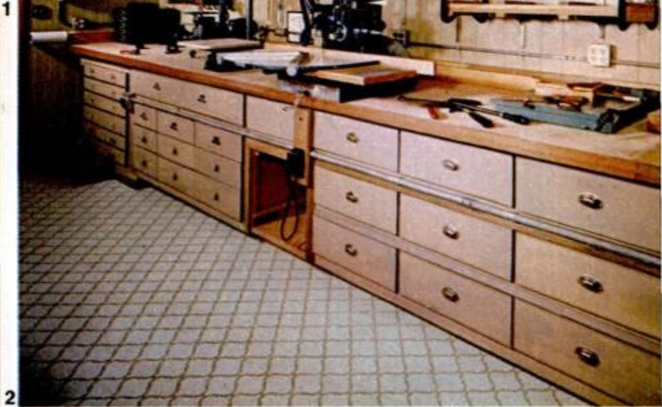
1. Overall view of narrow shop from double doors (see plan below). Good stunt used by Baskin: Radial-saw table is over workbench surface, old drill-press table supports work being cut. Thus, materials and tools (Surform tools here) needn't be moved from bench when piece of stock is cut. 2. View from opposite end of shop shows how owner gets good use of limited space. Ceiling over bench is dropped to gain storage above. 3. Shallow cabinets over 16-in.-wide bench.
