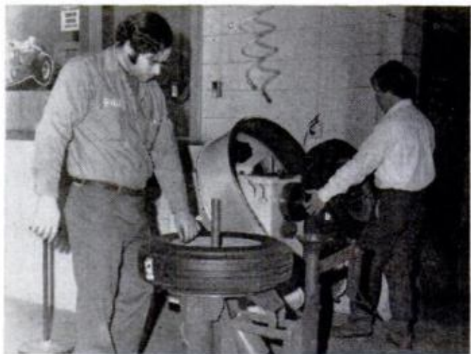
Wheel and tire assemblies should be balanced when old tires are remounted or new tires are purchased.
