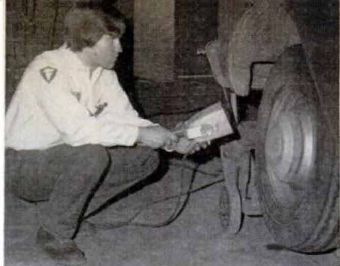
Dynamic wheel balancers check balance of a spinning wheel; this one works like stroboscopic timing light.
