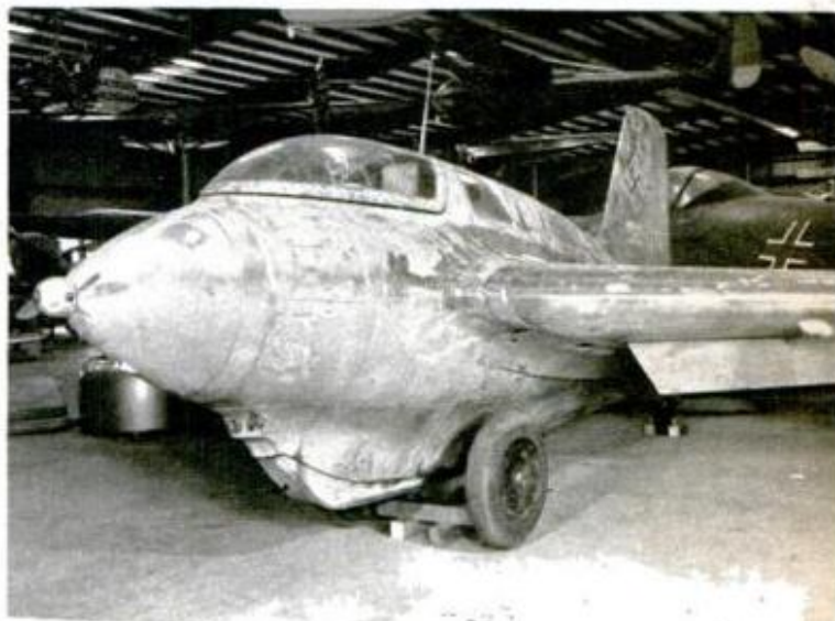
Short-lived but devastating , this first rocket fighter was developed by Germans near end of World War II. Capable of only few minutes' flight, the ME-163-B could reach 35,000 feet.
