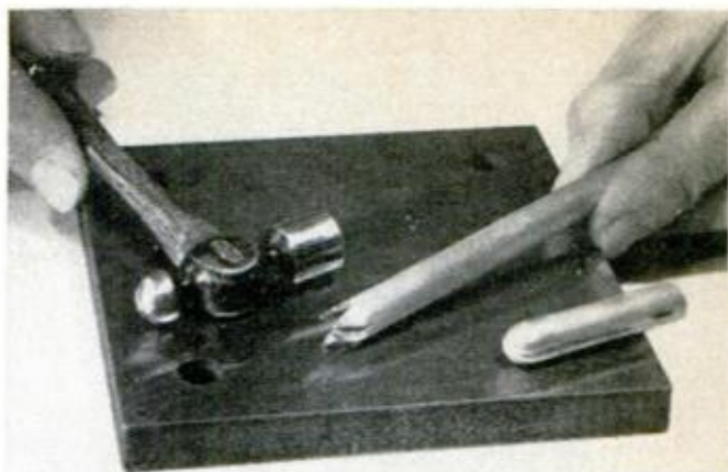
Aluminum tubing can be closed and rounded by cutting as shown and lightly tapping the cut ends.
