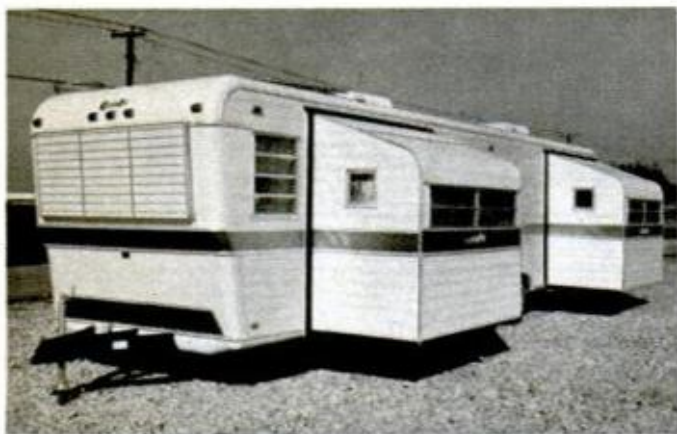
Twin tilt-outs are provided by Newmar Kountry-Aire and others for expansive living space for owners spending extended time at one campground. Fifteen-minute setup is claimed.
