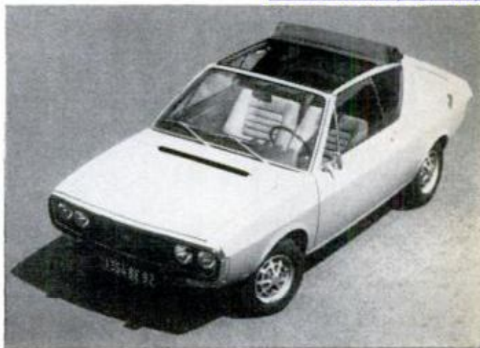
Renault 17 TL Coupe Convertible: Fiberglass hard top is removed; soft top underneath can be opened, closed.
