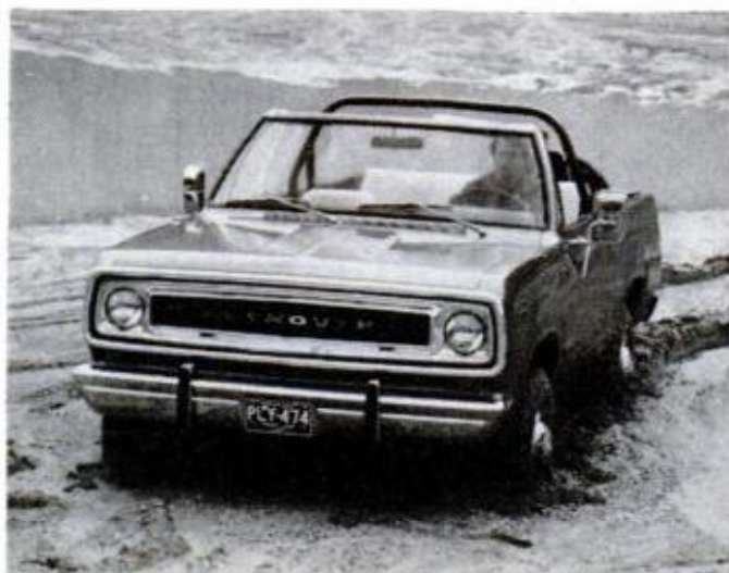
Plymouth Trail Duster is four-wheel-drive addition to famous line. Dodge will also have a Ramcharger. Options will include soft, hardtops, 313 or 440 V8.
