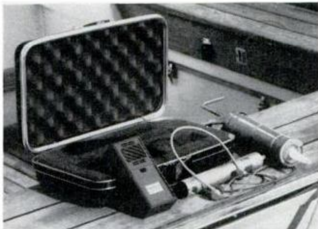
Complete kit includes leak locator, tone generator to transmit from far side of any solid material, earphones and focusing extension slip-on to localize voids.
