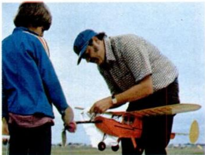
Contestants ready rubber-strand motor. Ordinary hand drill is used to get powerful strands as tightly wound as possible. This plane was a winner.
