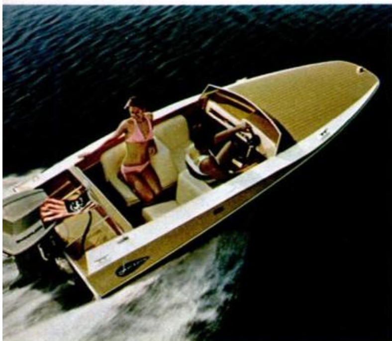
Larson LX-5 is high-styled sport runabout addition to Larson's 20-boat fleet. Rated for up to 95-hp outboards, 1150 lbs. capacity, this ski-boat has modified V-hull, metal-flake finish, optional stereo.
