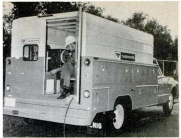
Data from the pig's sensors are relayed by cable to mobile unit, where readouts are recorded.
