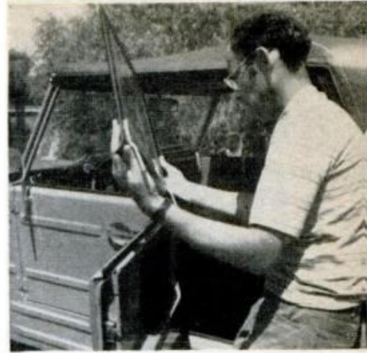
Side curtains' metal rods poke into holes in doors. With all curtains in place, ventilation suffers and the windshield fogs.
