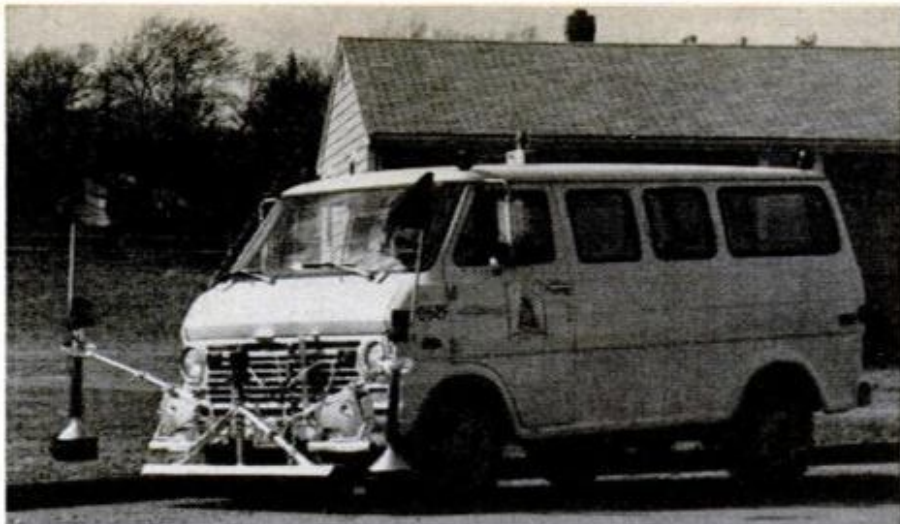
surveys are carried out with mobile leak plotter (right), capable of covering 400 feet per minute.
