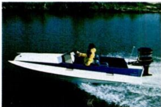
Starcraft Stinger 19 (top) wraps windshield around cockpit of this ski-boat 19-foot line leader. It's available as an outboard for up to 190 hp, or with I/O or water-jet-power push of as much as 350 hp.
