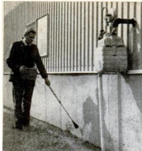
This portable flame-ionization unit (left) has proved to be a supersensitive detector of natural gas. Street
