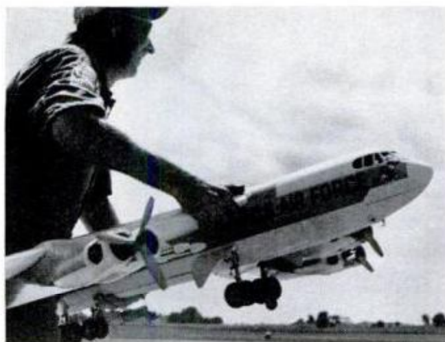
In flight, B-52 model looks like the real thing. Fast-spinning props aren't noticeable, giving plane jet look. Engines must be synchronized for proper flight.
