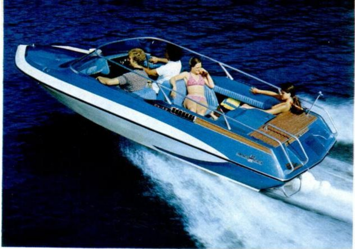
Sporty CV-18 S/S Glastron/Carlson offers stern-drive or water-jet powering. Built-in steps in transom are desirable safety and convenience aid. Handrail circles cockpit; finish is metal flake.
