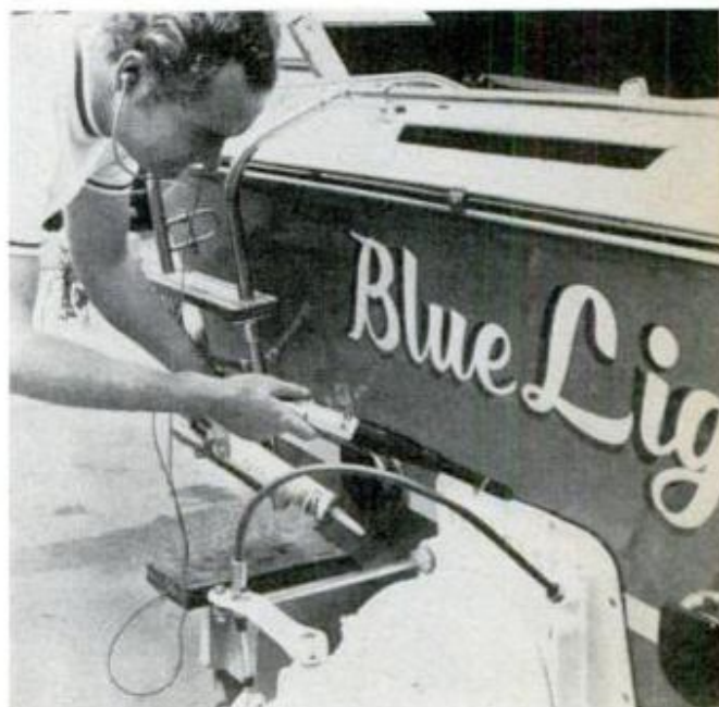
Complete kit includes leak locator, tone generator to transmit from far side of any solid material, earphones and focusing extension slip-on to localize voids.
