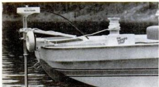
Weightlifter all-electric anchor hoist is newest bass boat (or any craft) accessory. From Motor-Guide Div., Hershede Hall Clocks, $100 12-v. unit lifts 190 pounds.
