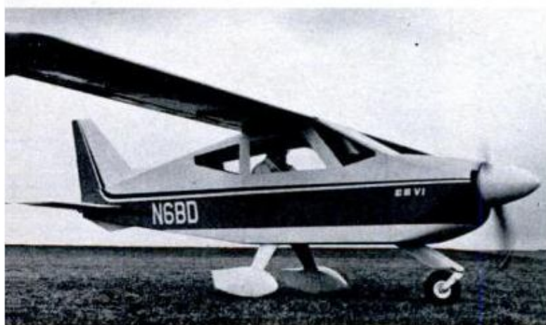
Super-aerobatic sport plane above is an original design by members of the Experimental Aircraft Assn. intended for advanced competition performance. Called Super Acro Sport, it's an outgrowth of EAA's earlier
