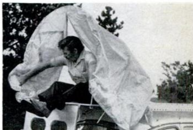
4 Setup is simple with ribs bowed into place and fitted into hole sockets in 1/4-inch plywood floor.
