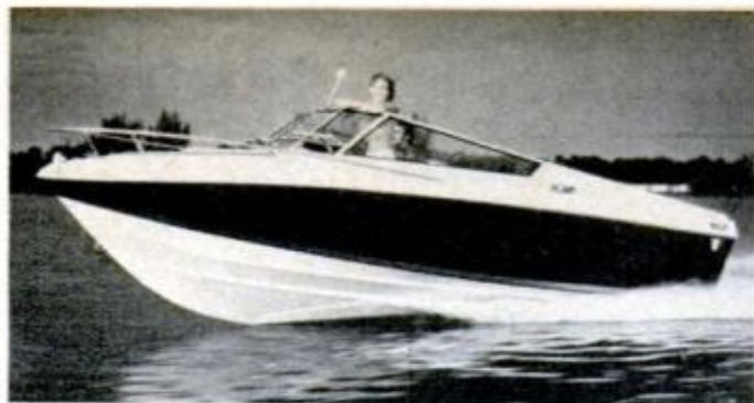
Wellcraft's Nova 21 is new slightly smaller model of style leader Nova 24. A deep-V offshore hull but with twin bunks forward, craft is rated for twin 140 I/Os.
