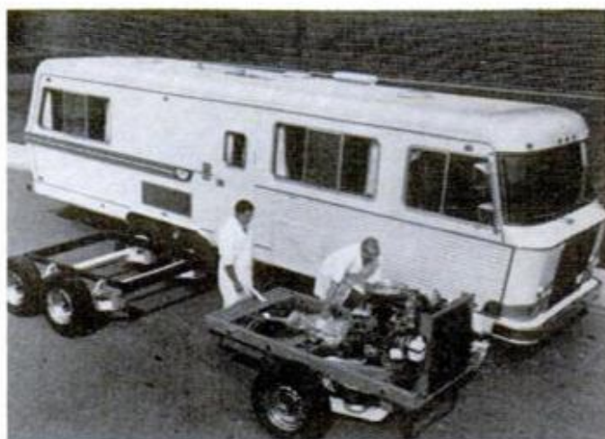
Pow-R-Pak is new front-wheel-drive motor-home chassis from AM General Div., American Motors. Holiday Rambler will be first to feature RVs with special unit.
