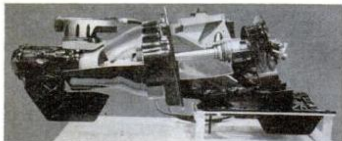
Power trim for jet drives is now option from Jacuzzi Jet Marine. Toggle switch at helm allows driver hydraulic control through 10° vertical arc of deflector.
