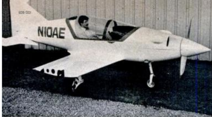
Needle-nosed beauty , still under construction, will soon be available in kit form for home assembly. Dubbed the "Eos," it comes with 55 or 70-hp engine, can hit up to 200 mph, climbs more than 2000 f.p.m., has retractable tri-gear, is a "hot" performer.
