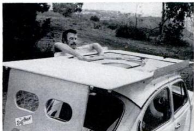
3 Flooring panel slides back to reveal storage compartment in base for rib-bows and nylon tenting.
