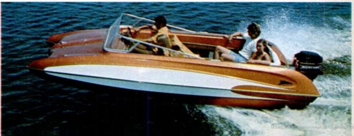
Tunnel-hull look is feature of Dolphin Corinthian from Dolphin Sport Craft, North Chicago, Ill. The 17-footer has been timed at 40 mph with 85-hp outboard. Runabout is rated for 150 hp.
