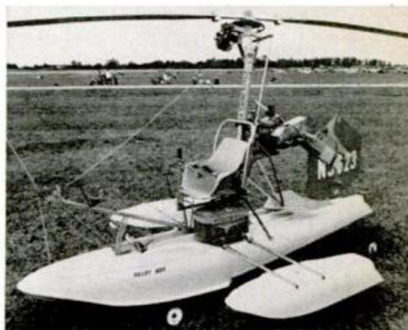
Fitted with floats, this amphibious autogyro can operate from land or water, was modified from a standard Bensen B-8M single-seater Gyrocopter kit by J. Hasselfeldt of Royal Oak, Mich. Cost, including the engine, fiberglass hull and outboard sponsons, came to $3200.
