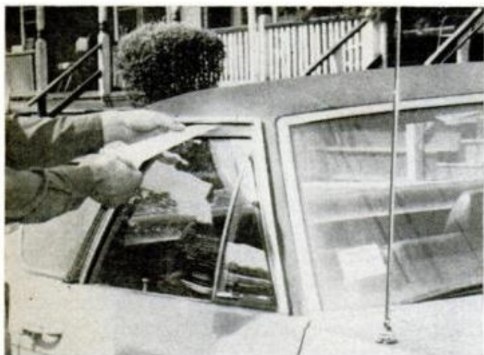
Check weatherstripping by closing the doors on strips of wrapping paper to see how snugly they're held.
