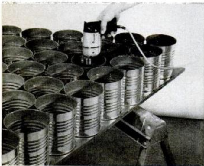
The 1/2-in. holes in bottom of cans are used as guide for drill when boring 1/2-in. holes through plywood.
