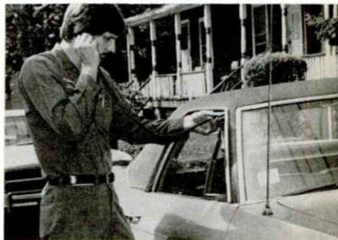
Air leaks can be detected with hose used as stethoscope. Car is closed tight with fan blower running.
