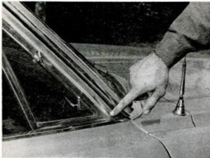
Rubber seals will most often "pucker" in the corners. Remedy is to carefully heat and smooth the rubber.
