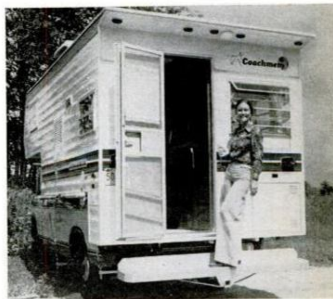
Extension Step Bumper for Chevy, Ford, Dodge, GMC and International pickups bolts on without welding, extends with camper mounted. From Kenco Engineering.
