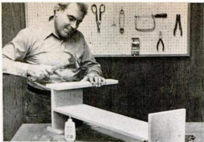
Nails are used to assemble bench temporarily, but for strength and rigidity, finish with screws and glue.
