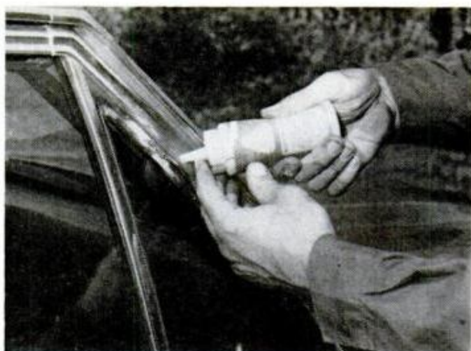
Window seals can be checked using a marking chalk that comes in a squeeze-type container (see text).
