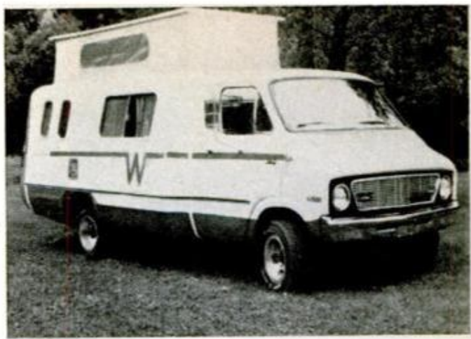
Winnie Wagon is latest in extensive Winnebago RV line. Van conversion raises roof for headroom, lowers it for garaging. Thermo-steel bodied unit will cost $6915.
