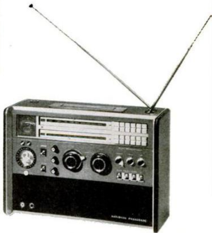
Panasonic's experimental RF-7000 24-band portable radio picks up AM, FM and SSB from 160 kHz to 230 MHz., with a motor-driven band selector and a world clock. It runs on battery, car battery or 100-240-v.a.c.
