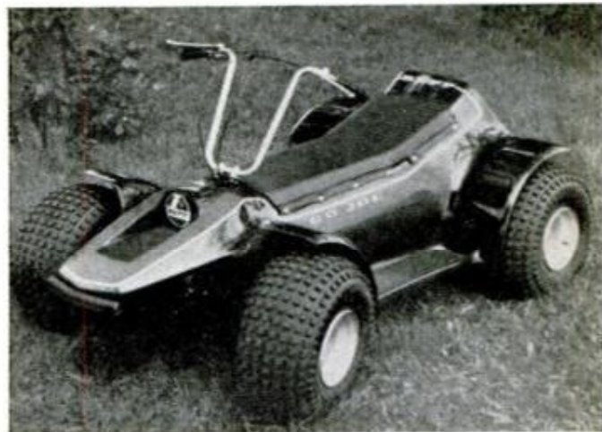
Go-Joe , a new four-wheeler from Rupp Industries, is claimed to be part motorbike, dune buggy, snowmobile, with speeds to 40 mph from a 2-cycle 8-hp Chrysler.
