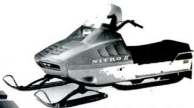
Rupp Nitro II provides 336-cc or 438-cc engines, twin carbs, CD ignition, aluminum rails.
