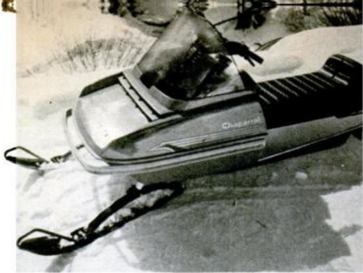
Chaparral Firebird , from Armco, has 22, 28 and 32-hp engine options. Liquid-cooled engines will be feature of new SSX 40 and 50-hp models.
