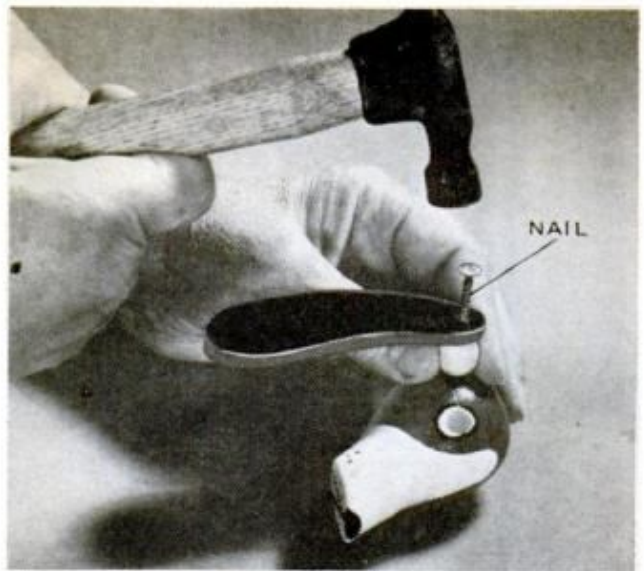
Attach ears to head by driving nails through oversize holes in ears, then through wooden beads.
