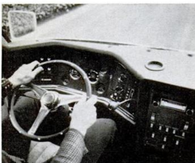
FMC starts by welding its own steel chassis, to which aluminum frame (left) is welded. Plastic conduits in center carry accelerator, brake and gear selector cables and heater hose. All joints on underbelly are sealed to prevent corrosion. Cockpit of FMC has good instrument array with panel at right supplying a digital readout on the coach's domestic equipment.
