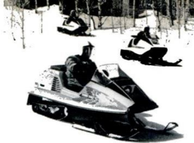
Raider, from Leisure Vehicles, has rear-mounted Canadian Curtiss-Wright engine, twin tracks, Double Eagle, Eagle and Hawk bucket-seat models.
