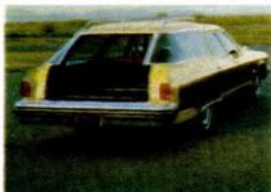
A tailgate on the Custom Cruiser that disappears into the floor.
