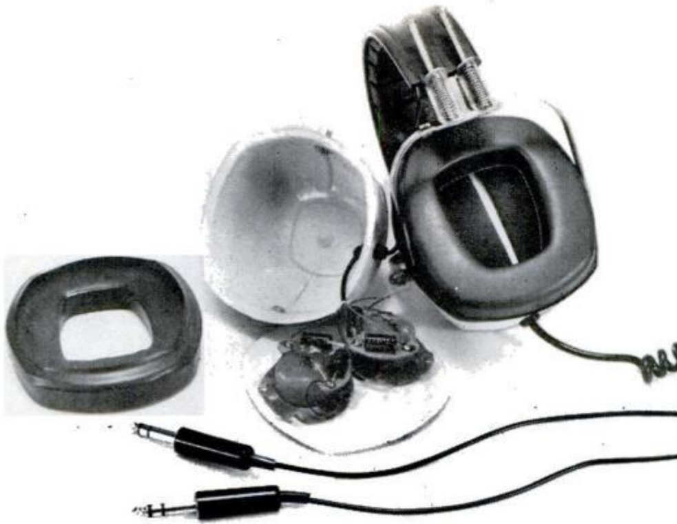
Inside a quadraphonic headphone like this Superex model, you'll usually find two small speakers angled slightly toward each other and facing the head: angles and the distance between speakers control sound perspective, construction of speakers; earcup controls sound quality. Fixler phones (facing page) are designed differently, have speakers aimed along axis parallel to the head's.
