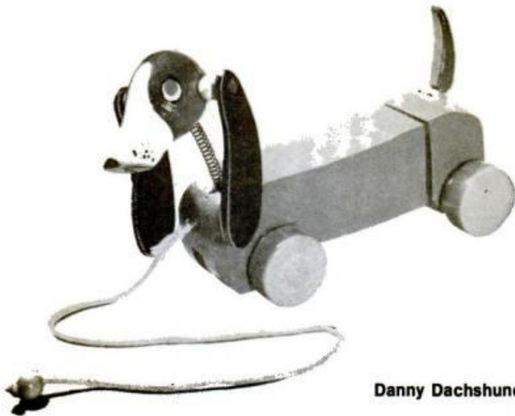
Attach ears to head by driving nails through oversize holes in ears, then through wooden beads.
