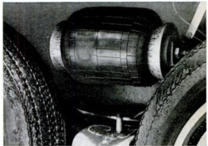
Air bellows is not concealed, is displayed as distinctive feature. Rear adjusts automatically to load under way, can be leveled at your campsite.
