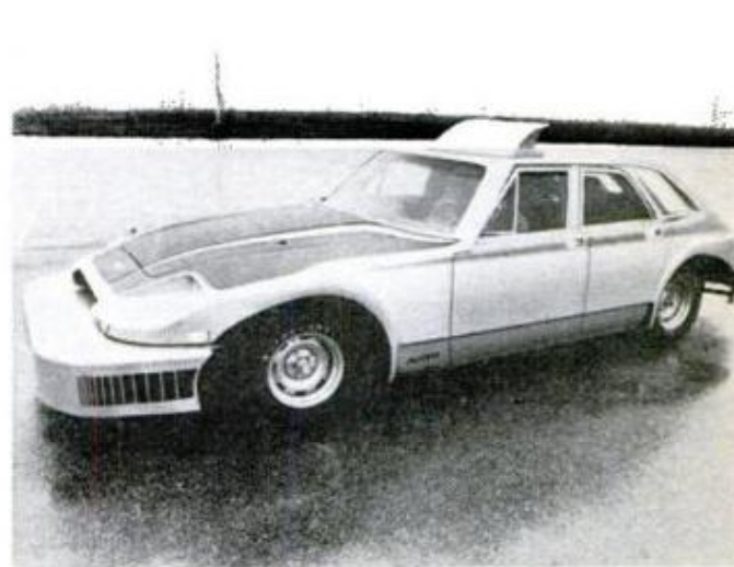
ESV from AMF uses a periscopic rear-viewing system that protrudes several inches from the roof. Its height enables it to provide the driver with a better viewing angle for objects close behind the car.
