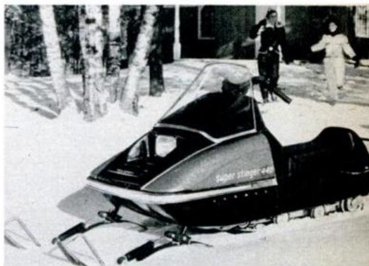
Scorpion Super Stinger 440 has Rockwell Twin 434-cc power, front shocks, speedometer, tach, flecked red styling, Para-Rail suspension, Power-Bite track.
