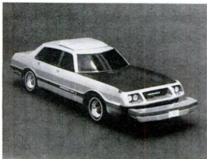
Experimental Safety Vehicle (ESV) from Fairchild prepared for the Department of Transportation includes a periscope installation that is aerodynamically integral with the roofline of the sedan.
