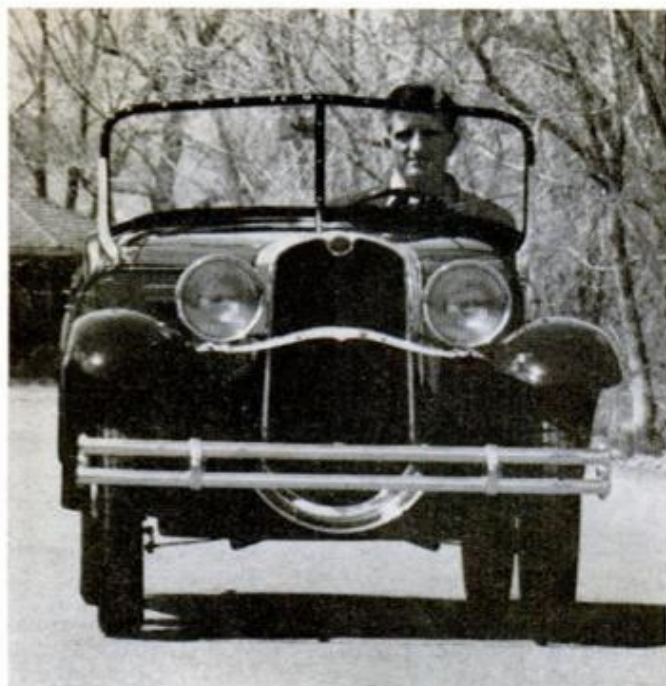
Front track of the roadster is 42.5 inches, and rear is 44.0 inches. The car sold for $315 in 1933.
