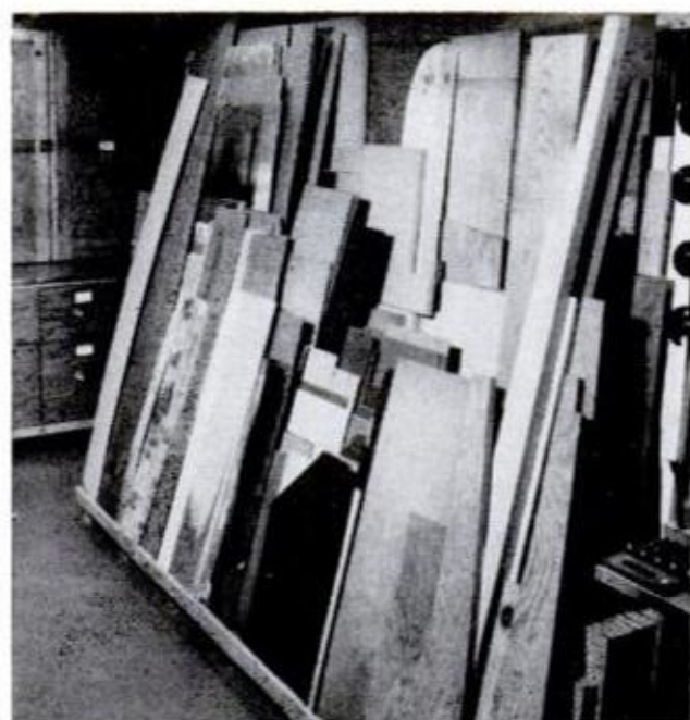
Long boards and scraps of various-thickness plywood are stored upright in simple rack.
