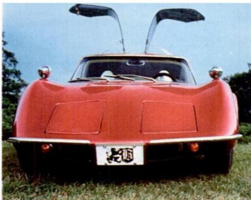
Bradley GT is an easy-to-assemble kit that's available with a full range of accessories and over 50 metal-flake and solid colors. The basic kit is $1500; the super kit version, which is more complete and requires less work, is $2400. The fiberglass body is designed for the full-length VW chassis and the detailed assembly manual starts with complete information on locating an old Beetle, a list of chassis numbers representing the various model years and instructions for removing the body from the chassis.
