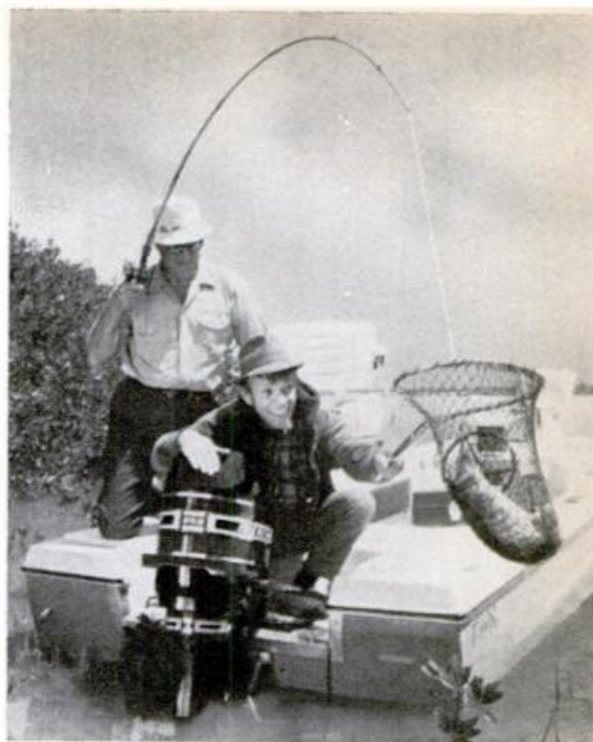
Fishermen are using faster motors to reach the hot spots where the lunkers hide. Mercury's 85-hp Merc 850 uses pulse-tuned exhaust and "power ported" pistons for added output from new 66.6-cu.-in. kicker.
