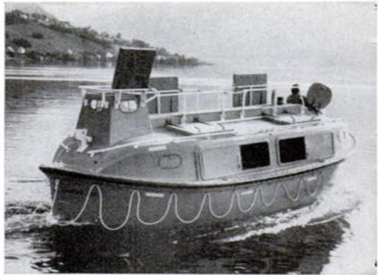
Harding survival boat , made in Norway, would provide escape for crew of disabled rig. Worker (left) inspects 26-inch bit before it's lowered to seabed.
