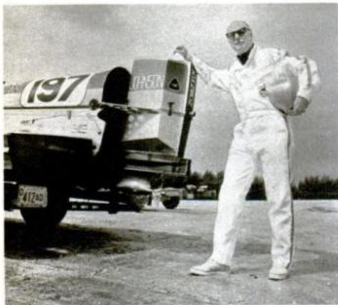
Same size as conventional two-cycle mill but hiding four rotors stacked down to waterline, unit is compact.
