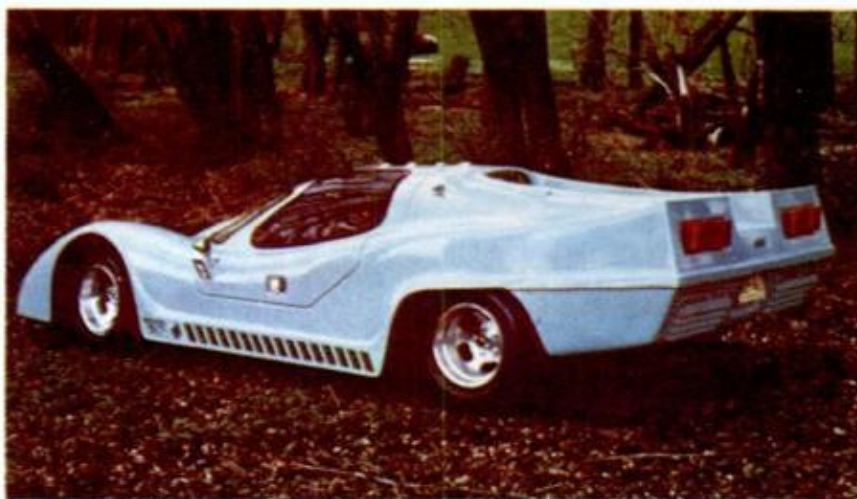
Laser 917 is Elite Enterprises body for unshortened VW chassis. Kit prices start at $1700.
