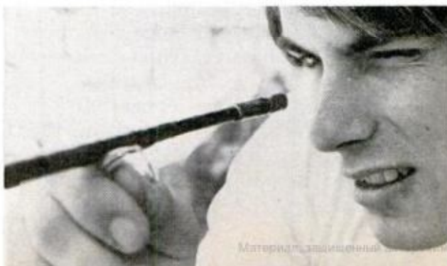
Sighting down rod while epoxy hardens allows slight bending corrections to insure straightness.
