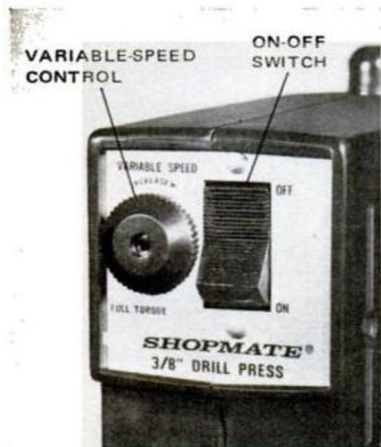
Wide range of drilling flexibility is possible with press; variable-speed range is 700 to 2000 rpm.
