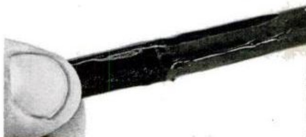
Final coat of epoxy, applied like paint to seal repair, makes joint stronger than original.
