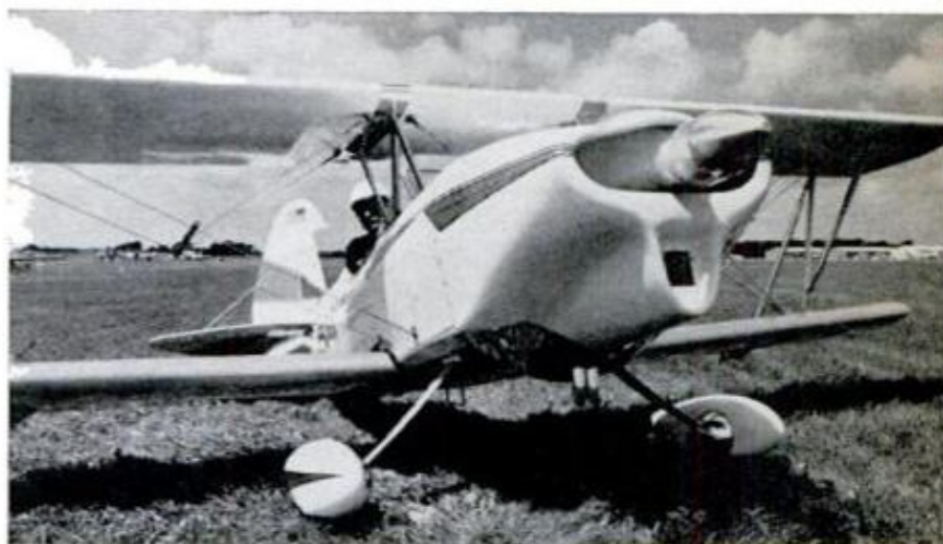
Sleek oval nose replaces blunter snout of prototype in this spruced-up modification—good example of how ship can be customized to suit builder's own tastes. Cowling is fiberglass, easier to form than canvas or aluminum. Cockpit and instruments are at upper right.
