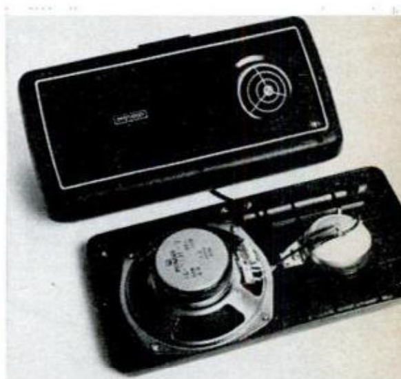
Test setup (left) used for speaker efficiency and frequency response checks included imitation "car trunk" used as speaker enclosure and a battery of instruments. Pioneer (above) had aimable tweeter, bass reflex woofer, could be mounted permanently or for easy removal.
