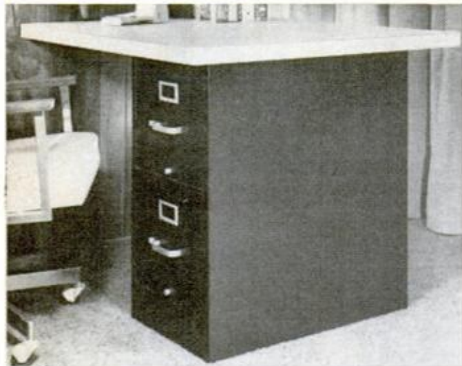
For permanent setup, desk can be supported on standard two-drawer filing cabinet in place of folding leg.
