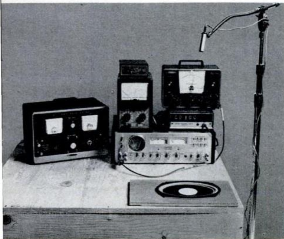
Test setup (left) used for speaker efficiency and frequency response checks included imitation "car trunk" used as speaker enclosure and a battery of instruments. Pioneer (above) had aimable tweeter, bass reflex woofer, could be mounted permanently or for easy removal.
