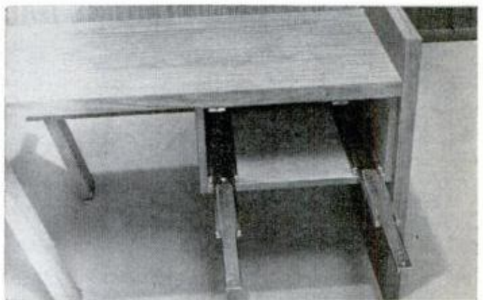
Sturdy drawer slides easily support weight of fully extended drawer. Drawer is then fastened to slides.
