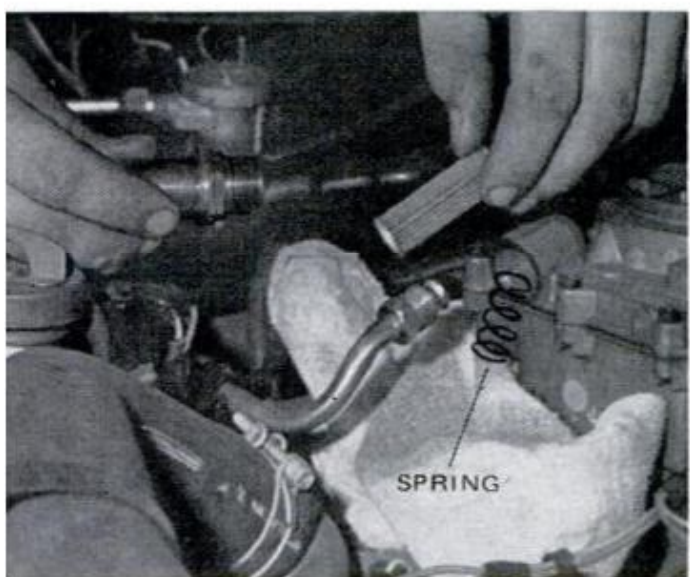
Internal-type fuel filter is found at inlet to the carburetor. When clogged, it, too, will restrict fuel flow and cause hesitation. When replacing, take care not to lose retaining spring; it can be reused.
