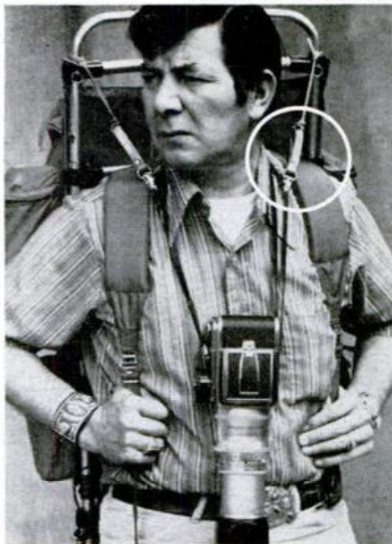
Transfer your camera's weight from your neck to your packframe when backpacking, and you can hike for days. Author did it with nylon tape and belt hooks (circle).
