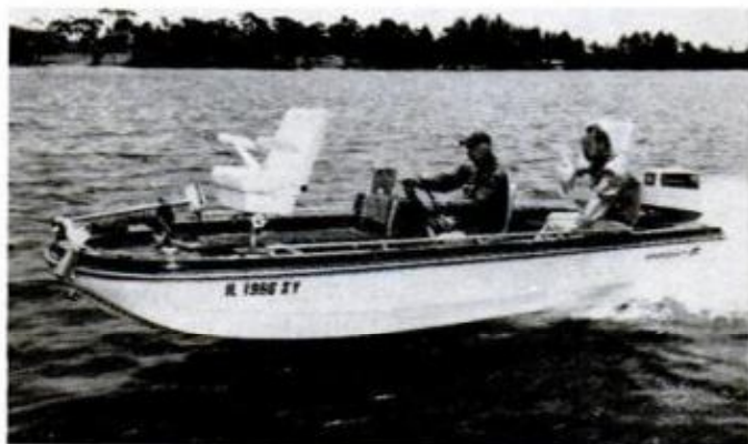
Starcraft 16 Bill Dance Pro model tops line of special models for fishing. It's rated for 70-hp motor on transom, 5.6 passengers or 1300 pounds of gear aboard.
