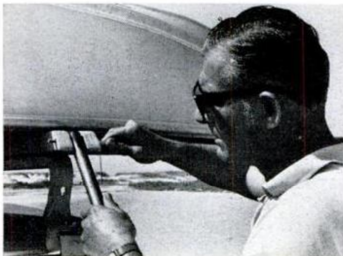
Roof rack is drilled on right side of the car to take bolt securing the pipe. Rack is rounded off at top edge.
