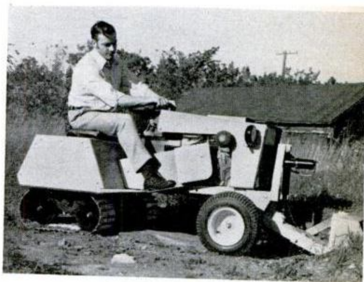
Heftier 16-hp model comes with half-track crawler-tread drive for added traction on snow or difficult terrain. It can also be fitted with a front-end loader, shown above, having 400-pound capacity.
