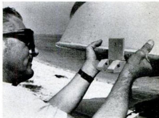
Angle irons on left side of the roof rack prevent the boat from sliding too far; help hold it for travel.
