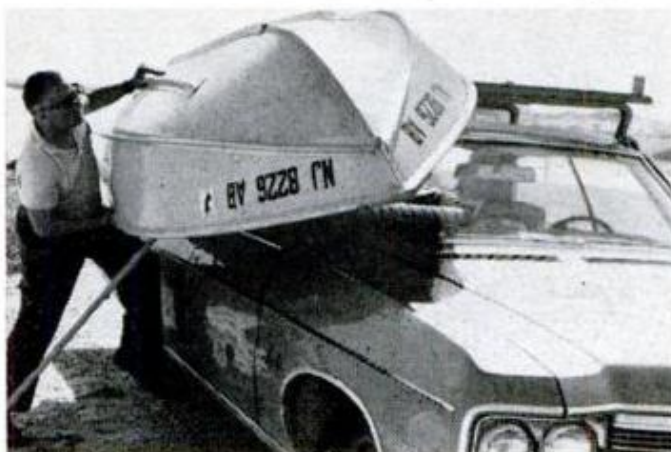
Slant of pipes clears side of the car, allowing the gunwales to ride at an easy angle up onto carrier.
