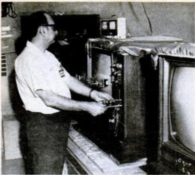
Electronic sensors (on screen) help factory technicians adjust preset controls for "pushbutton" color.
