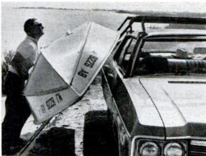
Cartopping a boat takes a lot less brawn when twin slide rod pipes are fastened to the roof brackets.
