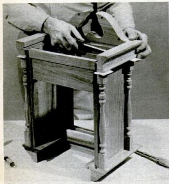
When adding crown molding , use paper spacers at tops of columns to provide clearance for gluing-on later.
