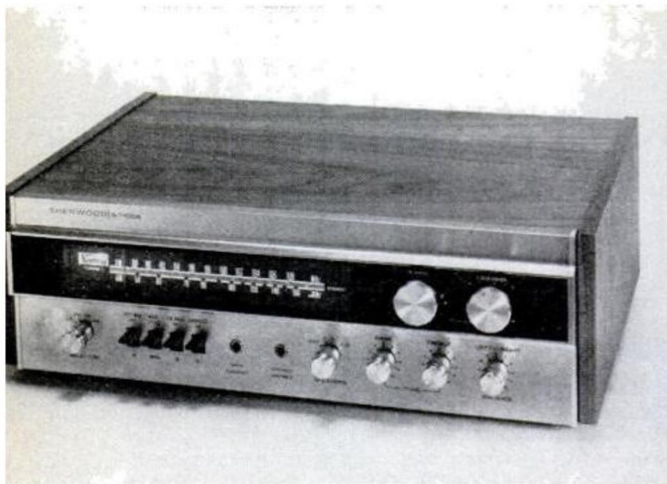
Unique tape-dubbing jack on the front panel of the Sherwood S-7100A receiver serves as tape in or tape out, according to setting of tape monitor switch. Extruded lip surrounding tuning dial and main (tuning and volume) controls is a distinctive styling accent. Four-channel jack on rear panel awaits whatever quadraphonic FM broadcasts systems may arise.
