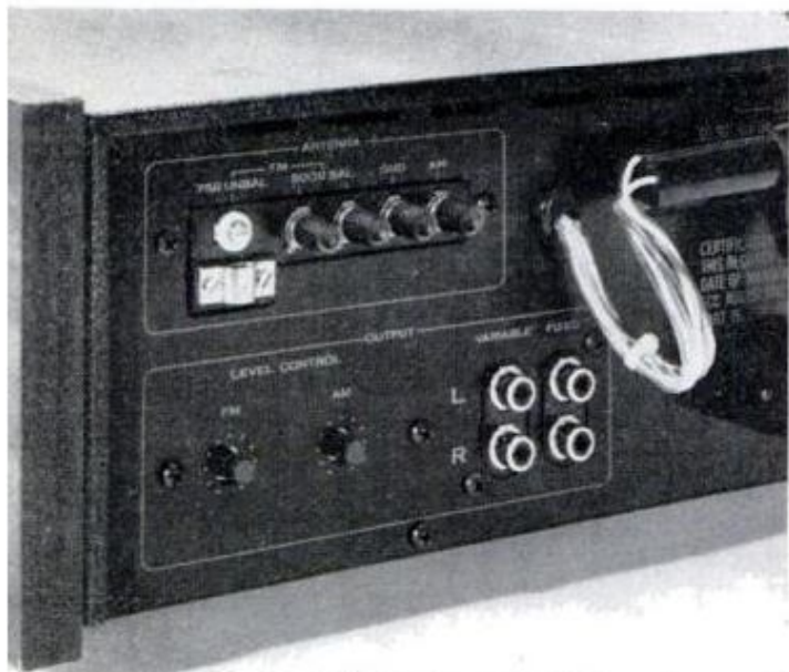
Pioneer tuner has two pairs of output jacks; one with constant level, one with adjustable output level. Clamp below 75-ohm antenna screw holds round, shielded 75-ohm cable.
