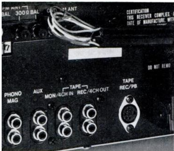
Tape monitor jacks can also be used with 4-channel adapters, so Pioneer marks its rear panel for both functions. Large multipin tape connector is for single DIN plug.
