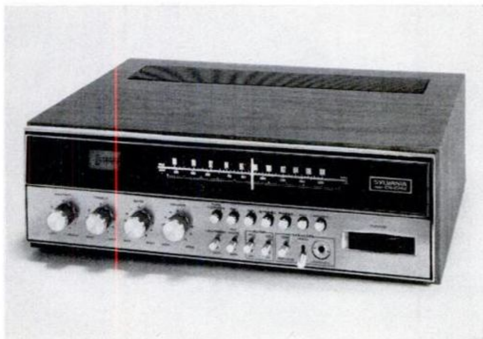
Chrome-plated knobs and levers stud the Sylvania CR27-42A's control panel; they feel just as solid as they look. Black bar at the lower right is an edgewise tuning knob, which takes some getting used to.
