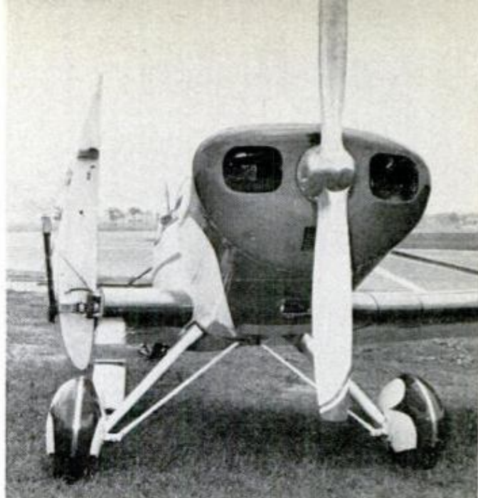
Rear-folding wings make ship easily trailerable on its own wheels. The tail wheel is fitted with a tow bar to fit standard ball-type bumper hitch on car for road-towing.
