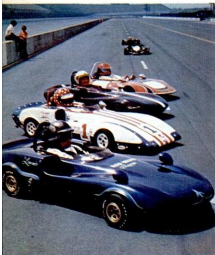
The three karts in foreground are "Moles" or limited-production models. These bodied bombs run in two classes: 6.1 and 8.25-cu.-in. engines. The fancy paint jobs and the pinstripping are de rigueur!
