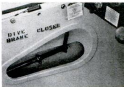
Dive-brake control is located to pilot's left. Students are taught to test the control before getting into landing pattern. A "frozen" control is not unknown.
