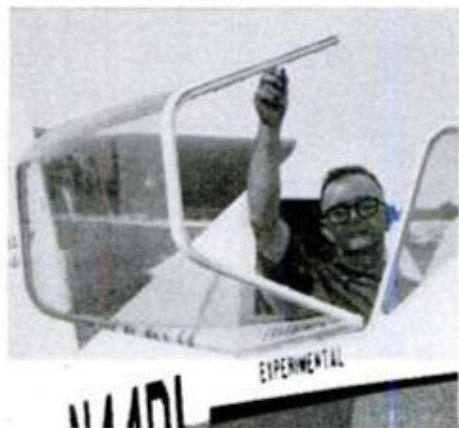
Side-hinged canopy swings up for access to cockpit, is fully removable.
