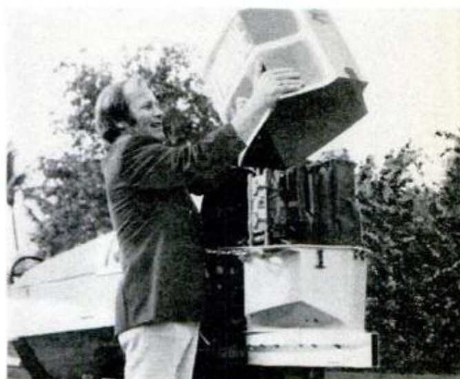
Taking the wraps off, ace unlimited driver Bill Muncey shows top half of Evinrude's new rotary high-performance mill. Johnson is testing a similar engine.
