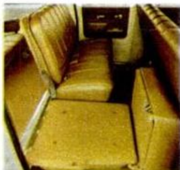
New folding second seat standard on Series 20; available, Series 10. Cushion folds forward. Backrest folds down.
