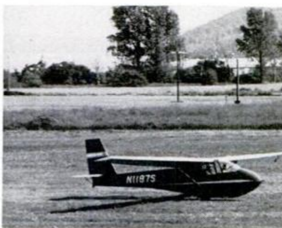
Extended, the dive brake allows plane to lose altitude without causing it to pick up speed. Dive brakes make landing easier, but plane can land without them.
