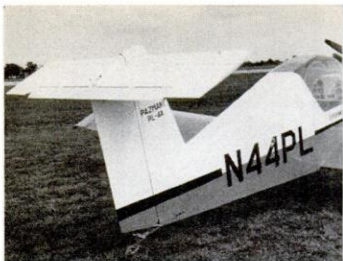
Top-mounted horizontal stabilizer, forming T-tail arrangement, is easier to construct than conventional tail, also gives good stability and control in flight.
