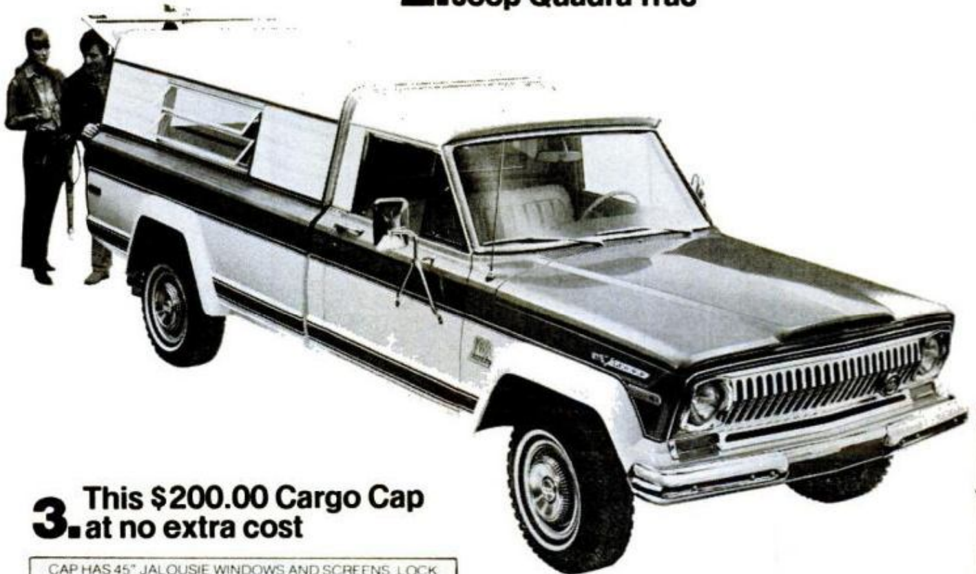
CAP HAS 45" JALOUSIE WINDOWS AND SCREENS. LOCKABLE LIFTGATE WITH SAFETY GLASS
