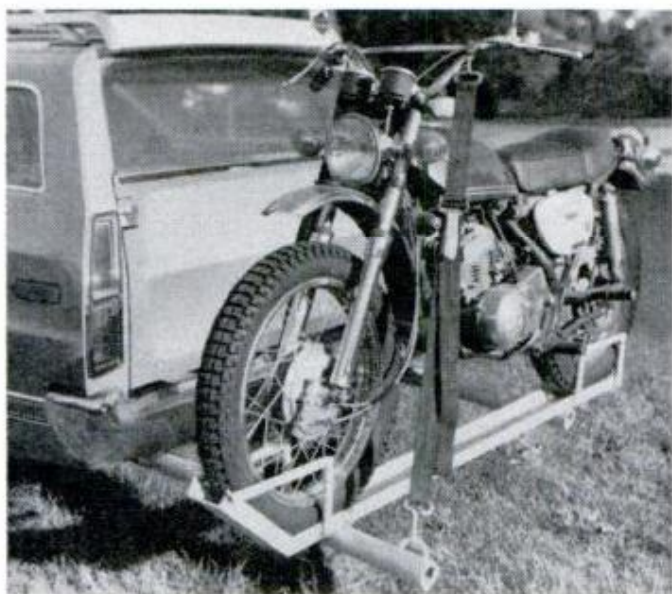
Carrier holds 315-lb. trail bike—too heavy for bumper-mounted types—slides into mounts welded or bolted to underframe of car, leaves bumper unmarred.
