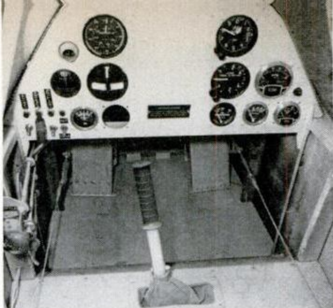
Cockpit is roomy, clean, uncomplicated. Only barest number of most necessary flight instruments are used in order to keep cost and complexity to a minimum.
