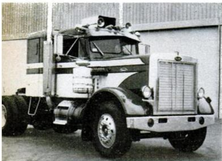
ANOTHER POPULAR MAKE is the Peterbilt. Model shown has tandem rear axles, sleeper box, enough bright metal to satisfy the most finicky of drivers
