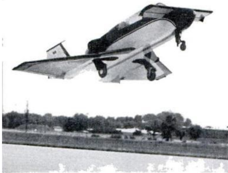
BELIEVE IT OR NOT , this is a takeoff, not a landing approach—showing how steeply the VariViggen gets off the ground, using canards for added lift
