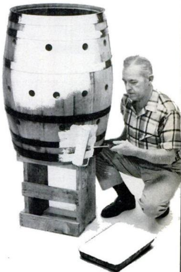
OLD BARREL CAN BE PAINTED , new one stained and varnished. Treat the inside with wood preservative
