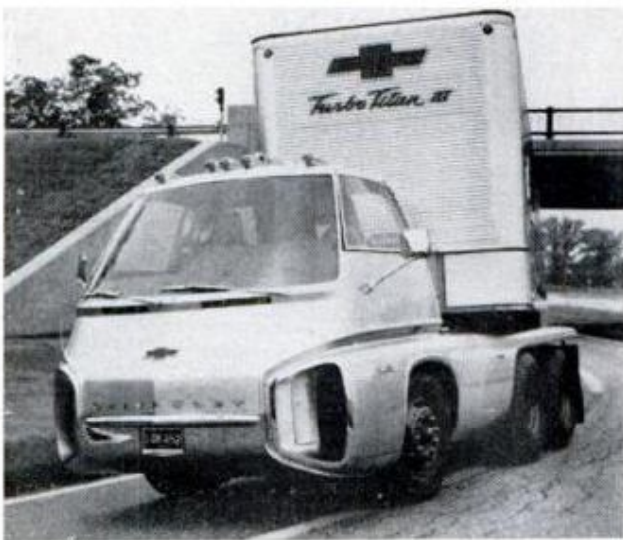
CHEVROLET'S CONCEPT of gas-turbine transport of future is fiberglass and a steel Turbo Titan III. The experimental design even includes "astronaut" seats
