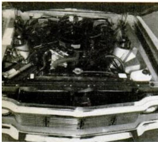
THE 304 V8 ENGINE is most popular with owners. Smog controls make engine hard to tune, say many
