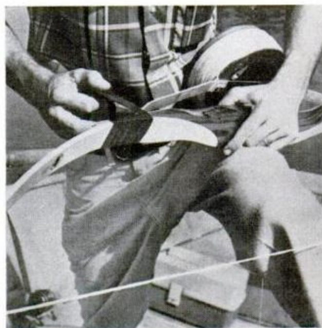
PLASTIC ELECTRICAL TAPE secures reel brackets to bow. Tape should be removed after use, or left on no more than a week, to prevent possibility of sticky black adhesive from tape remaining on bow
