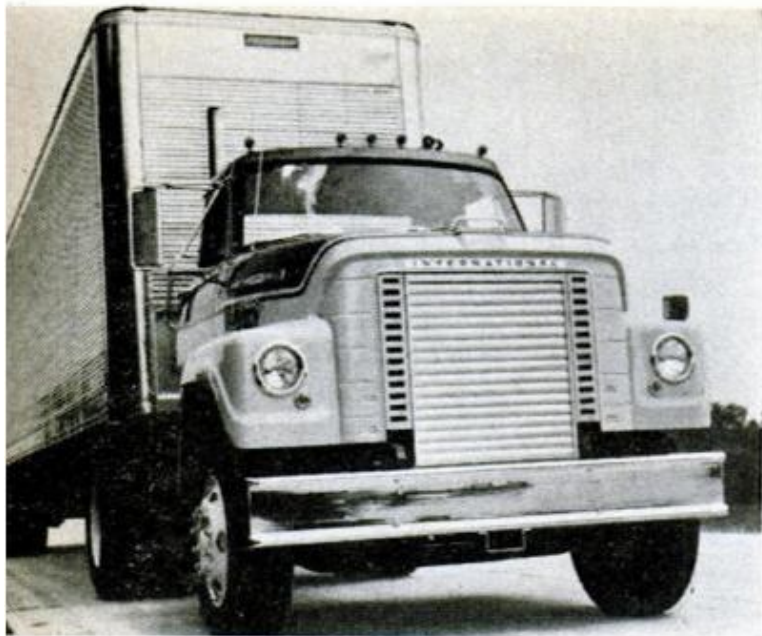
NEW LINE from International is the Transtar series of tractors. Single and tandem-axle versions are available. The standard engine is a 230-hp diesel
