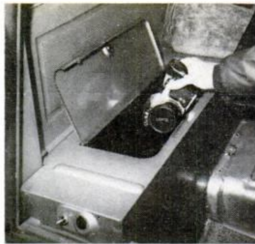
SPARE COVER UNSNAPS , bins are lockable. Safety switch keeps tailgate locked with the engine running
