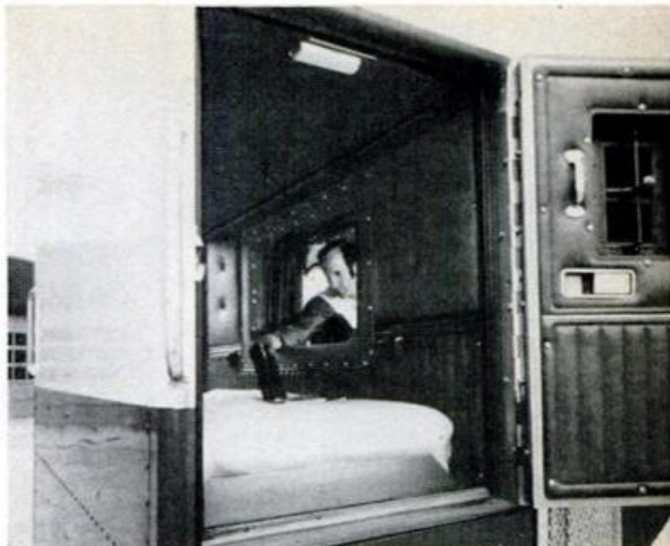
TYPICAL SLEEPER is wall-to-wall mattress and it may be airconditioned. Padded full door, for easy access, is optional and adds to cost of "bedroom"
