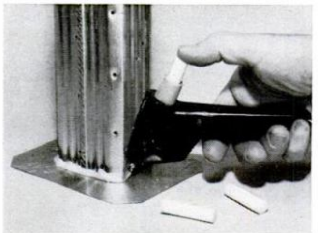
STANDPIPE IS CLOSED at bottom with an aluminum scrap "welded" to pipe with an electric glue gun
