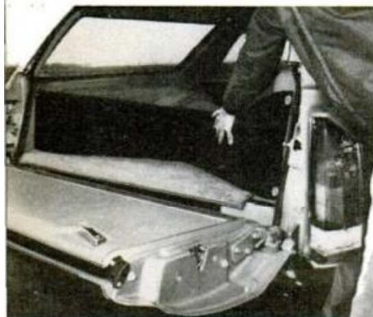
CARGO NET , part of visibility group, prevents grocery bundles from falling forward in sudden stops
