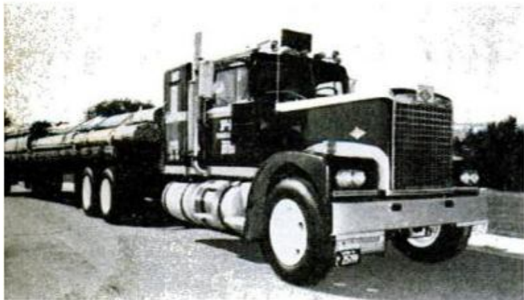
BIG DIAMOND REO hauls a heavy load on a flatbed trailer. Rigs used for heavy work in mountain areas usually are ordered with an axle ratio of 6.14 to 1
