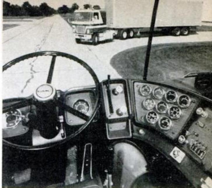
CURVED INSTRUMENT PANEL surrounds the driver of a GMC Astro tractor. Speedometer and tachometer are seen through wheel. Other gauges are clustered
