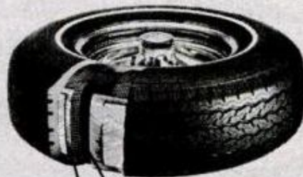
Two Steel belts Radial design
