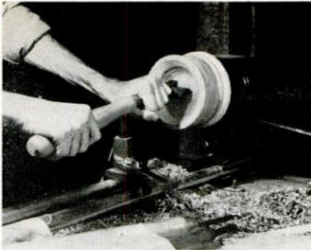
3. INNER CUT to hollow out reel is stopped once backup paper and pine block with screws are reached
