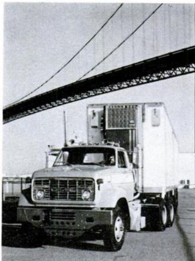
LIKE OTHER MAKERS , GMC builds tractors of conventional and cabover design. The legal length requirements are easier to meet when cab rides over engine
