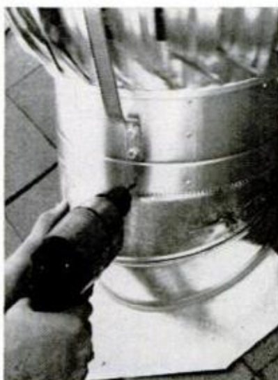
10. USE BASE-RING HOLES as guide in drilling matching holes around and through base flange
