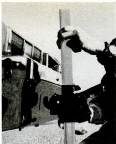
SLOTTED BUMPER accepts the jack at its strongest point and makes the lifting steadier
