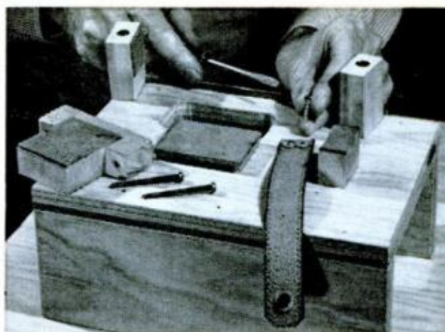
ASSEMBLING HOLD-DOWN DEVICES on sander platform (above). Below, platform with blocks and strap in place. Note opening provided for airflow from motor
