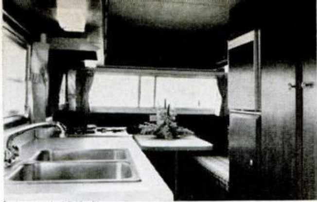
DINETTE at back of trailer becomes 4x6-ft. double bed. Sink is of stainless steel. On opposite wall is 4-cu.-ft. gas/electric refrigerator
