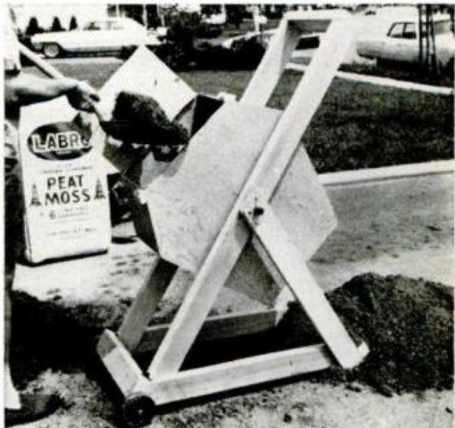
WHAT TUMBLER DOES FOR THE SOIL. Clayey soil below was much improved by quick treatment in tumbler. Hand-held finished product has sand and peat added, but the soil could need other ingredients as well
