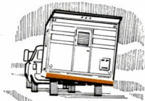
LEAN to side, tongue-heaviness or back droop can indicate bad springs, loading
