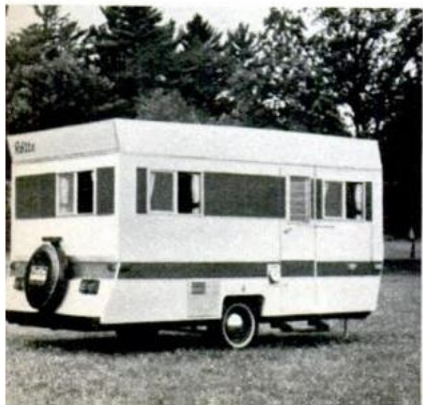
FOLDING TRAVEL TRAILER that hinges down its four Retractable-Walls to camper-trailer height, Rolite 1700 Self-Contained has power-lift top, toilet, shower
