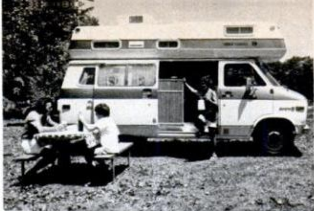
SUPERIOR has widened its van motor home by 14 inches without changing basic Dodge or Chevy chassis
