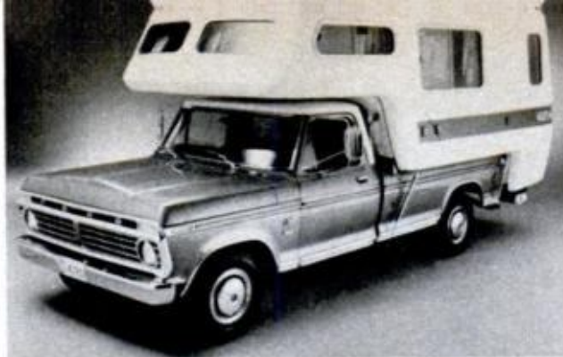
FORD AMERICAN ROAD is name of new luxury pickup camper you haven't seen before. Built by Starcraft for marketing through Ford dealerships, this slick 11½-footer made of 1-piece fiberglass claims full self-containment, two holding tanks plus design innovations
