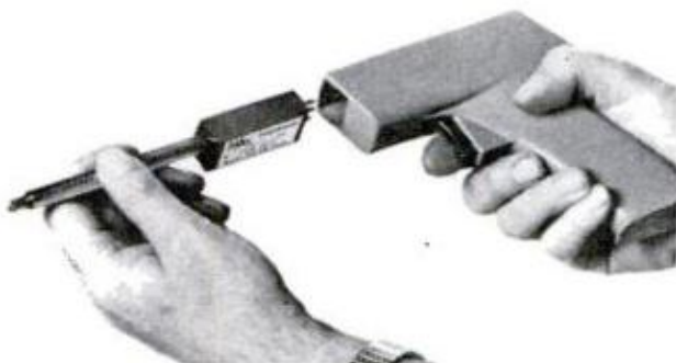
CHANGING POWERHEADS on Weller Tempmatic gun changes tip size and temperature, but not wattage. 150-watt tip shown has screwdriver point, automatically regulated 700° tip temperature; 150-watt conical head has 600° temperature. Head costs $10.25
