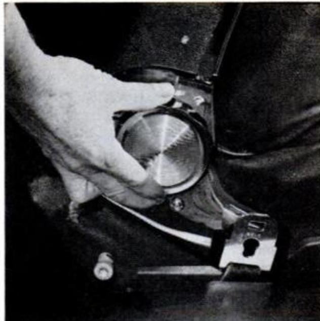
SEATBACKS ADJUST not only for rake, but also have back supports inside that can be dialed firm, soft
