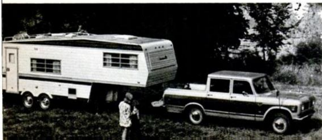
QUINSTAR 24-foot model is new addition to line of Coachmen 26 and 28 models. All three fifth-wheelers are mounted on wide-track tandem axles with four-wheel electric brakes. A three-way gas/electric refrigerator, 33-gal. holding tank and 12-volt converter system are standard
