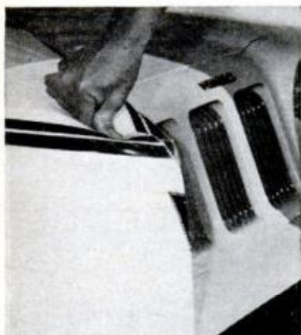
BOPPABLE NOSE pops back, but vinyl racing stripe cracks if wrinkled too often. Louvered side windows don't go down, are hard to clean. Driver can see out of them but rear riders can't
