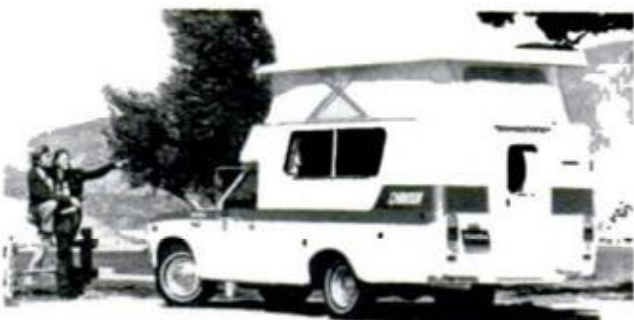
RIDING HIGH , the driver of Shasta's new Motorhome looks out over traffic. Features include aluminum skin and frame, steel roll bars and rubber body mounts
