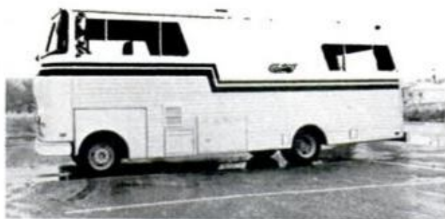
RIDING HIGH , the driver of Shasta's new Motorhome looks out over traffic. Features include aluminum skin and frame, steel roll bars and rubber body mounts
