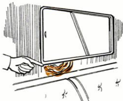
LEAK MARKS around the windows? Sealant should fix this, but check for wall damage
