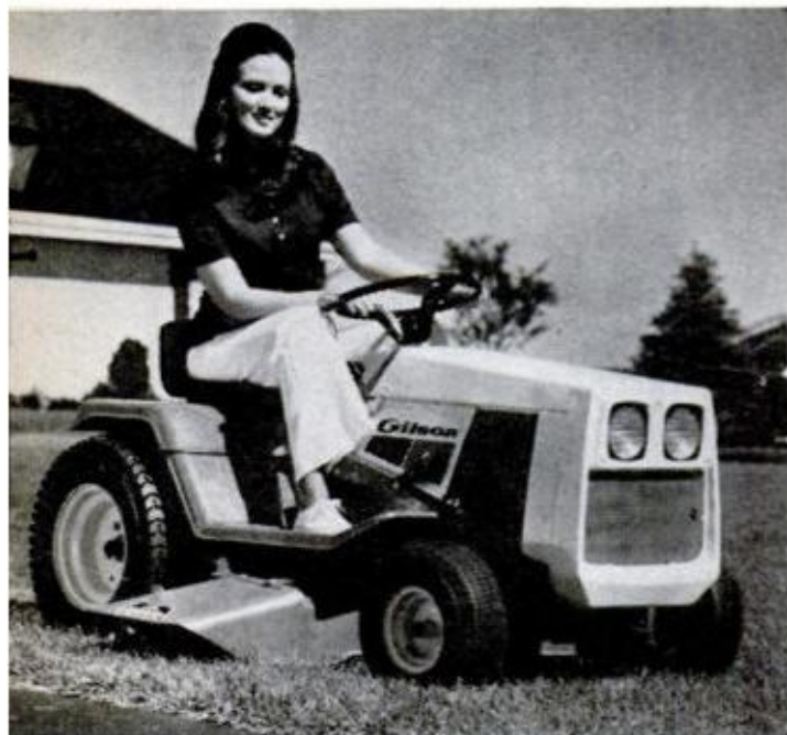
GILSON 8-HP TRACTOR has low profile and 36-inch, twin-bladed mower. Traction-drive system is said to deliver smooth power in all speeds
