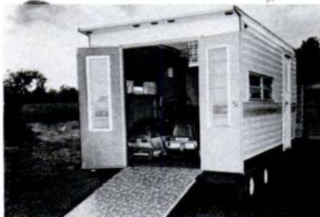
DOUBLE-DUTY TRAILERS , like All Sports Vehicle from Ace Traveler, Alfred, Me., has four swing-up bunks to allow rear loading of snowmobile or motorcycles
