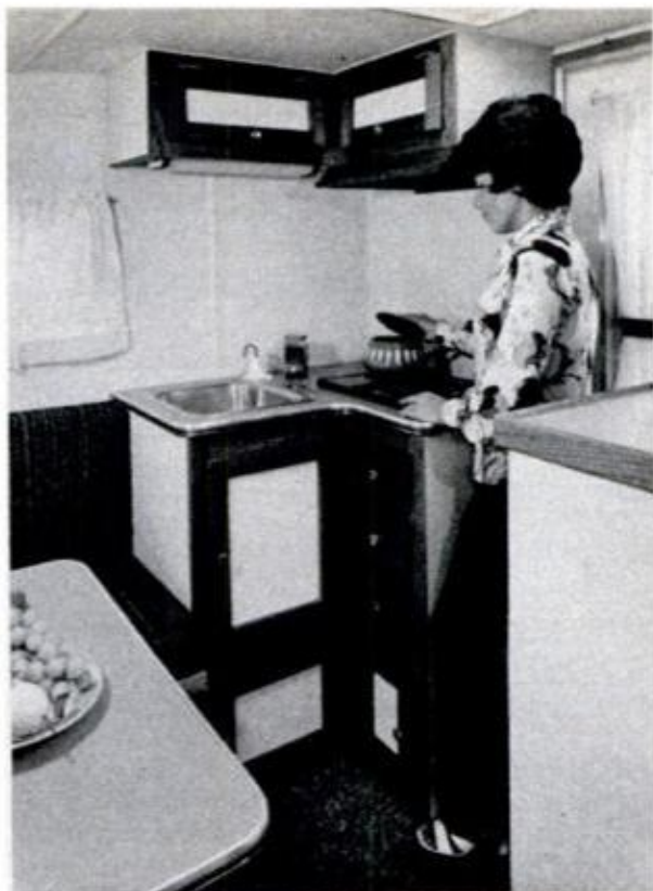
TINY KITCHEN AREA contains two-burner range, sink and self-contained water supply. An icebox is installed on the opposite side of the camper
