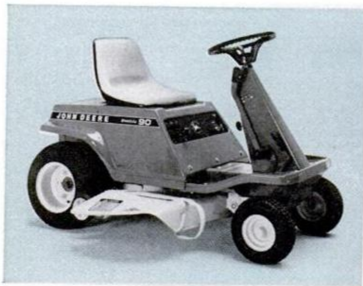
THREE 12-VOLT BATTERIES supply power for John Deere's Electric 90. It has 34-inch mower, can cut about an acre of lawn on a charge, and costs $885
