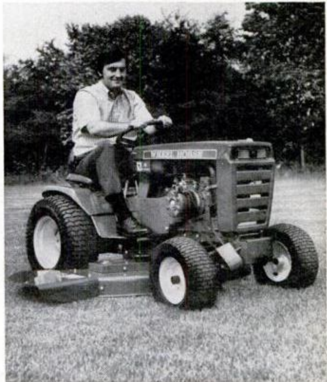
WHEEL HORSE couples a 48-inch mower to 16-hp engine in its big Automatic garden tractor (right). Attachments include hefty sweepers, snowblowers
