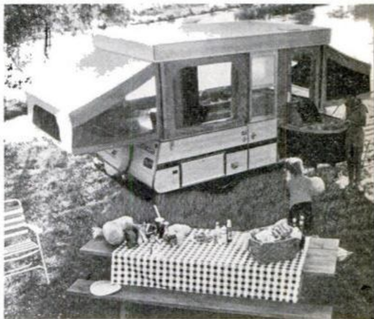
SWING-OUT KITCHEN for serving inside or out with top up or down is feature of Starcraft Swinger 6
