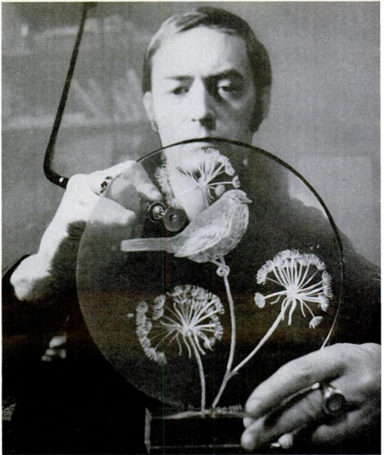
ARTIST CHARLES LE NORREYS uses diamond-impregnated grinding wheel to shape leaves and stems
