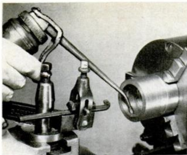
FLOOD THE WORK with a sulfurized cutting oil when you bore the spindle-nose recess in the chuck body
