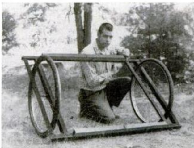
KEEL NOTCHES in cross members help center the hull FEBRUARY 1973
