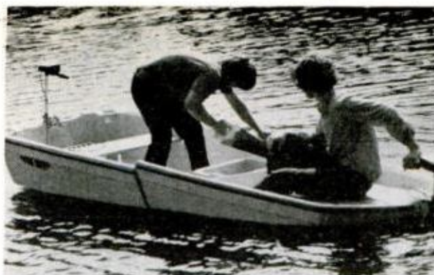
CENTER STORAGE COMPARTMENTS also divide hull with water barriers, and can serve as fish-bait wells
