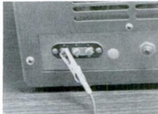
ALLIGATOR CLIP is a good temporary connection to set. Plain wire or spade lug is more permanent
