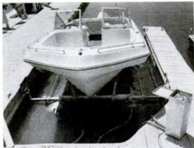
LIFTED CLEAR OF WATER , fouling and ice, the hull is stable enough for passengers to climb aboard
