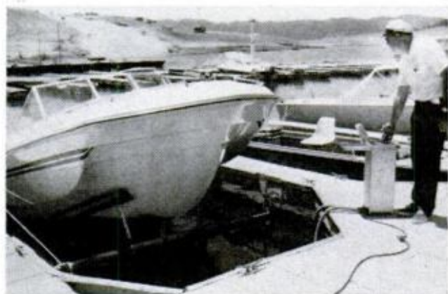
AIR DISPLACES WATER in twin fiberglass tanks and boat bow rises first on padded cradle of the hoist
