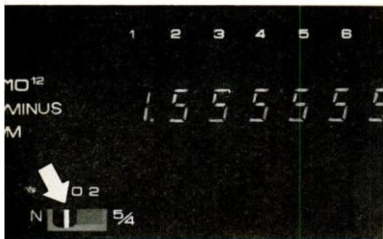
DECIMAL SWITCH (arrow) on Miida can be set for fixed or floating decimals. Floating-decimal answer (left) shows all decimal places that will fit
