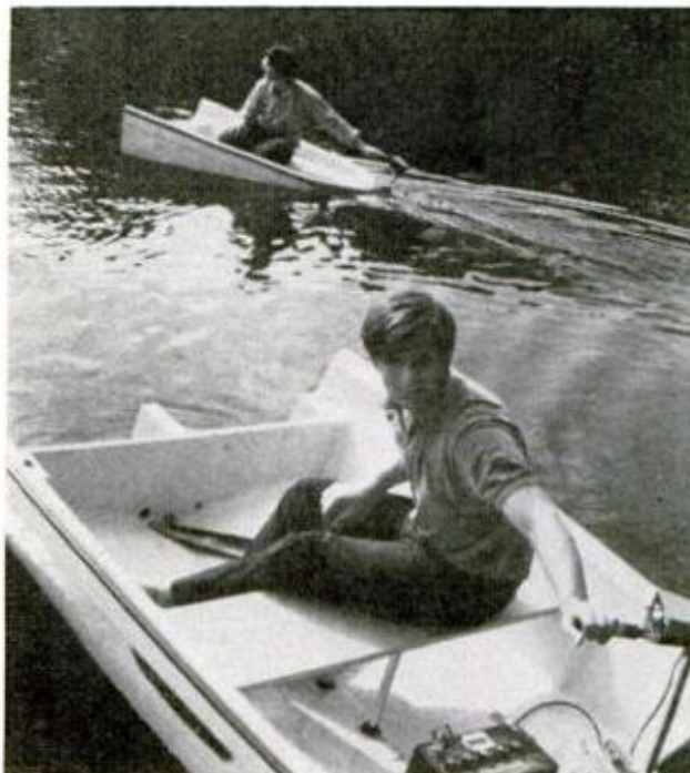
MOTOR MOUNTS are molded into bow (background) and stern. Plugs allow draining center compartments
