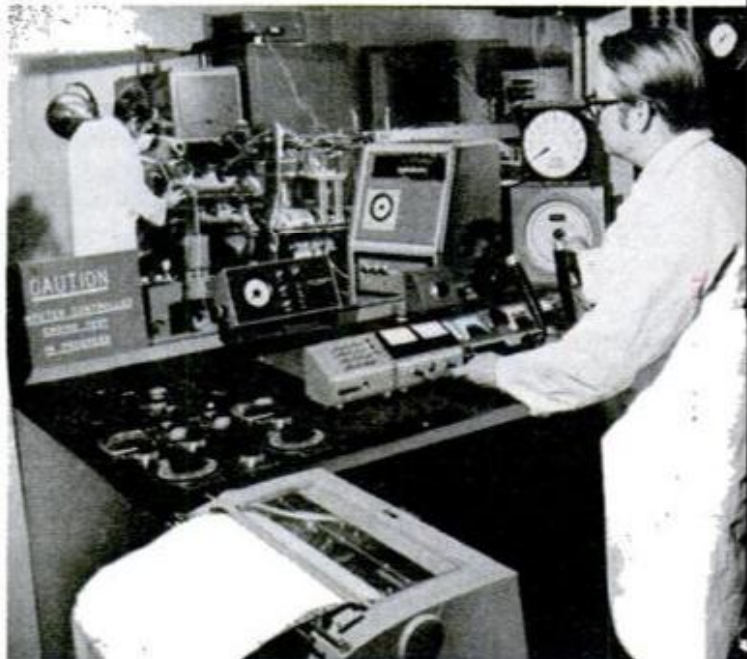
TEST CELL at GM Research Laboratory "road tests" engine, computer-duplicating actual road conditions
