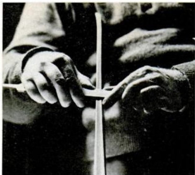
SHARPEN SIDE EDGE with flat No. 10, removing rough spots, nicks. Result should be even edge that forms 90° angle between bottom edging surface and side
