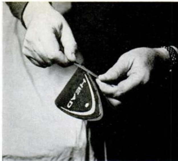
TIP EDGING of ski should not be sharp. Starting even with front end of center groove, round edging forward toward "shovel" tip to prevent tip-tripping
