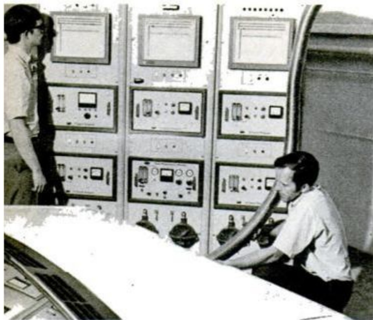
EMISSIONS MEASUREMENTS at Bendix laboratories are for unburned hydrocarbons, carbon monoxide, NO x
