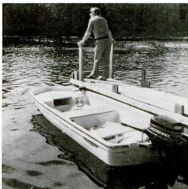
STORAGE BOXES in bow and under center seat have seat tops secured with shock cord to prevent loss
