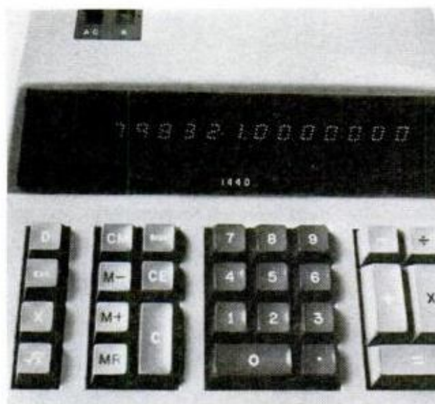
EXTRA FUNCTIONS on MITS 1440 include square root, square, memory (with + and - inputs, independent clearing). EXC key exchanges dividend and divisor for some complex calculations. D key sets decimal
