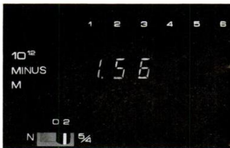
on the display, cuts off others. Fixed decimal settings demonstrate round-off: two-place setting (center), useful for dollars and cents, rounds 1.555
