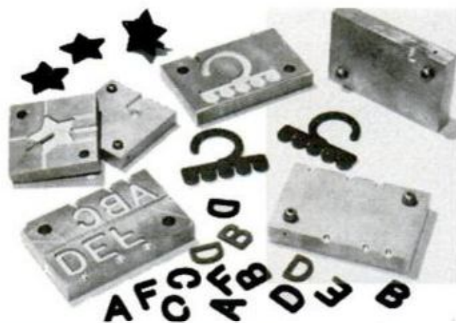
SAMPLING OF MOLDS AVAILABLE show few of many plastic items you can mold and sell: star tree ornaments, sign and nameplate letters and novel hosiery hangers
