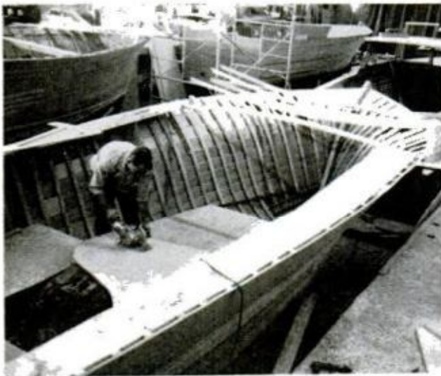
PREPARATIONS for framing out may require space of a rented warehouse. Figure you'll start job upside down, then right the planked hull for final decking
