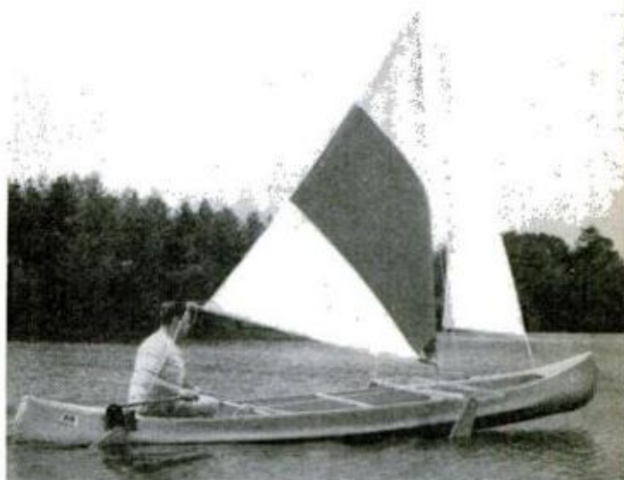
CONVERSION TO SAIL for any rowboat or canoe is claimed for Michi-Craft's $245 kit, with sail, spars, leeboards, rudder, motor-mount bracket
