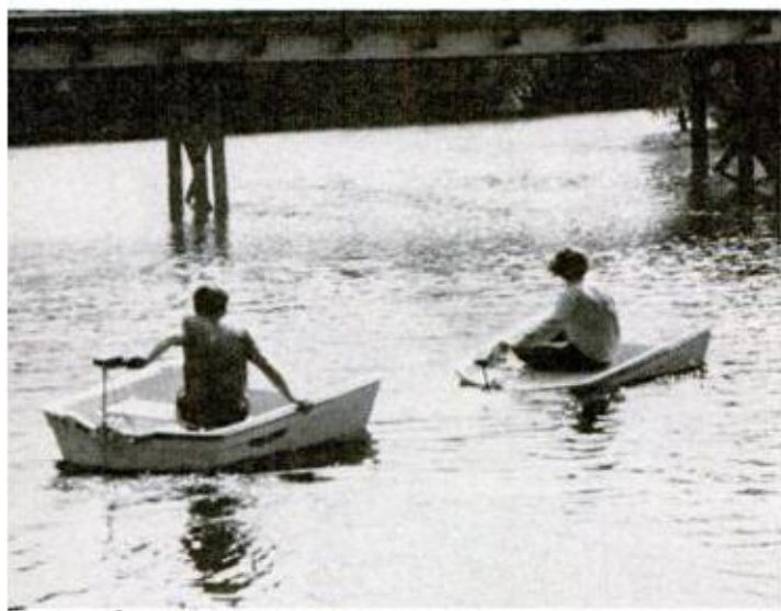
TWO FOR THE PRICE OF ONE , but with limited free-board, is result of cut-up test of hull's flotation FEBRUARY 1973
