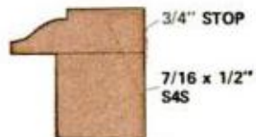
6 1/2 x 9 1/2 in. (7). Assemble the subframe and add stop molding at front. Size all wood with shellac and allow to dry. Sand it lightly and brush on avocado green latex paint. Let dry, finish with varnish. Print should be backed with cardboard and, if desired, covered with glass
