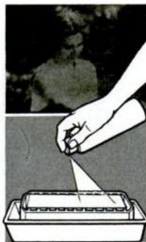
POSITIVE IMAGE is created by reversal exposure, brought out by color-developer spray. Combination of positive and negative images turns print black
