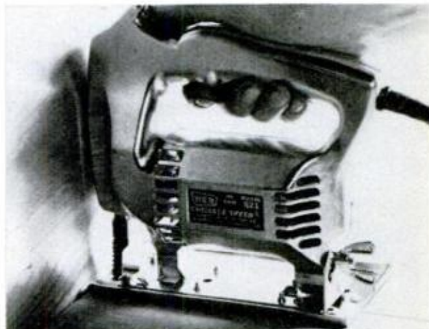
SHOES ON SOME SAWS SLIDE BACK to permit cutting to a wall when sawing openings for ductwork
