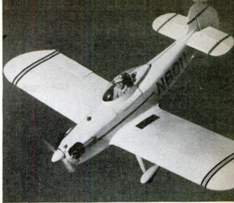
CESSNA SPRING GEAR and hydraulic brakes are among modifications made by Jim Kerley. His 25-hp engine eats only two gallons of fuel per hour. Range is 270 miles
