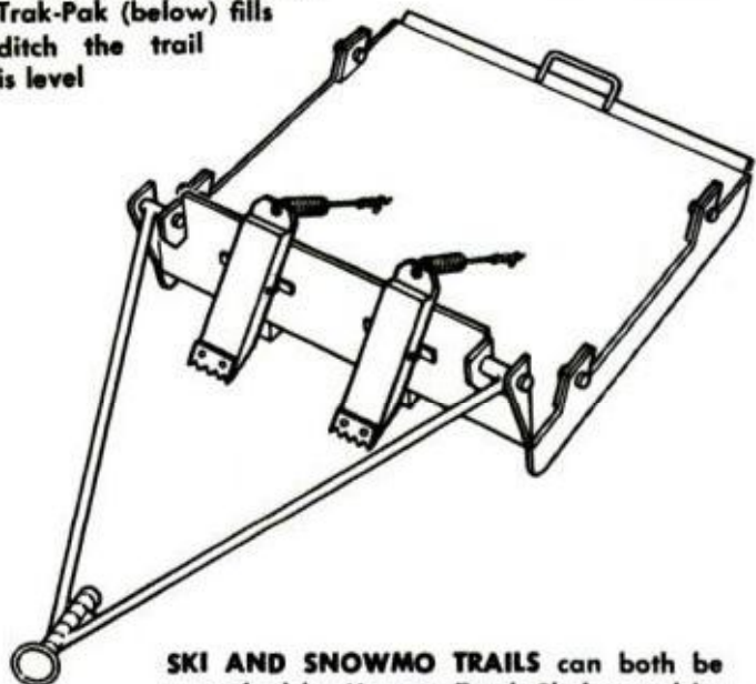
COMPACTOR bar can pack snow or scarify it to break hard-packed moguls, rough stretches
