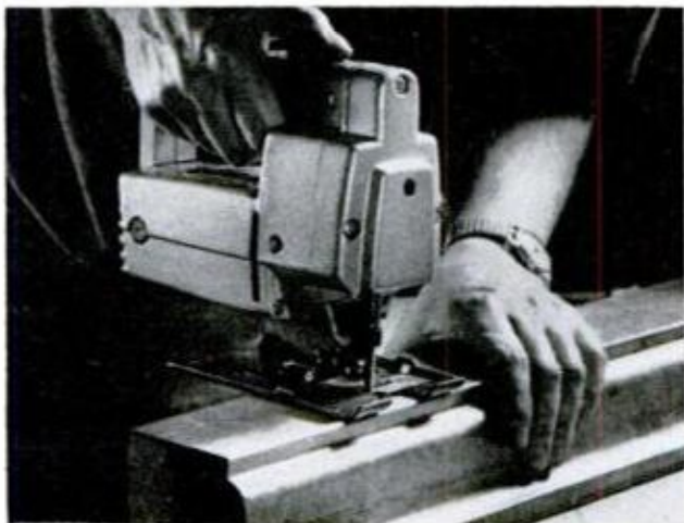
TO SAW SHEET METAL SMOOTHLY , use a 32-tooth, wave-set, metal-cutting blade with a slow, even feed
