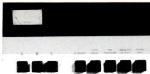
HEATH CONTROLS include tuning modes, three station preselectors. Meter reads signal or multipath
