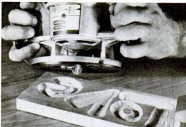
A REAL CHALLENGE for a creative craftsman, free-hand routing is done without guides or templates
