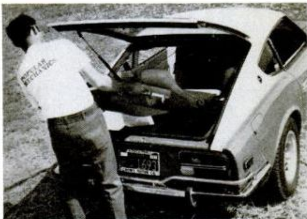
CARGO DECK is fine for pets but not people. Tiedowns are designed to keep bags from sliding forward
