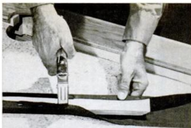
CUSHIONS ARE COVERED with 5-in.-wide strips of billiard cloth, pulled taut and stapled to rear side
