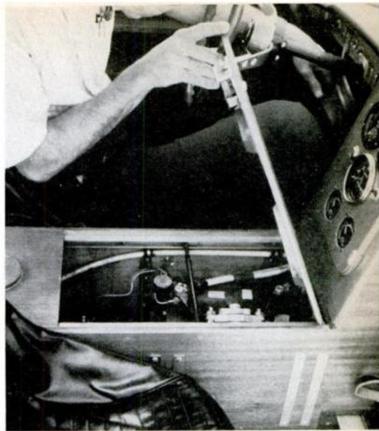
CONSOLE BETWEEN BUCKET SEATS is actually motor housing with a hatch for access. The 15-hp motor is coupled to rear wheels without transmission. Instruments are mounted in beautiful mahogany panel
