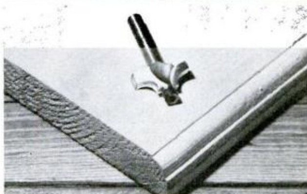
TYPICAL EDGES SHAPED using a pilot-type bit: rounded-over (quarter round) at top and beading
