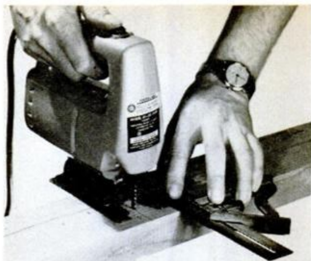
FOR PERFECTLY SQUARE CUTS when sawing lumber to length, use small try square to guide saw's shoe
