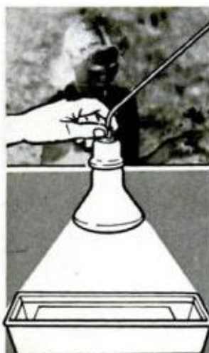
POSITIVE IMAGE is created by reversal exposure, brought out by color-developer spray. Combination of positive and negative images turns print black
