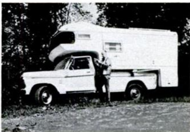
FORD SUPER CAMPER SPECIAL F-350 has longer wheel base, higher GVW rating, new tie-downs, sway bars
