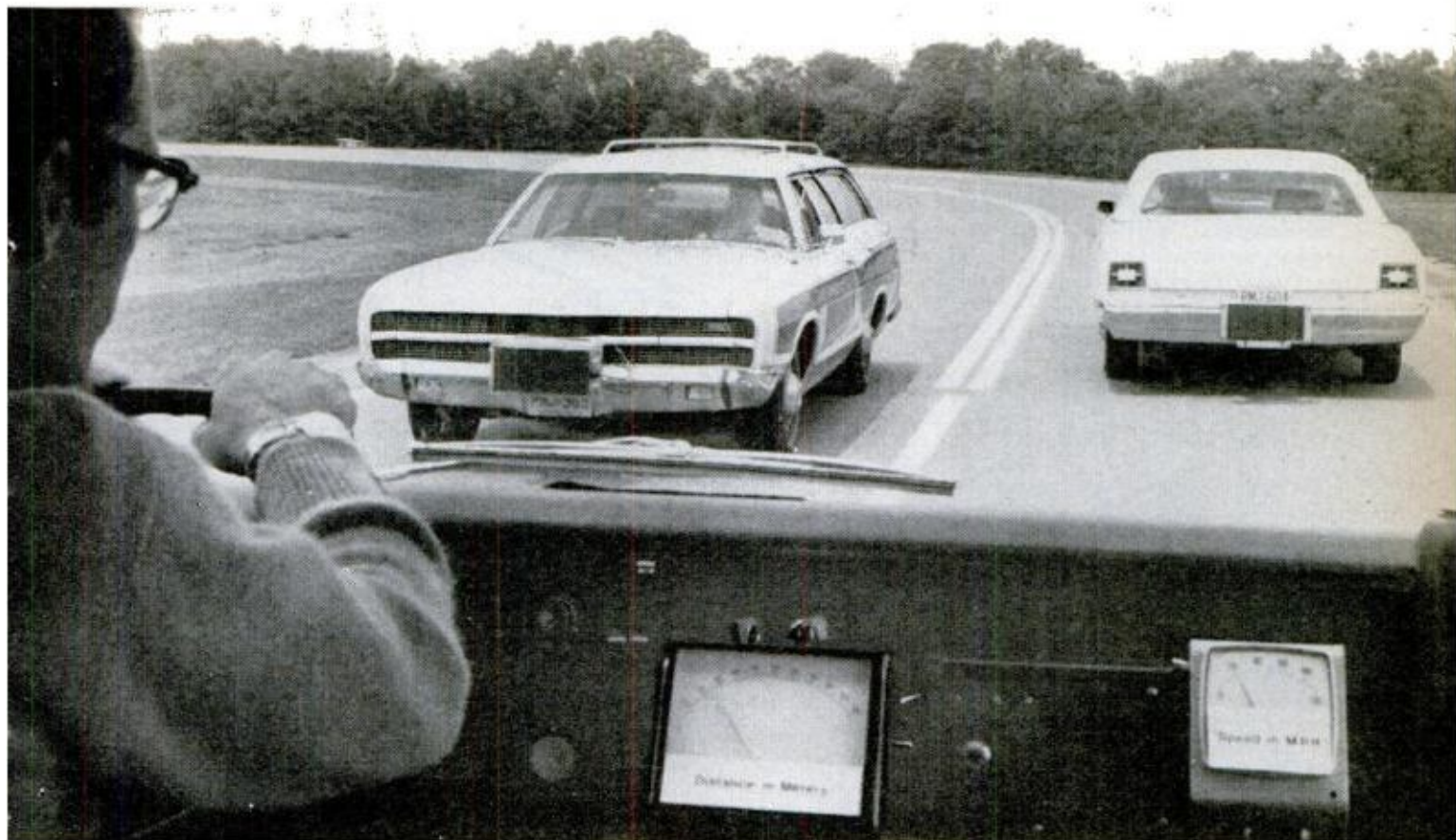
SPEED AND DISTANCE are shown on meters in RCA's experimental system. Reflector under plate of car ahead sends back radar signal at double frequency
