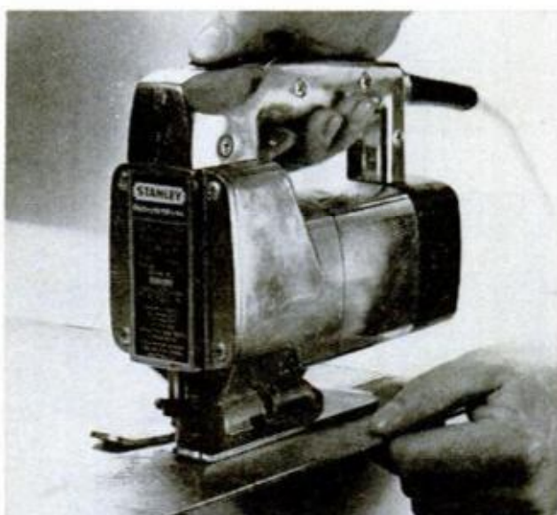
ON ALUMINUM , use a blade with teeth fine enough not to snag, but coarse enough to avoid any loading
