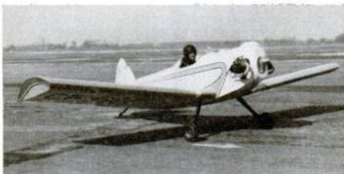
LANDING GEAR MOUNTED on fuselage wing stubs and blunted wingtips were major modifications made by Canadian Geoffrey Broadwood. Plane cost $1000 to build
