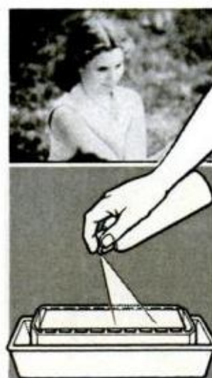
BLEACH removes negative image, brings out pale, bluish color. The final stabilizer spray deepens color, but it's still blue until it's washed and dried
