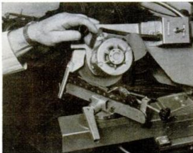
GRINDER WHEEL on saw chain grinder is set with angle to assure definite hook when the chain is ground
