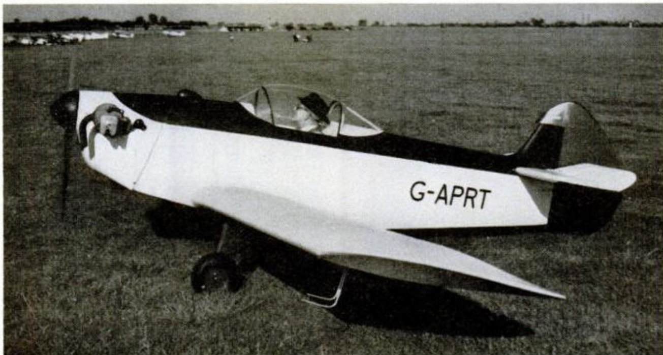
THE PLANE THAT STARTED IT ALL —the original Monoplane —is shown with John Taylor at the controls. It has a wooden frame that's covered with plywood, a fixed main landing gear and a modified VW engine
