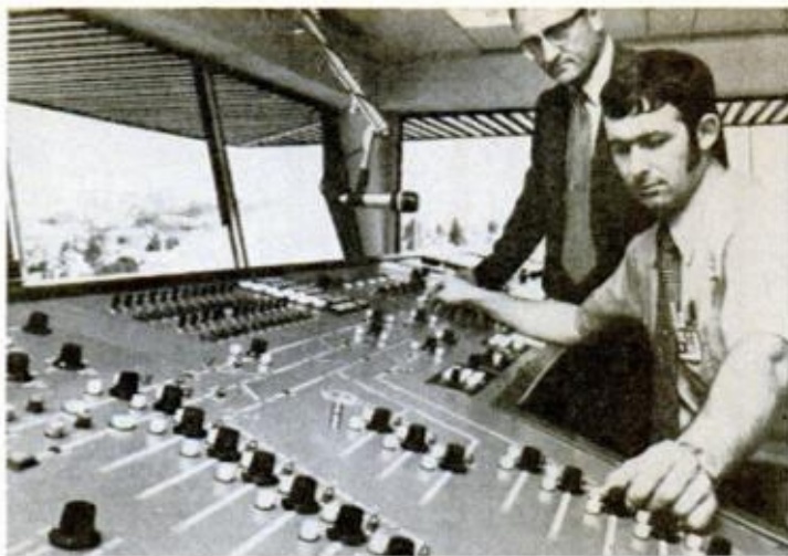
ALL SWITCHING , inventory and communications functions are directed by this computer in BART's big repair yard
