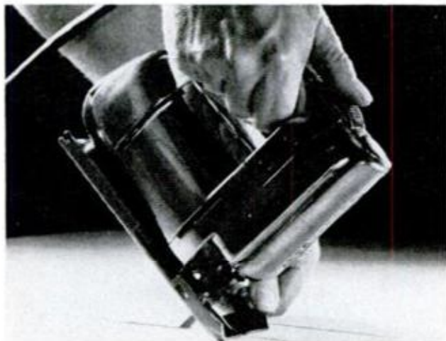
FOR A PLUNGE CUT , rock saw forward, then gradually pivot tool backward until blade cuts through
