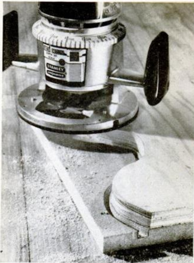
TEMPLATE CUTTING is done using template guide and pattern cut slightly under the finish-work size
