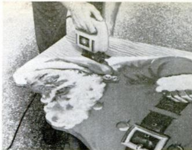
USE SABRE SAW and fine blade to saw out Santa. Let saw glide over the work so as not to mar poster
