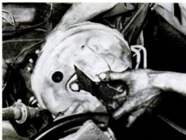
VACUUM BOOSTER with master cylinder integral is installed next. Connect all brake lines carefully
