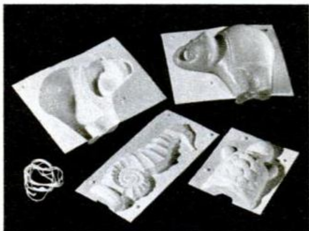
TWO-PIECE PLASTIC MOLDS consist of matching halves bound and sealed at edges with masking tape
