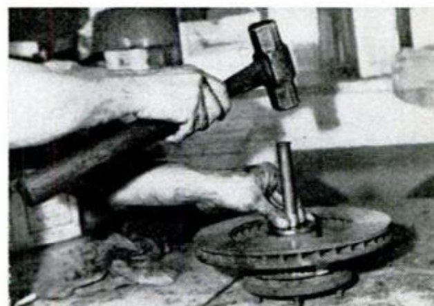
DISC ROTORS are then turned to clean them and check trueness. Here, new bearing seals are being installed. Rotor can then be installed on spindle as shown in the photograph on the opposite page
