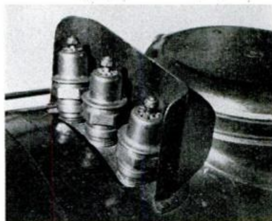
THREE SAFETY VALVES bleed off steam when the pressure in the boiler tops 140 pounds
