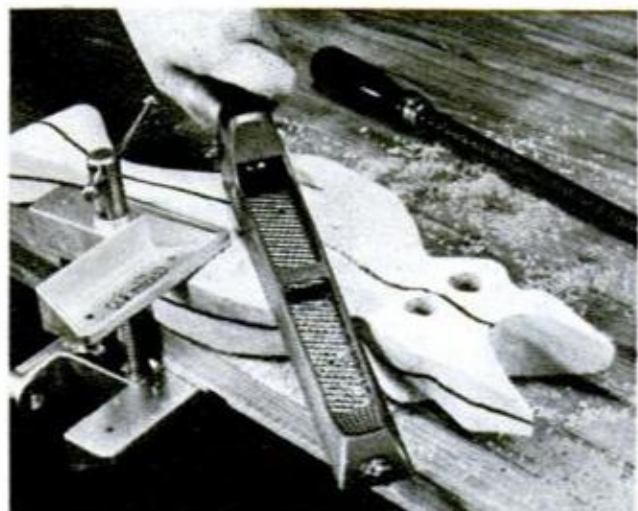
5. MIDLINES are drawn down center of front, back and both sides. Using these for reference, contour the body with a flat blade in either file or plane
