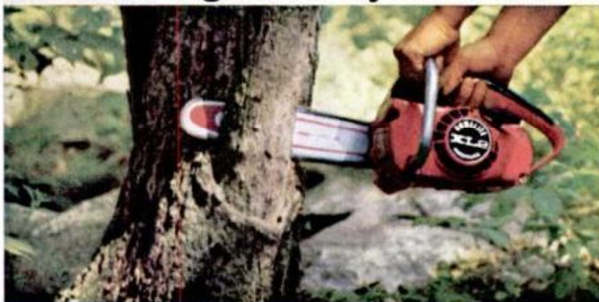
1 Front trigger gives more control on tricky angles.
