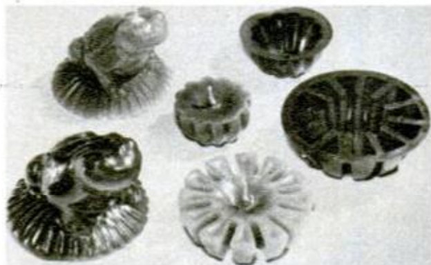
ONE-PIECE STRETCH MOLDS are flexible. To remove from candle, you pull them off like a rubber glove
