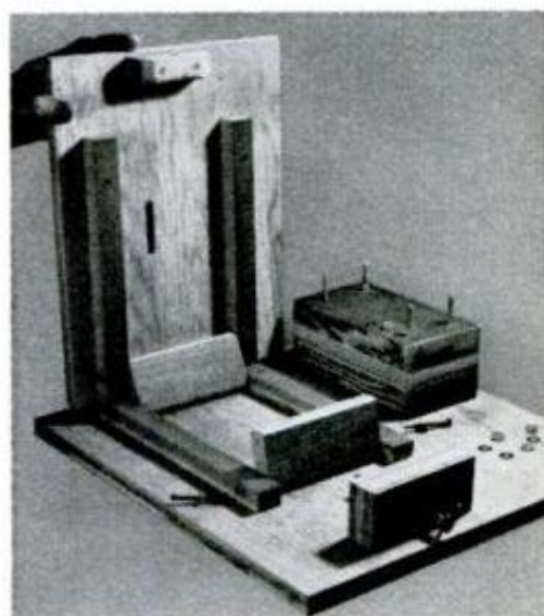
BY REMOVING two pivot screws from the parallel bar unit, upper bars can be swung up for installation or removal of the table
