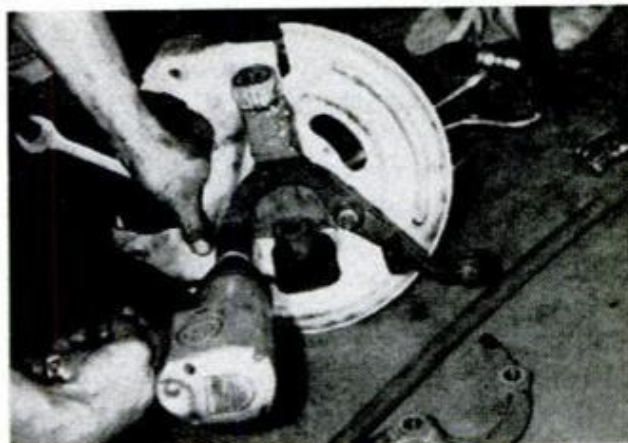
UNBOLT SUPPORT ARM from new disc-brake backing plate and replace with those from drum-brake plate
