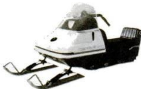
SUPER STINGER 400TX from Scorpion has Para-Rail slide suspension system
