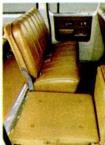
Two-part folding second seat, available Series 10, standard 20. Access to rear. Folds flat to cargo deck.
