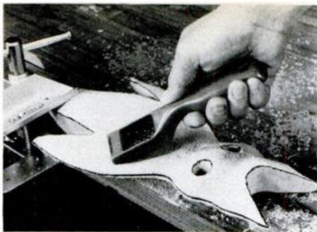
6. NEWEST SURFORM is only one that removes stock by pulling action, works well on convex surfaces
