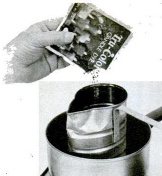
ADD COLORING after wax is completely melted. Stir and allow the coloring to dissolve thoroughly
