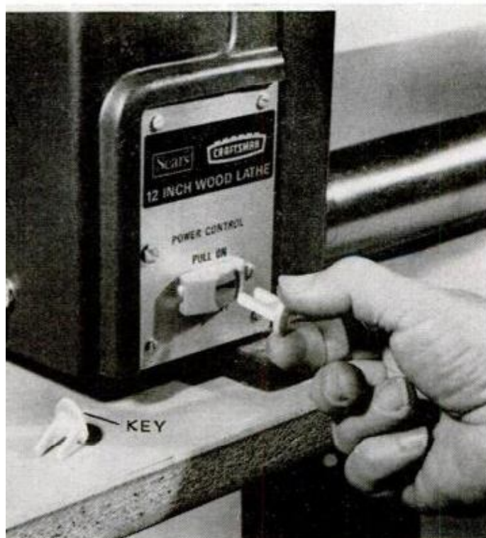
REMOVAL OF PLASTIC KEY from switch prevents unauthorized use of the lathe. Spare key is furnished
