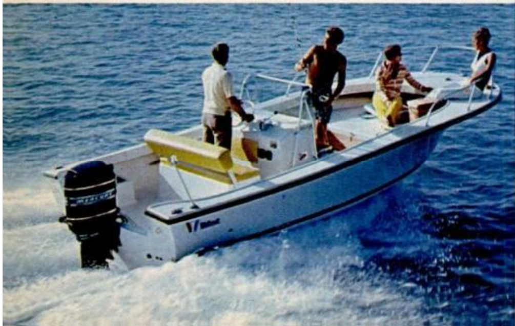
MERCURY 1500 , at 150 hp the most powerful production outboard ever made, can plane a 20-foot Wellcraft Fisherman to 40 mph
