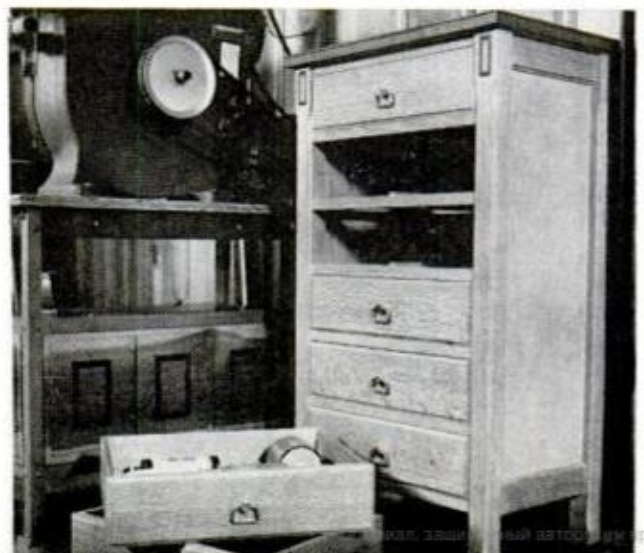
OAK CABINET positioned along wall between the bandsaw and drill press is used to hold accessories and related equipment for both tools. Fred practiced recessing of drawer fronts when he built the six drawers
