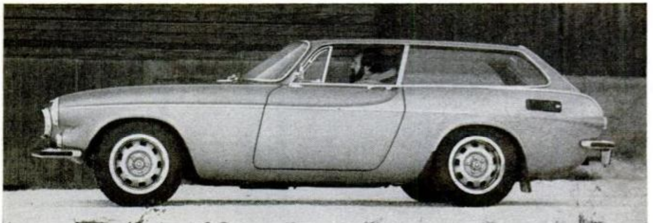
1800ES has wheelbase of 96.5 in., length 172.6 in., width 66.9 in., height 50.4 in., track f/r 51.6 in.
