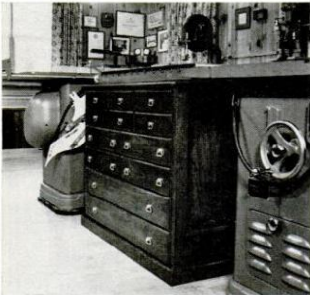
LONG WORKPIECES are supported by rollers on cabinet as they leave bench saw. The walnut cabinet is built so that rollers are just below saw-table height. The cabinet has 24 half-depth drawers, 12 on each side
