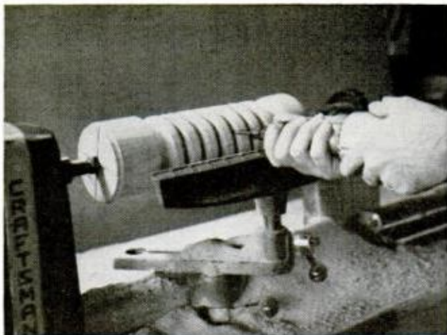
SPIRAL GROOVE IS CUT fastest with electric hand grinder and burr cutter; can also be filed by hand
