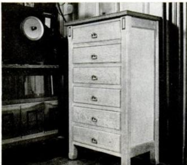
OAK CABINET positioned along wall between the bandsaw and drill press is used to hold accessories and related equipment for both tools. Fred practiced recessing of drawer fronts when he built the six drawers
