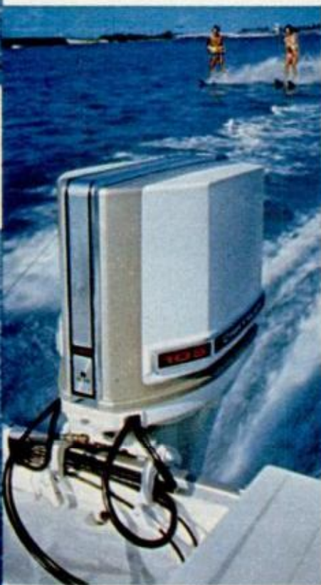
STARFLITE 135 , Evinrude's new line-topper mounted here on the high-styled Glastron, uses hydraulic assist for an improved shift
