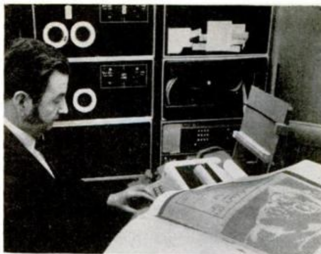
SCOREBOARD COMPUTER in Pittsburgh's Three Rivers Stadium controls thousands of individual light bulbs precisely, to flash pictures and messages. Print-out of one scoreboard pattern is in foreground
