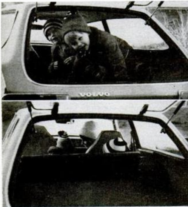
SEAT DOWN results in cargo area that's 60 in. long by 49 wide by 22.4 high. That's nearly 35 cu.ft.
