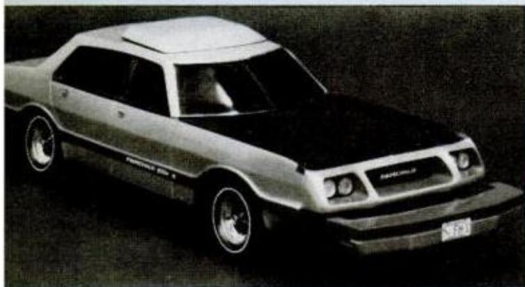
FAIRCHILD ESV has front bumper that automatically protrudes farther as speed of the vehicle increases
