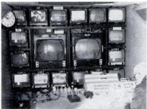
MONITOR SCREENS in control van show as many as a dozen camera views for director to pick from. Actual pictures transmitted appear on center screens
