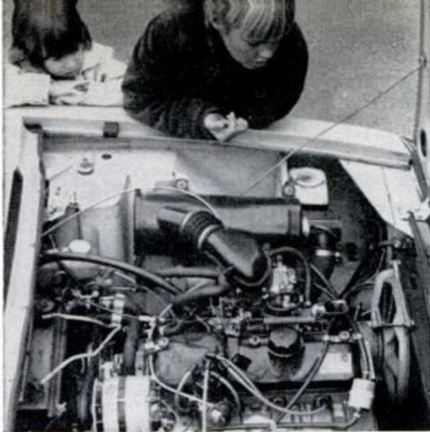
PERFORMANCE of longitudinally placed, aluminum-alloy Four is as exhilarating as it is economical
