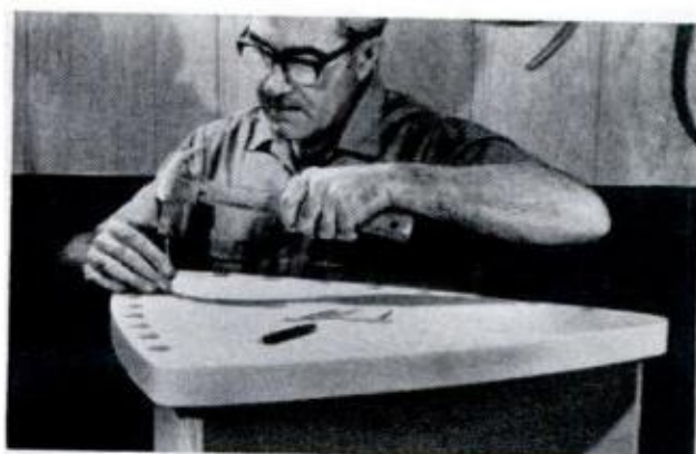
HOLD OFF LAMINATING plywood top until it's glued and nailed to the sides with 2\frac{1}{2} -in. finishing nails
