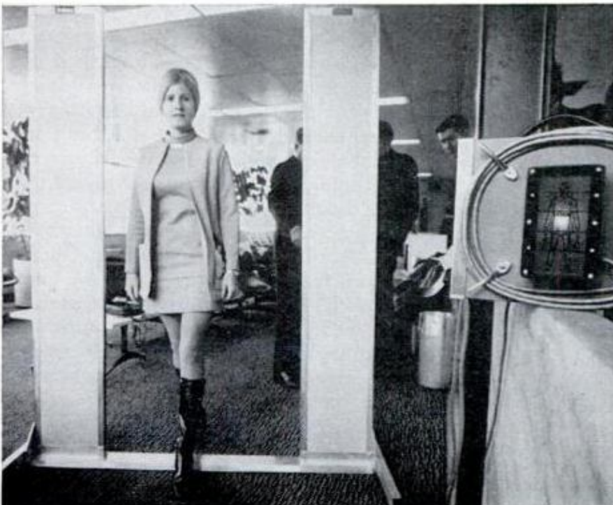
IMPROVED MAGNETOMETER not only indicates presence of metallic objects, but also pinpoints their location by lighted area on small nearby screen. At left, light shows girl is carrying gun concealed
