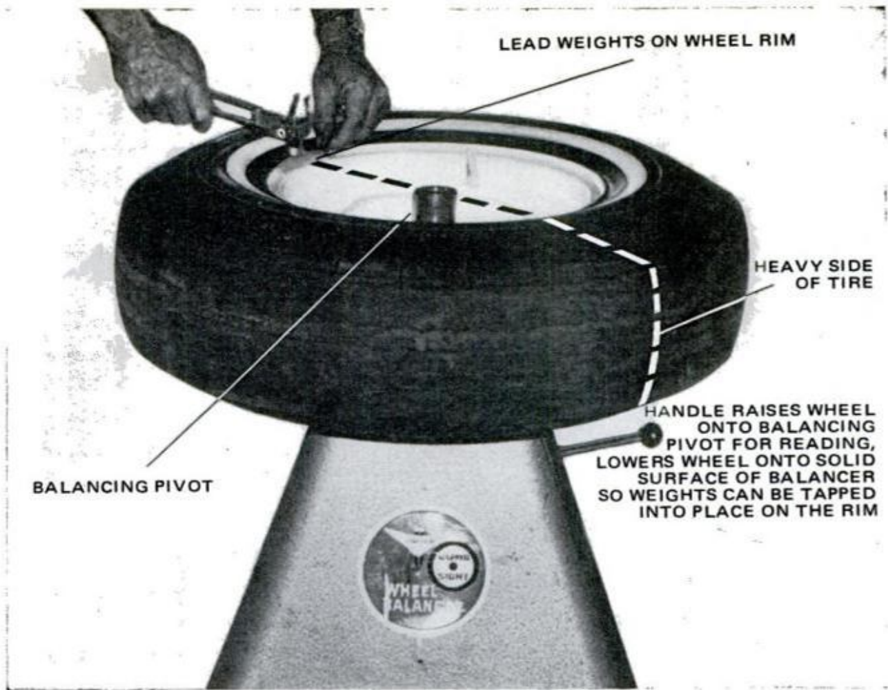
STATIC BALANCER , which is good for about 70 percent of balance problems, is just a seesaw in principle
