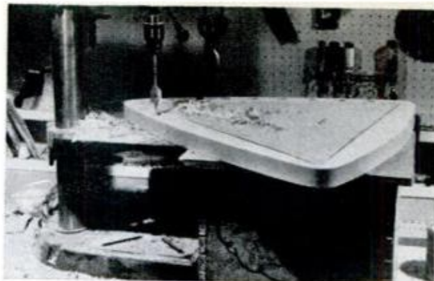
SUPPORT THE HEAVY PIECES on drill press for neat drilling job. Holes in the base are only \frac{3}{8} in. deep
