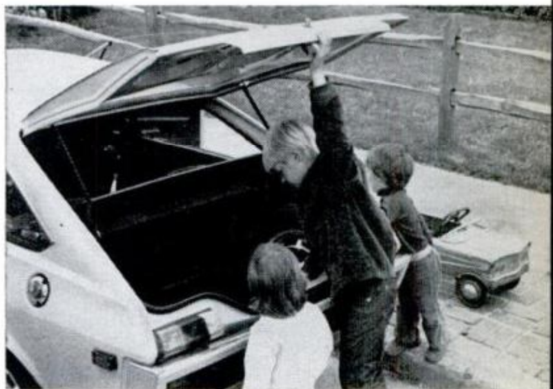
THIRD DOOR LIFTS to swallow 8.5 cu. ft. of luggage. Overall, usable capacity of the trunk is 10.5 cu. ft.
