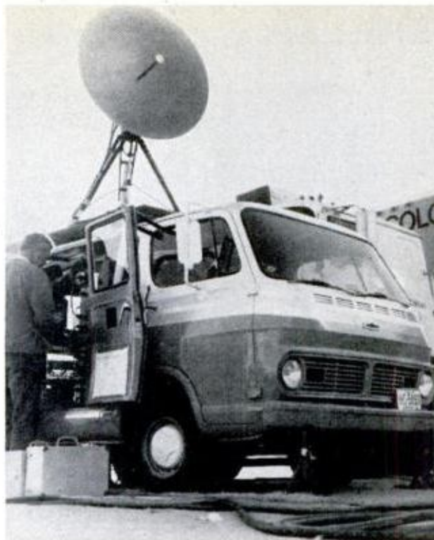
MOBILE MICROWAVE TRANSMITTER relays TV signal from golf course to distant receiver. Signal then goes over telephone lines to TV broadcast stations
