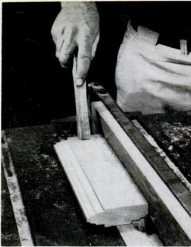
EDGE BEING SHAPED must have maximum support. Here, fence shifted to left of the blade provides it
