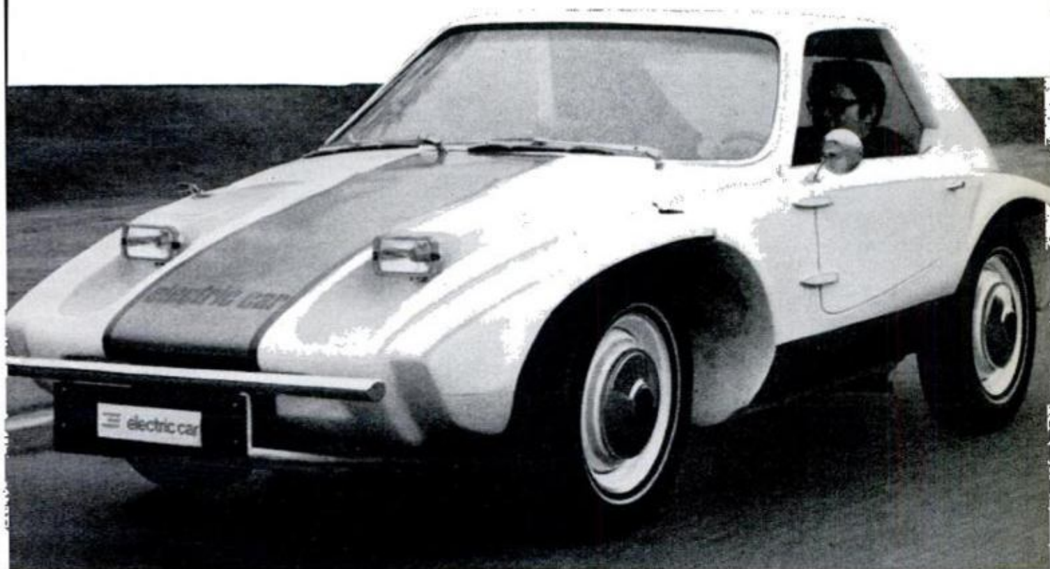
BATTERY PACK in experimental Transit IV runs through center of chassis. It can be charged in place or slid out for change
