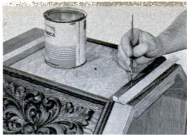
BAND OF CONTACT CEMENT is applied to laminate along edge of masking tape with a small paintbrush
