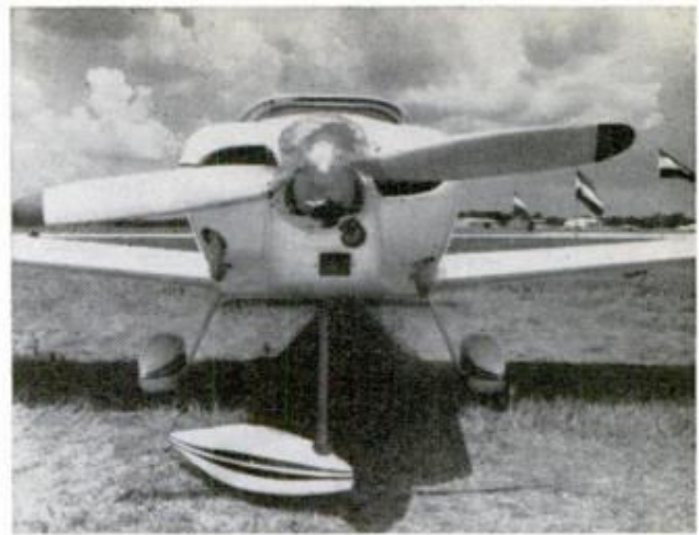
THE SIDEWINDER has a fixed, tricycle landing gear with spring-steel supports. For easy maneuvering on ground, the nosewheel swivels as much as 70°
