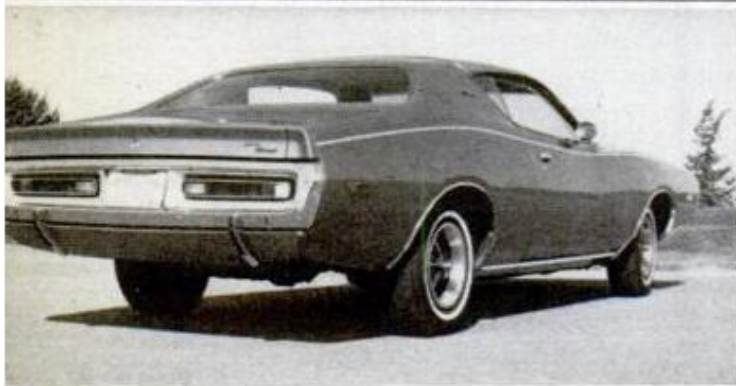
GOOD HANDLING , roadholding, but wide pillars and small rear window make backing a time for prayer
