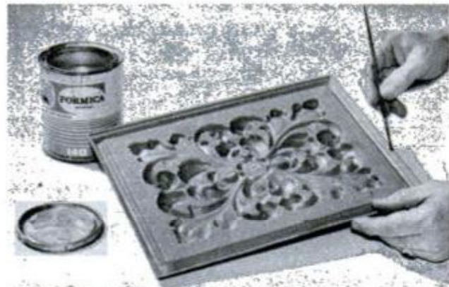
CONTACT CEMENT IS APPLIED also to back of carved panels at the center and along top and bottom edges
