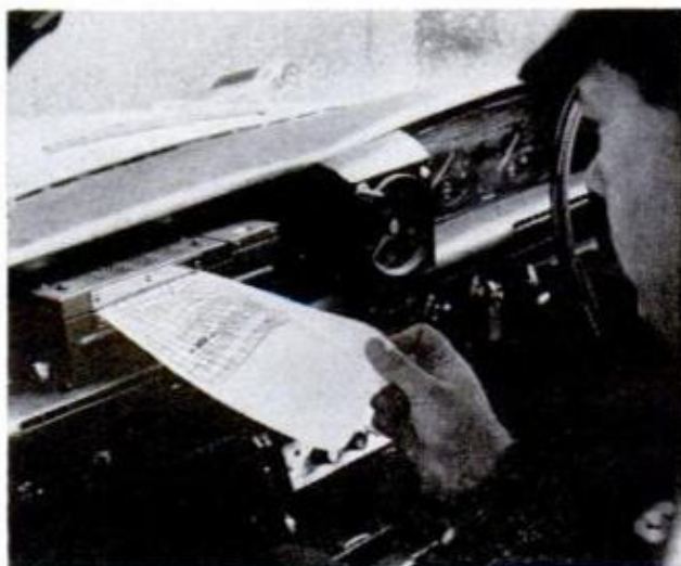
POLICE-CAR FACSIMILE SYSTEM transmits maps, photographs of suspects and missing persons, written messages, stolen-car lists and other information to squad cars in Bristol, England. Facsimile transmissions can't be intercepted by ordinary radios or misunderstood. Messages are 4 1/2 inches wide and as long as needed. Equipment costs about $1500 per car: most of it fits in the trunk.
