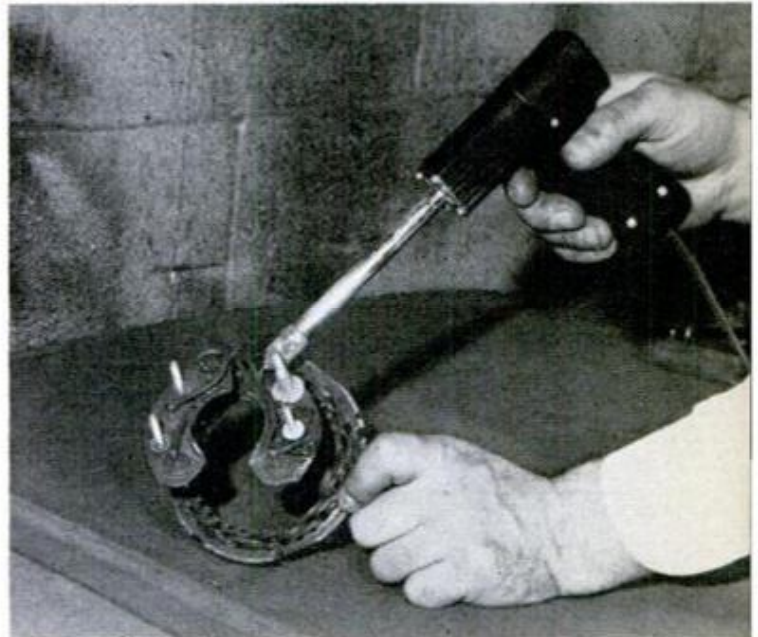
DISCONNECT DIODES before checking them and before bench-testing other components of the alternator
