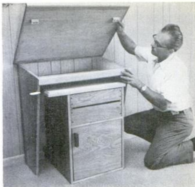
WOOD BLOCKS glued to the underside keep lift-off drawing board in place over the storage compartment
