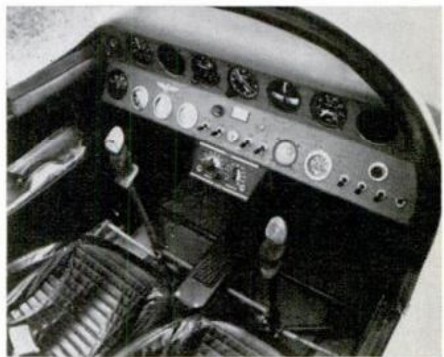
THE PLANE features an exceptionally clean instrument panel layout. There are dual controls—except for brakes—as indicated by two control sticks
