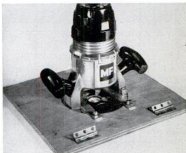
BOTTOM OF TOP PANEL: Router is clamped against metal plate. Two strips make up thickness difference
