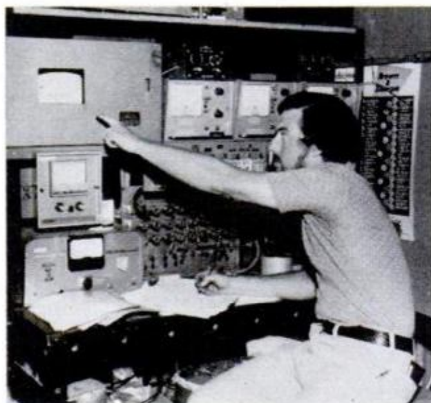
EMISSION LEVELS of hydrogen system are checked in UCLA dyno lab by team co-captain, Frank Lynch
