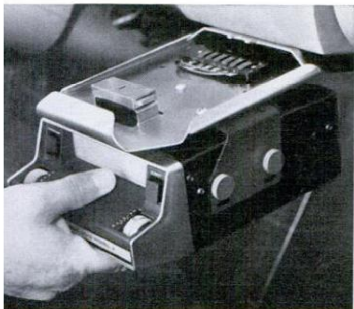
TO PLAY TAPES AT HOME , slip deck out of car (above) and into a matching mount in house (below)
