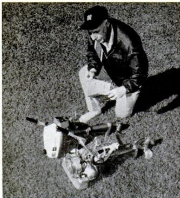
NEWEST two-horse Sea-Horse is 11 pounds less than first model, pivots to reverse, has innards enclosed
