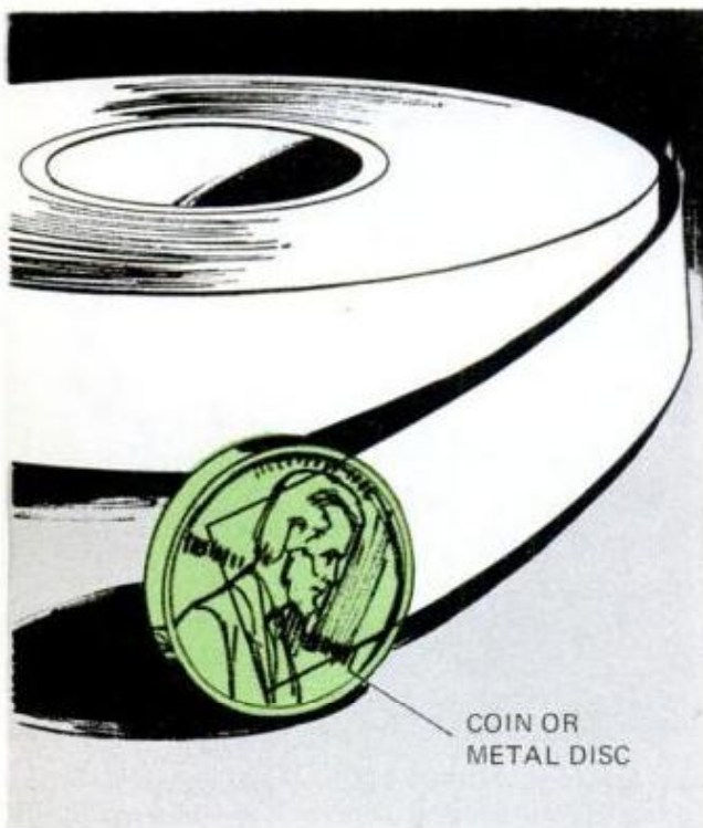
CELLOPHANE TAPE END will be easy to spot if you slip a penny in place before putting away the roll. This stunt saves annoyance of picking at the end with your fingernails or a knife.—Joe Braunstein, New York.
