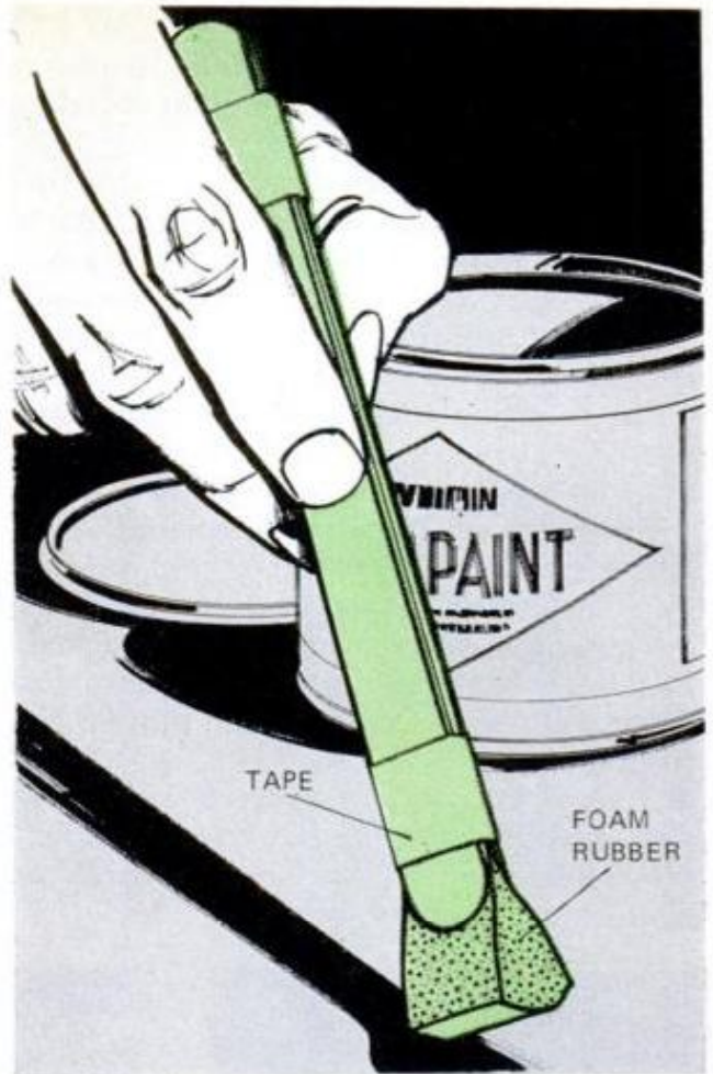
PAINT TOUCH-UP APPLICATOR is made from a \frac{1}{2} \times 1 \times 1\frac{3}{4} -in. piece of foam rubber and two tongue depressors. Clamp half the rubber between tips and wrap ends with tape.—G. Bertrand, Le Saules, Que.
