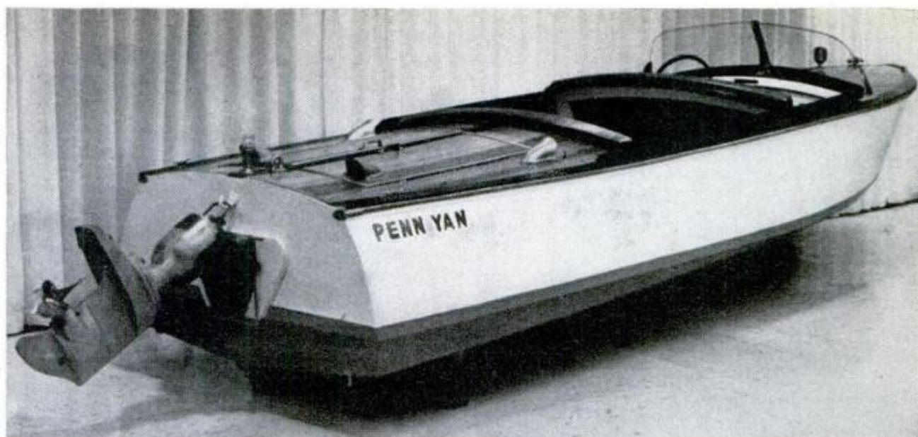
1930 STERN DRIVE , from Johnson Outboards and Penn Yan Boats, came too soon and was depression victim
