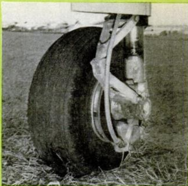
LANDING GEAR is attached directly to wing spar. Hefty shocks take the bumps out of rough landings
