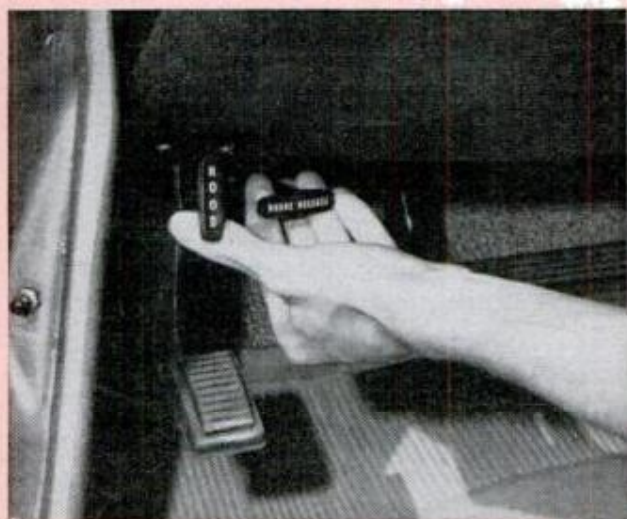
RELEASE PULLS for hood and emergency brake stand too near each other. Drivers often confuse the two
