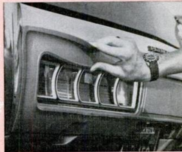
REAR-BUMPER RUBBER , supposedly permanent, pulls away. Platers say it makes bumper hard to straighten
