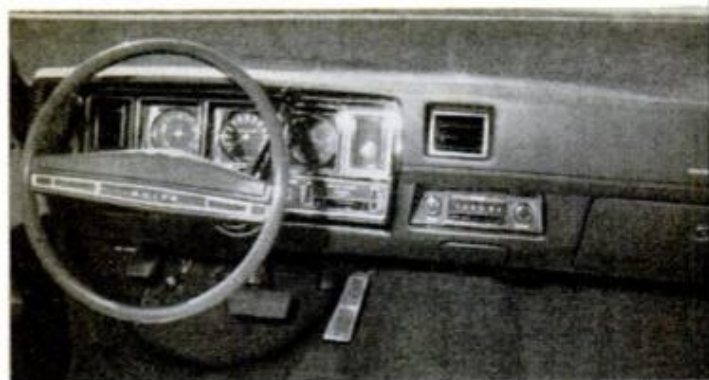
HORN BUTTONS in steering-wheel spokes are hard to locate in emergencies. Owners would like ring back
