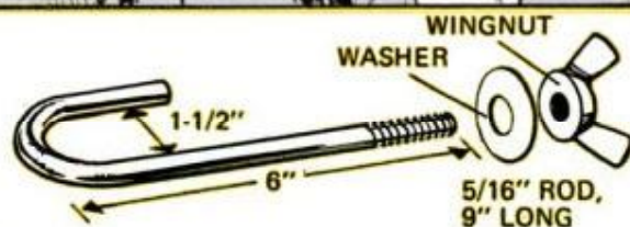
MAKE A WINDOW "SPANNER" for your ladder by bending two J-hooks from 5/16-in. rods threaded at one end. Short leg goes in blind hole; the long one receives washer, wingnut.—Andrew Vena, Philadelphia
