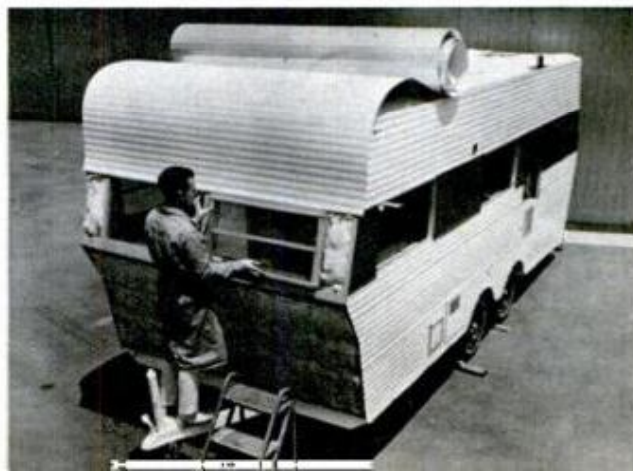
CONTINUOUS ROLL ROOFING is started at front above windows. Latter inserts into "Pittsburgh" lip
