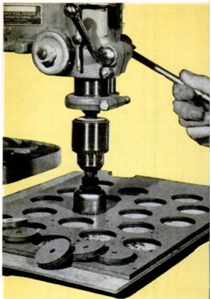
BALL HOLES are bored in hardboard sides with a 1\frac{1}{4} -in. hole cutter in a drill press
