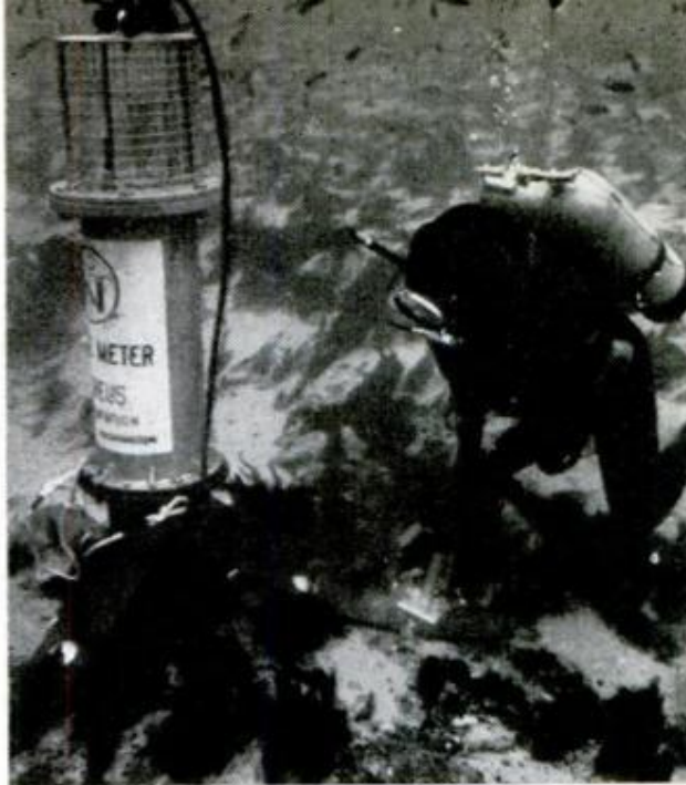
SURGE METER was fixed to summit with explosive bolts. Instrument was damaged by fishing trawlers
