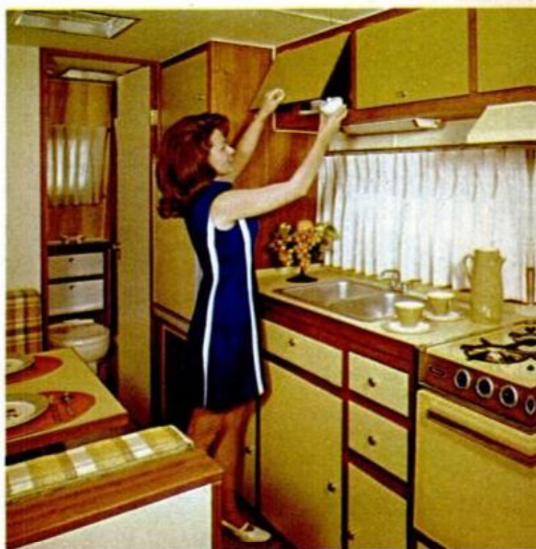
LOTS OF DRAWER SPACE and cabinets, plus pullout cutting boards are in dream camping kitchen. Plumbing fixtures are connected to a 6-gal. water tank and a 30-gal. waste-holding tank (to make the unit independent during extended on-the-road time). Comfortable dinette at the left converts into a roomy bunk to sleep two adult-size vacationers
