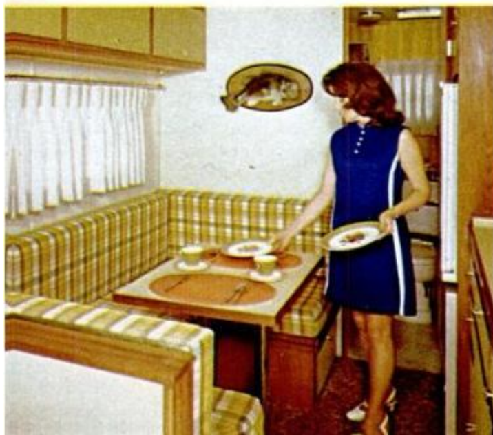
LOTS OF DRAWER SPACE and cabinets, plus pullout cutting boards are in dream camping kitchen. Plumbing fixtures are connected to a 6-gal. water tank and a 30-gal. waste-holding tank (to make the unit independent during extended on-the-road time). Comfortable dinette at the left converts into a roomy bunk to sleep two adult-size vacationers
