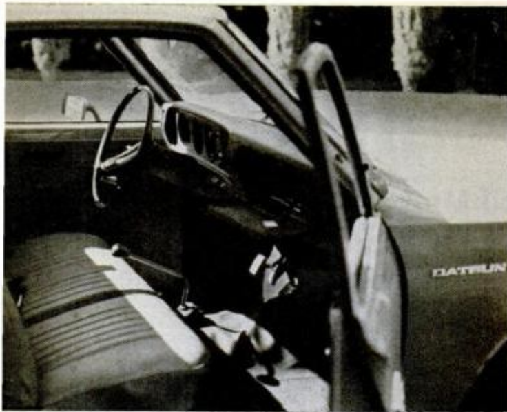
DATSUN PL-620 interior is neat and functional. Re-design of the side glass eliminates wind wings. There's more legroom, thanks to slightly longer cab
