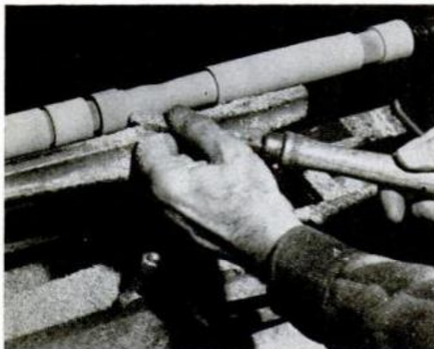
LONG, THIN SPINDLES tend to vibrate, so work the center area first. Thick ends minimize bouncing
