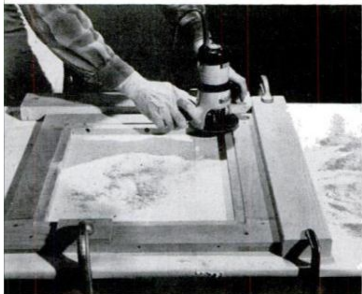
ROUT RABBET FOR HARDBOARD INSERT before sides are attached. Clamped 2x4 limits width of the cut
