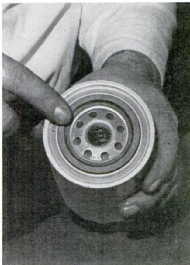
OIL FILTER GASKET should be coated with oil before installation. Do not overtighten the filter
