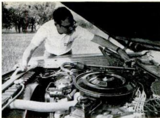
ELECTRONIC IGNITION (on firewall) uses no points, can't wear, keeps emissions low and engine in tune
