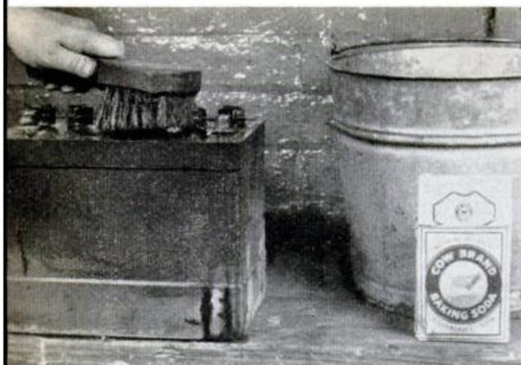
BAKING SODA neutralizes acid on battery case. Be careful to avoid getting solution into the cells
