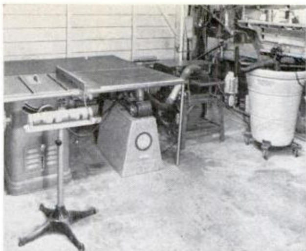
DUST-COLLECTING UNITS are on nearly all tools in shop. Dust they miss is inhaled by the shop vacuum
