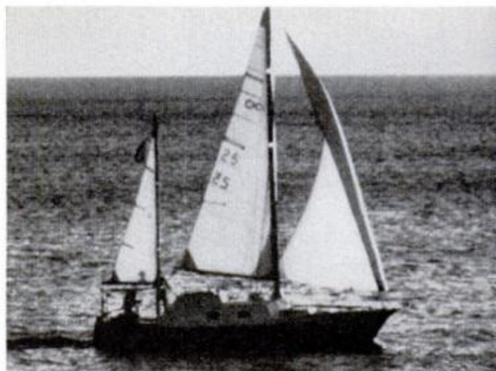
UNDER FULL SAIL , Queequeg carries a large jib, mainsail and smaller after sail on the mizzenmast
