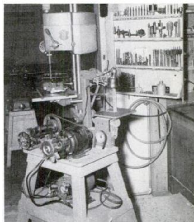
DRILL-PRESS ACCESSORY BOARD is hinged for convenience; Stanley dowel machine converted to power
