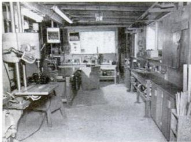
NEW SECTION OF SHOP features evaporative cooler and space heater, both suspended from the ceiling
