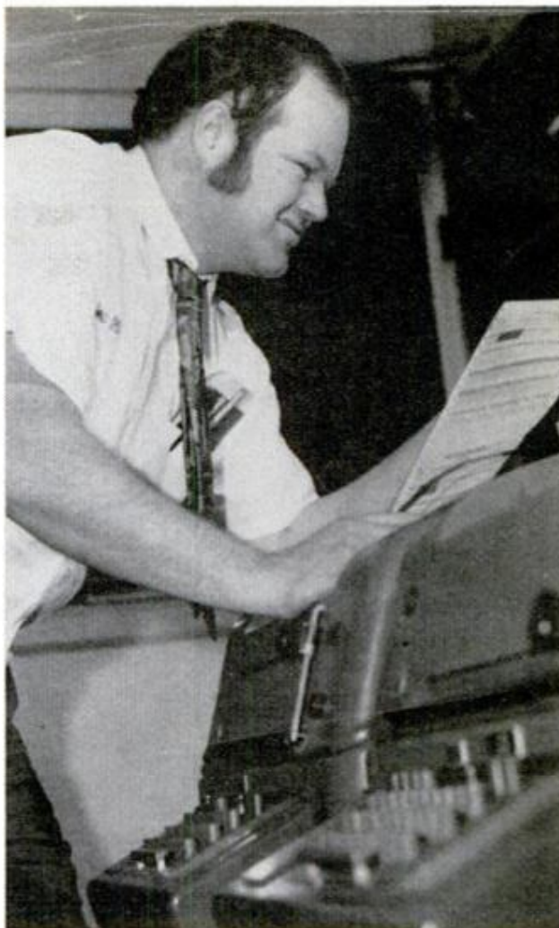
CAR-BUILDING ORDER is received by a teletype machine in scheduling booth at Pontiac Motor Div.
