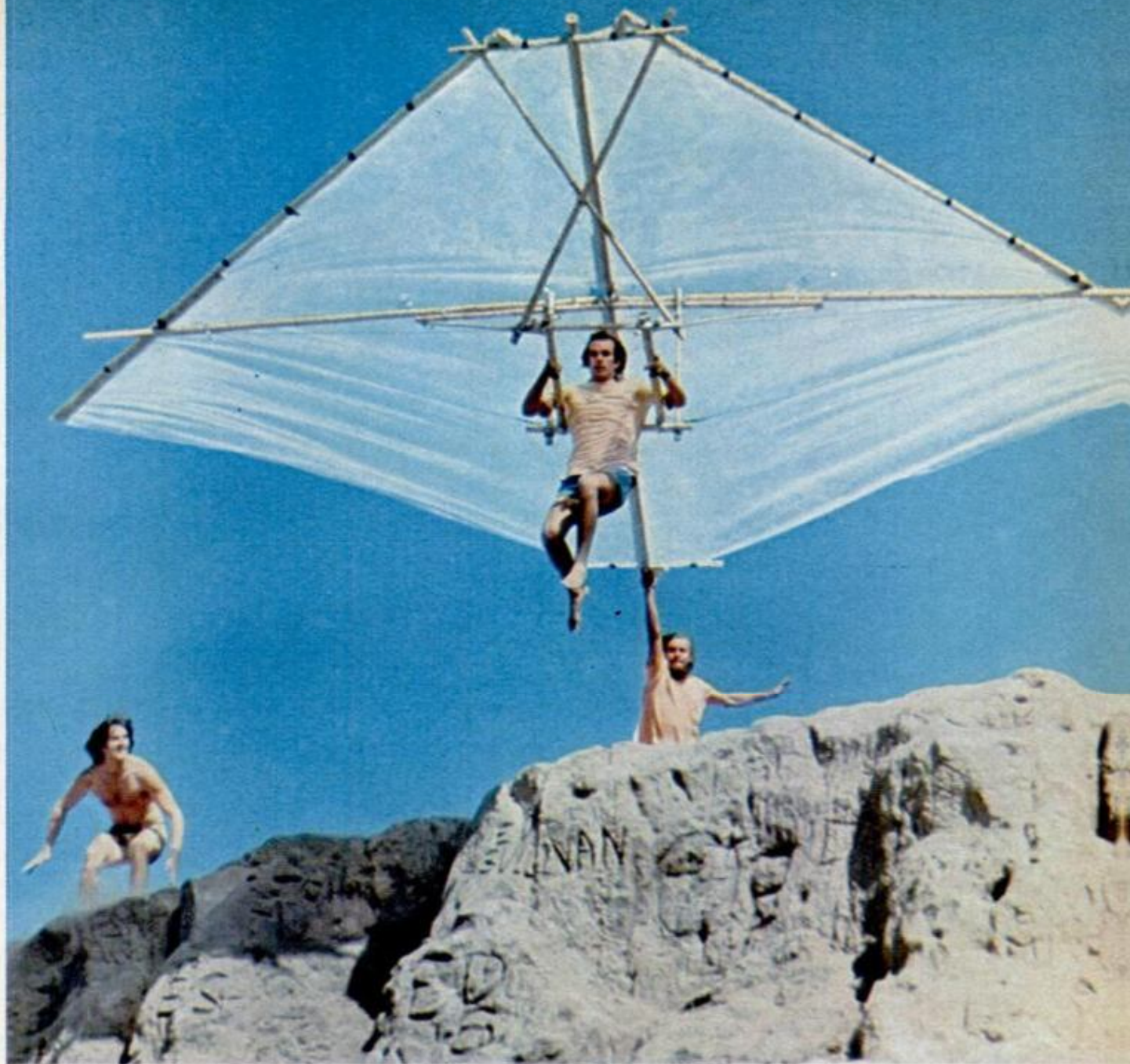
LAUNCHING HIMSELF FROM A CLIFF , California kiteman gets a helpful push from assistant above. Below, another surfer skirts mountain ridge, riding updraft. Both kites are Rogallo types. At right is a bi-winger reminiscent of Wright brothers' design
