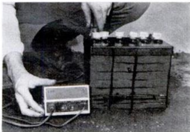
TRICKLE CHARGER provides safe, slow recharge of battery, and it's the least expensive type available
