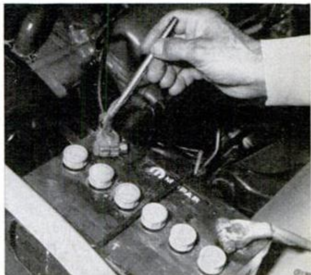
TERMINAL LUBRICANT or petroleum jelly should be applied to connections to retard corrosion buildup
