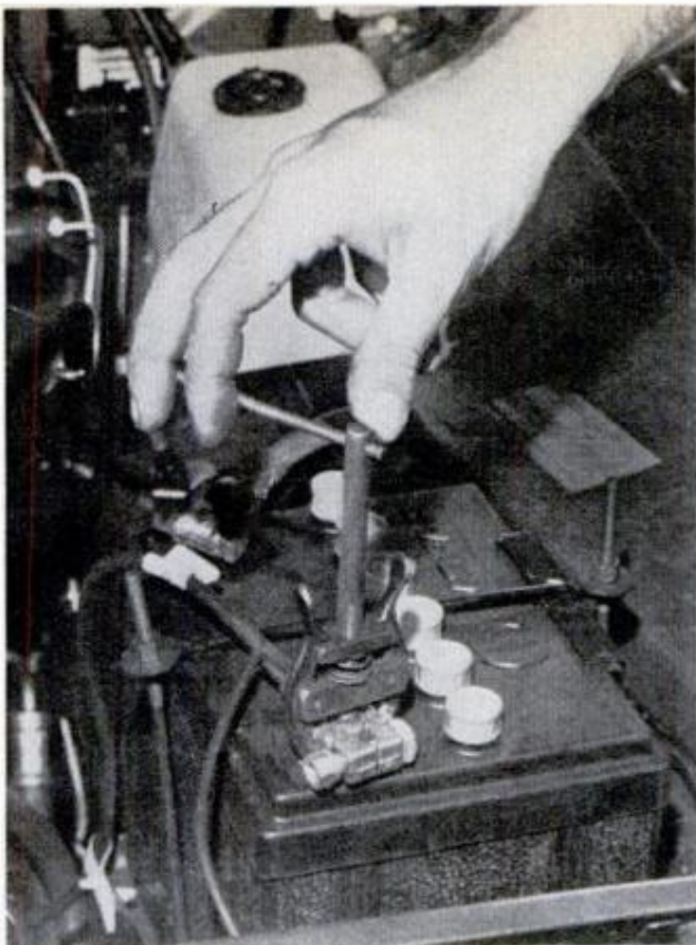
CABLE-TERMINAL PULLER applies leverage to lift up the terminal off of the battery post. It's a must
