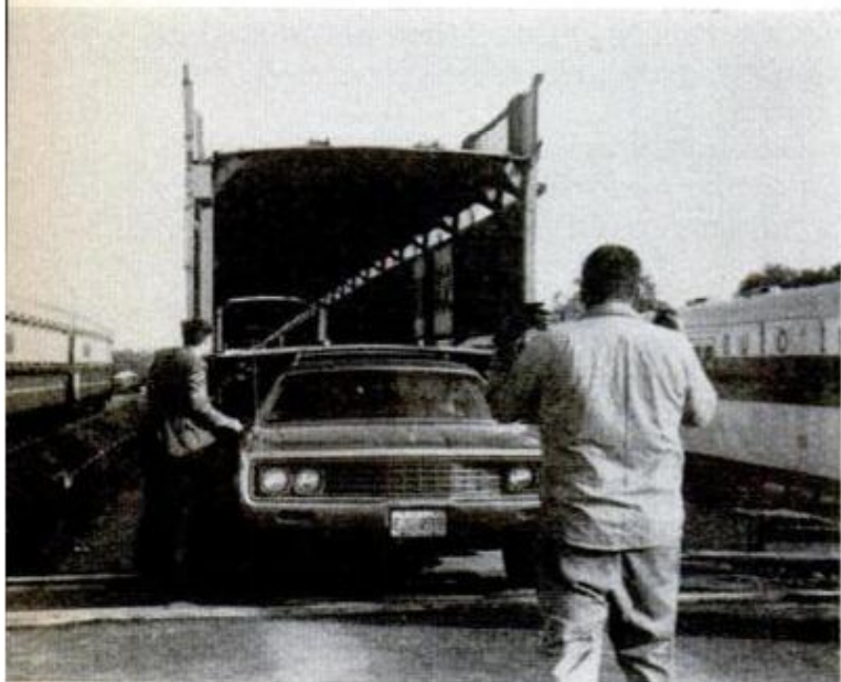
UNLOADING OPERATION in Florida moves smoothly. A car is rolled off ramp about every three minutes
