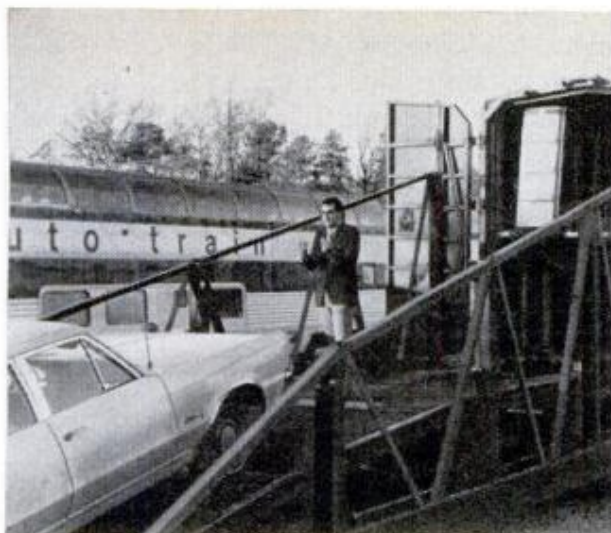
AT TERMINAL , attendants drive cars up ramp for loading. Here author's wagon heads for lower deck
