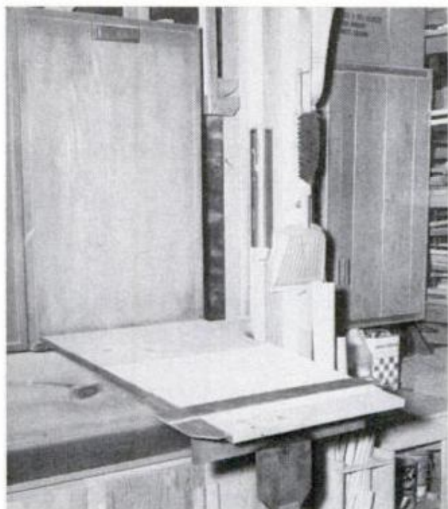
DRAWING BOARD ready for action. When not needed, board flips up against cabinet and stays dustfree
