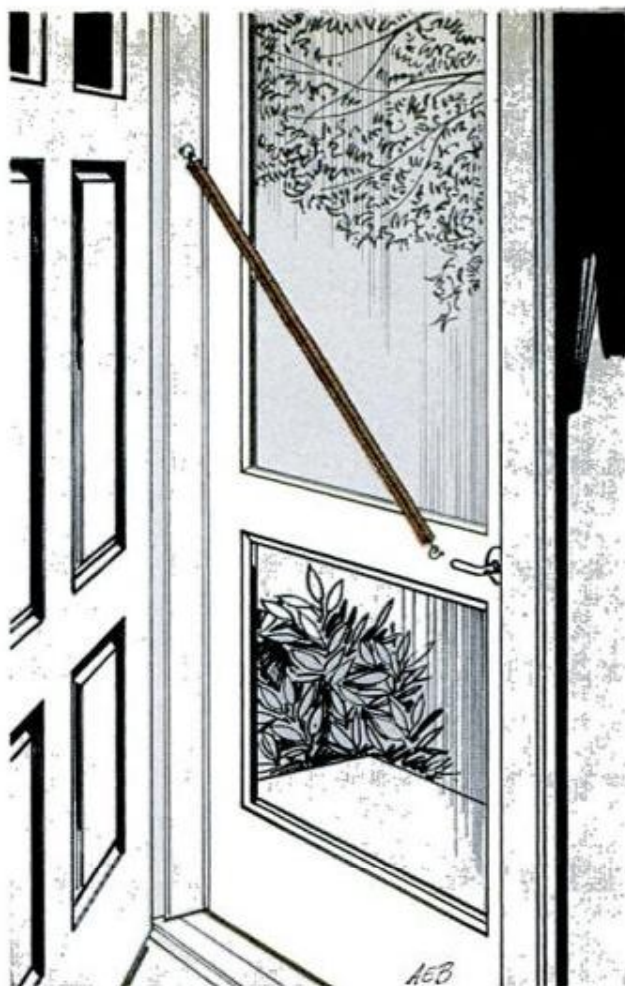
SCREEN-DOOR-CLOSER SPRING can also be used to correct any minor sagging. Simply fasten outboard end at an angle until the frame is pulled into square.—Dennis G. Richardson, Perkinsville, Vt. Illustrations by Adolph Brotman
