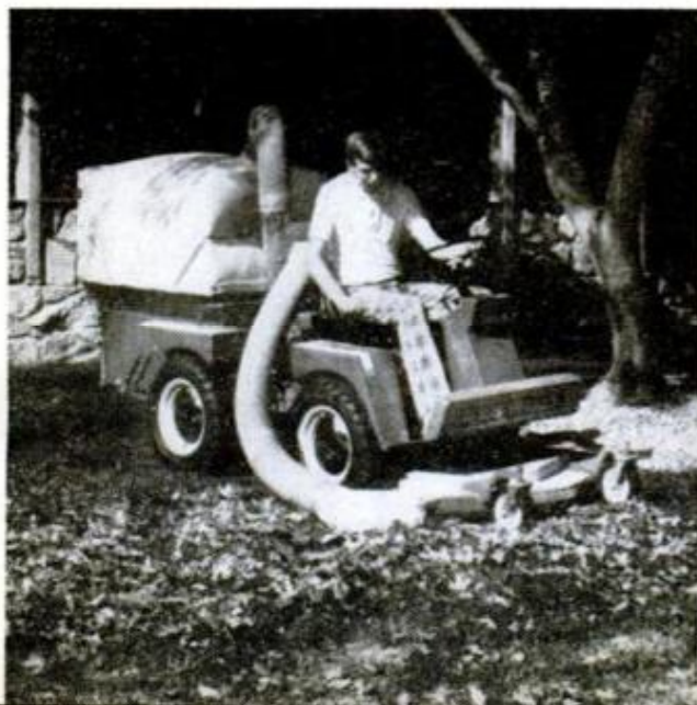
VACUUM PICKUP is powered by GMT's engine, feeds leaves, clippings into a 20-bushel box on carryall. A 15-foot snorkel attachment reaches under shrubs
