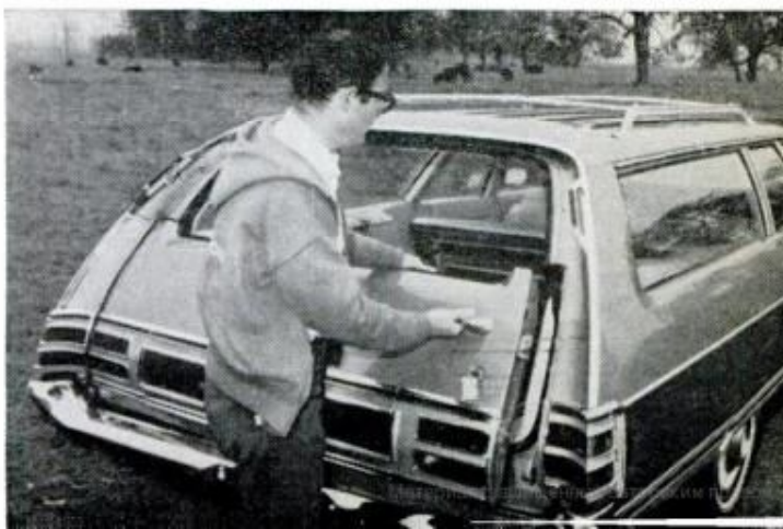
AUTO-LOCK SYSTEM for tailgate keeps it locked if key is on. Gate swings open even with window up
