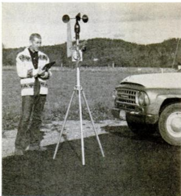
AIRCRAFT-TYPE wind recording gauges showed that velocity can influence gas consumption of RV rigs
