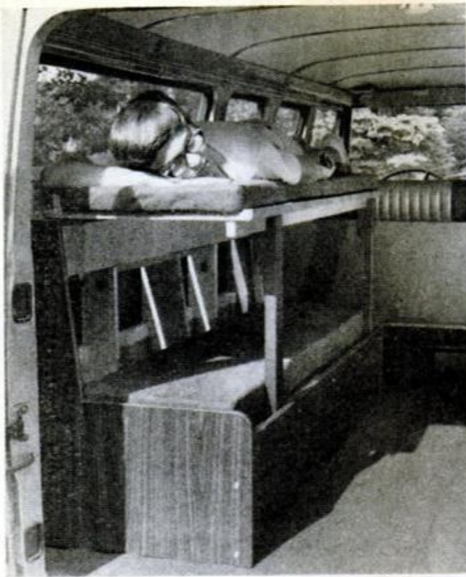
DOUBLE-DUTY BENCH-BUNK serves three functions—as daytime seat, as upper and lower berths at night and as a spare storage bin for sleeping bags and gear at any time. Such items as flashlights, pencils, insect repellent and reading materials are stored along back in easy reach
