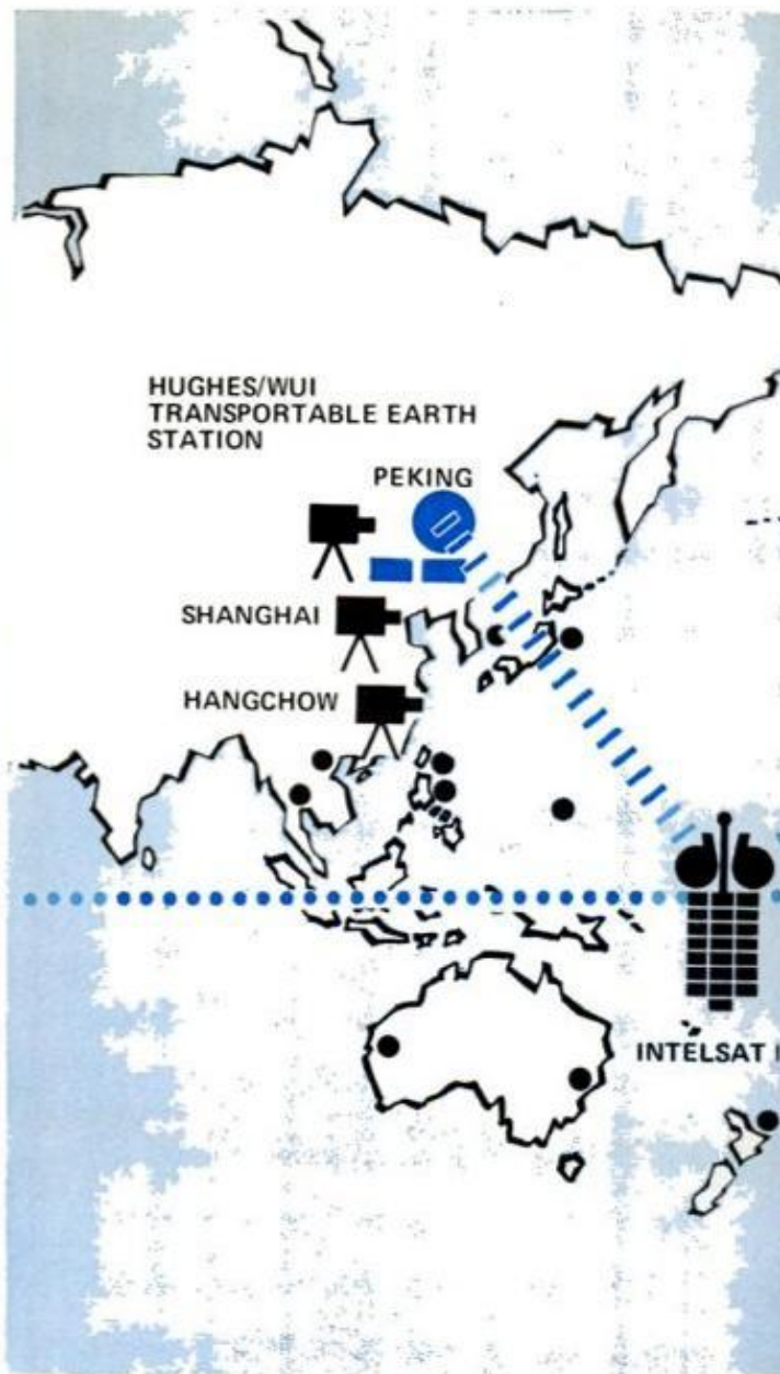
GROUND STATION was flown to Peking prior to the President's visit. Made by Hughes Aircraft, the facility boasts a 24-foot-diameter antenna and enough electronics to transmit 1 color TV broadcast, 9 voice commentaries and 60 two-way phone conversations. It beamed transmissions to Intelsat IV, as shown in the drawing
