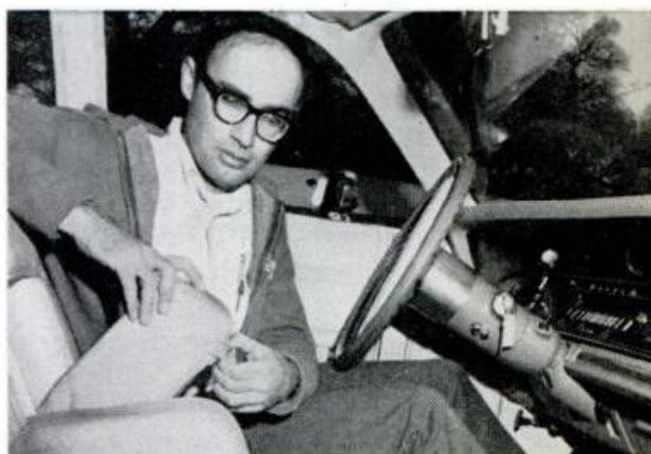
TWIN ARMRESTS up front fold for center passenger. In two-seat wagons lockable storage is under floor
