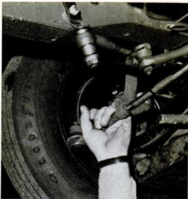
LOOSE TIE RODS are a major cause of front-end shimmy. Also check steering idler and pitman arms
