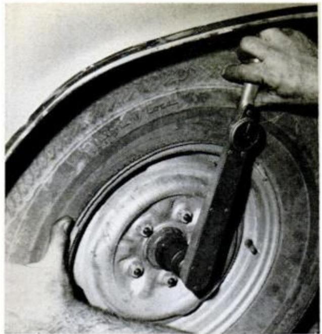
FRONT-WHEEL BEARINGS that are too loose can be felt as shimmy in steering wheel. Torque to spec
