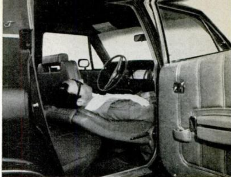
OPTIONAL RECLINING SEATBACKS are real favorites with Ambassador owners, but headrests tend to stick
