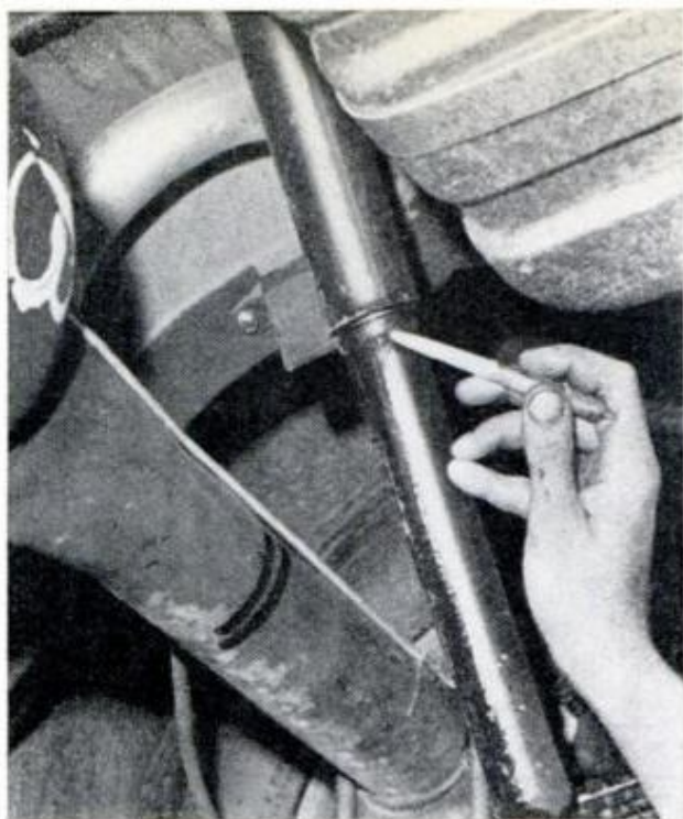
BAD SHOCKS can cause vibrations. Check for fluid leaks and that mounts are tight at top and bottom
