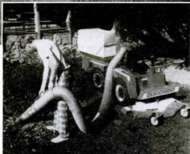
VACUUM PICKUP is powered by GMT's engine, feeds leaves, clippings into a 20-bushel box on carryall. A 15-foot snorkel attachment reaches under shrubs
