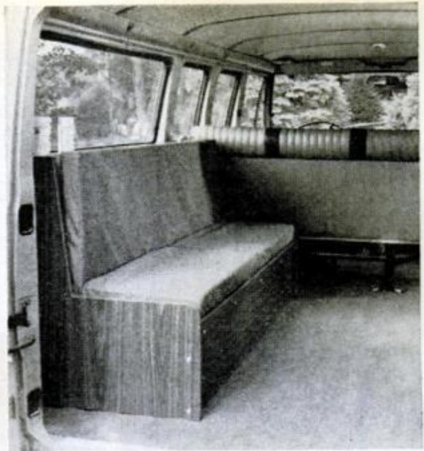
DOUBLE-DUTY BENCH-BUNK serves three functions—as daytime seat, as upper and lower berths at night and as a spare storage bin for sleeping bags and gear at any time. Such items as flashlights, pencils, insect repellent and reading materials are stored along back in easy reach
