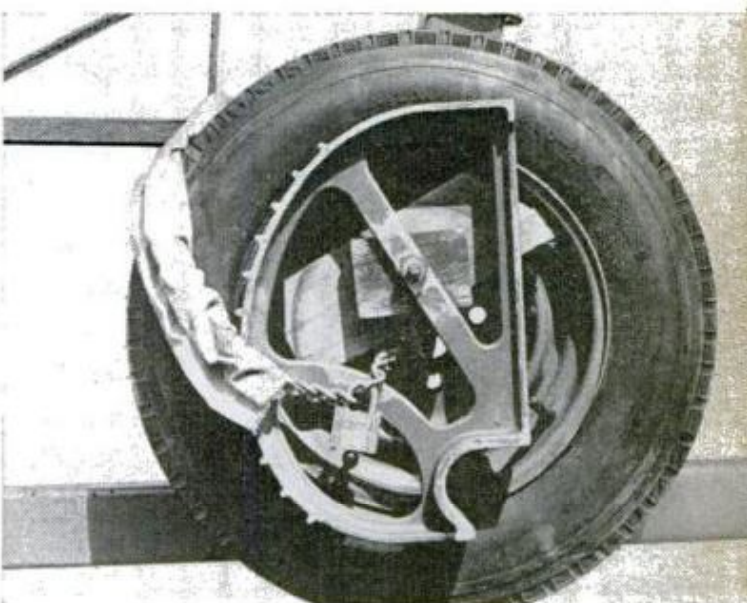
SPARE TIRE AND TRAILER JACK can be bolted to the trailer with a length of 1/2-inch rod stock and then secured with a lock and chain in a cloth sleeve
