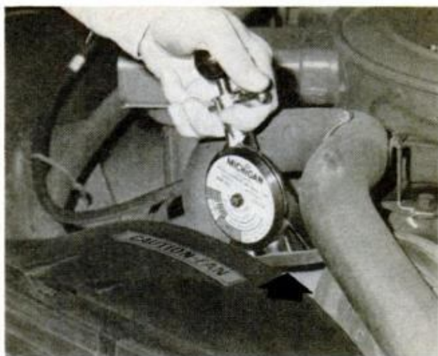
FAN-BELT TENSION GAUGE sets tension to spec as it must be on engine with many power accessories
