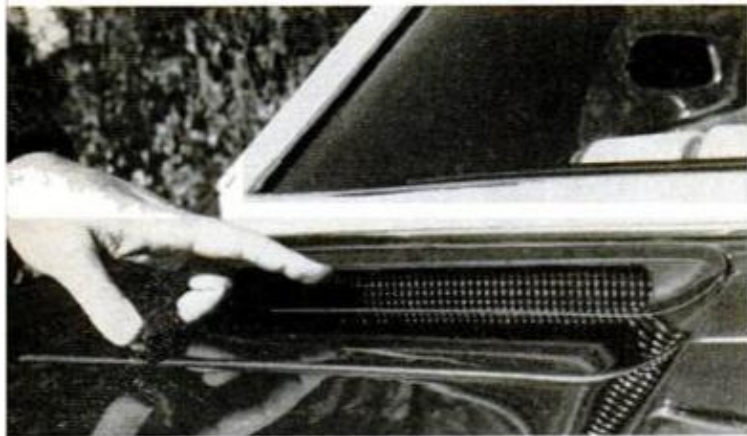
TORONADO SECONDS taillights under rear window. Drivers two to three cars behind see signals easily
