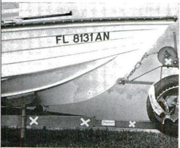
Xs MARK THE SPOT: Reflective tape makes your rig visible when it's towed or parked at night or in fog. Tape's particularly helpful on unloaded trailer
