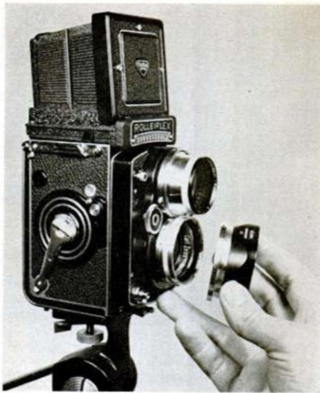
ROLLEIFLEX OWNERS can take close-ups with this set of Honeywell Rolleinar accessory lenses, one for upper viewing lens and one for the lower taking lens. Resulting focusing range is 9½ to 12½ inches
