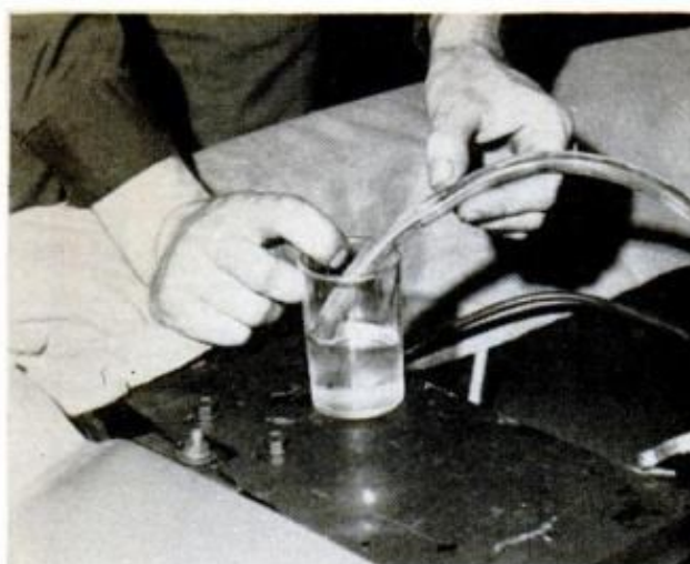
AIR OR GAS LEAKS in the cooling system can be detected very simply (see procedure given in text)
