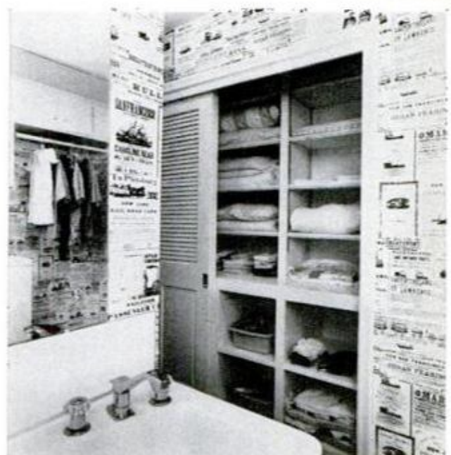
TOWEL CLOSET convenient to sink has louvered bypassing doors to insure adequate circulation of air
