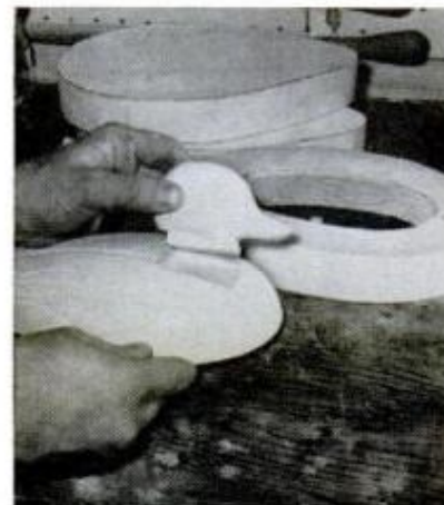
CUT RECESS IN BODY and fit head into the slot, securing it in place with waterproof glue, screw
