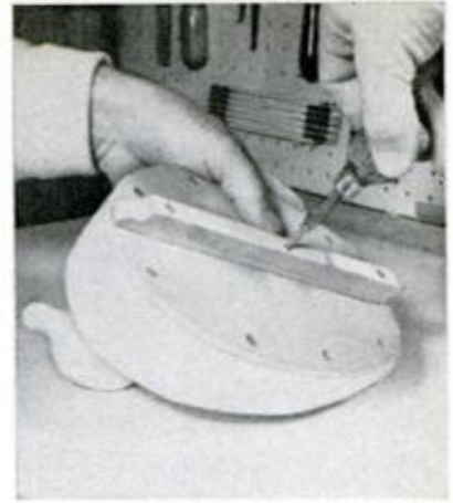
BOTTOM PLATE IS GLUED and screwed on, followed by keel. A lead-weighted keel steadies decoy
