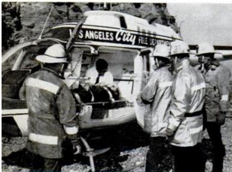
HELICOPTER AMBULANCE can carry two injured persons on stretchers plus an equipped first-aid man
