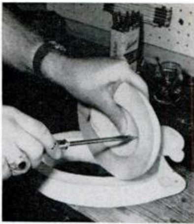
SCREWS ARE USED in the final assembly to hold head to body and all sections glued together
