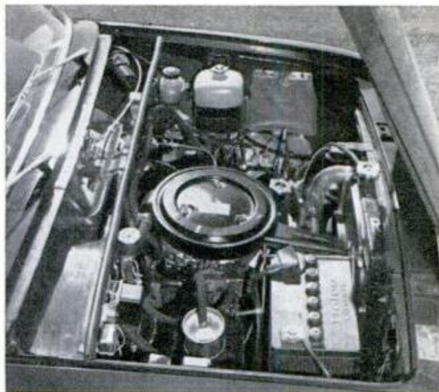
SEDAN AND WAGON use familiar overhead valves in four-cylinder engine; sports models, overhead cams
