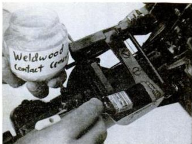
APPLY contact cement to carpet and metal bracket
