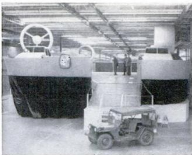
LANDING CRAFT (shown in a full-scale mock-up) designed to carry a 60-ton tank plus fighting men
