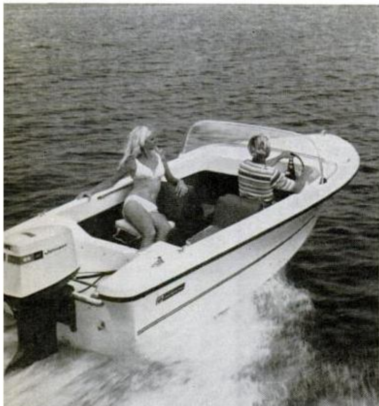
NEW SEAHORSE by Johnson is 65-hp three-cylinder model claiming better fuel economy than former 60
