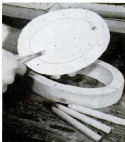
REASSEMBLE the two body halves after cutting center out of lower half to give decoy lighter weight
