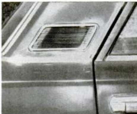
EXHAUST VENTS in the C-pillar are for a flow-through ventilation system
