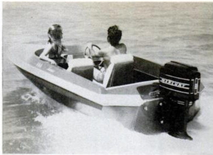
MERC 650 is a new 49.8-cu.-in. three-cylinder Mercury mill designed for a compact package of 65 hp
