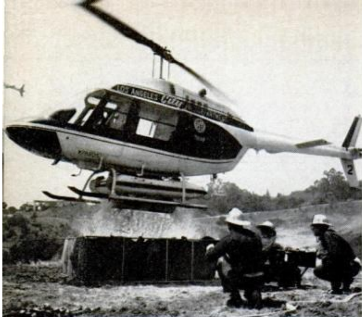
"WATERBOY" HELICOPTER refills 1000-gallon portable bag dropped to firemen far from a hydrant
