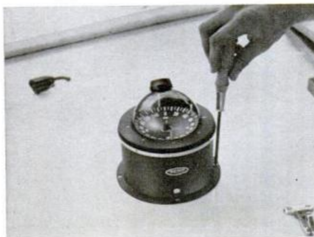
FLAT (OR DISHED) COMPASS CARD has lubber line opposite helmsman, ranges in price from $20 to $300. One above is designed for binnacle mounting
