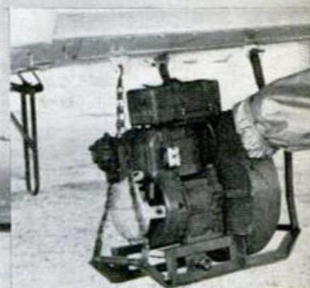
ON GROUND , blower is required to maintain proper pressure in ship's air bags
