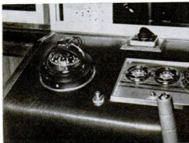
CUPPED CARD COMPASS , sometimes referred to as the direct-reading type, has the lubber line facing the pilot. This type ranges in price from $10 to $50
