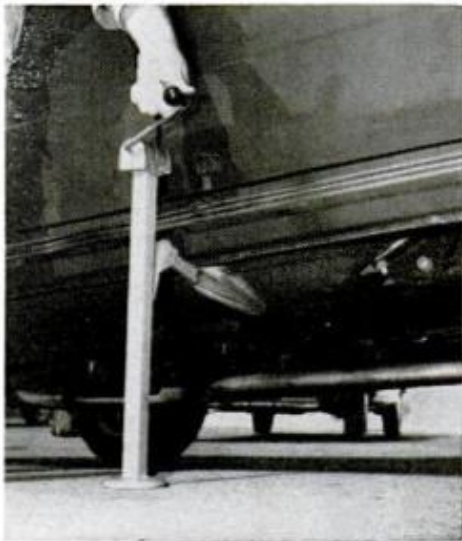
JACK SLOTS on sides are positive and secure as on most imported cars
