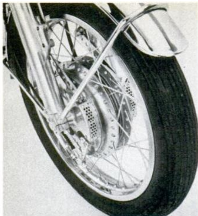
DUAL FRONT BRAKE is actually two brakes on a common drum. We'd prefer an efficient, simpler disc
