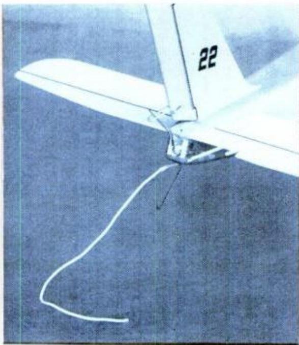
RUDDER LINKAGE holds the rudder full-left with receiver off. Antenna end simply hangs free
