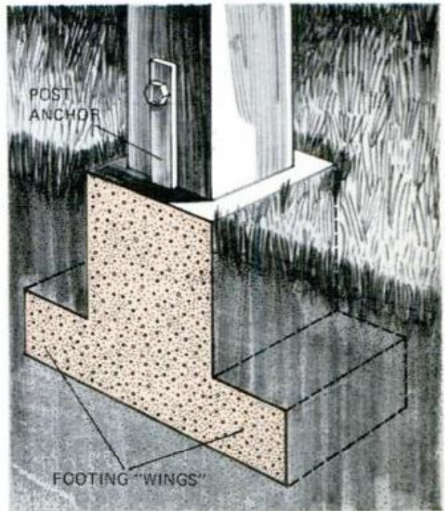
WHEN ROOFS BLEW OFF a few neighbors' patios, I decided to make mine more secure by pouring post-anchoring footings as shown. The trick has worked and our roof is intact.— George Oxford, Boise, Idaho
