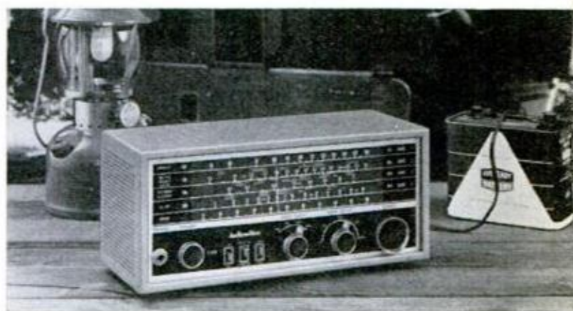
YOU CAN OPERATE this Hallicrafters S-120A on either battery power (above) or on house current. The set, also shown at top of facing page, covers 76 shortwave services plus AM, is priced at $79.95
