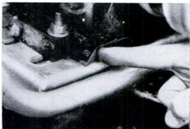
EMERY CLOTH placed between engine and mounting plate will stop engine drift if tightening doesn't
