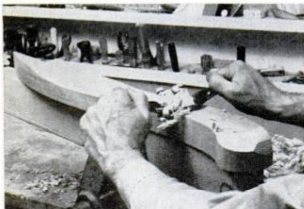
DON'T RUSH SHAPING. Use full-size drawings of contours, plus calipers, to make frequent checks
