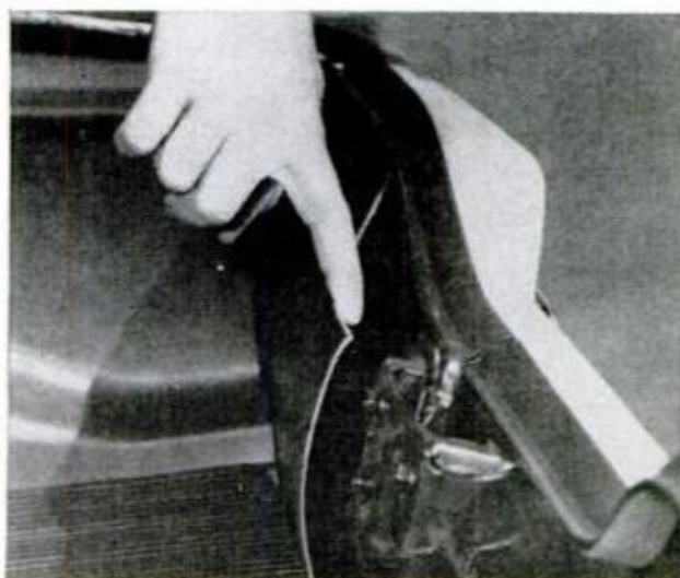
LOOSE PANELS contribute to many Vega owners' mention of rattles and need for better workmanship
