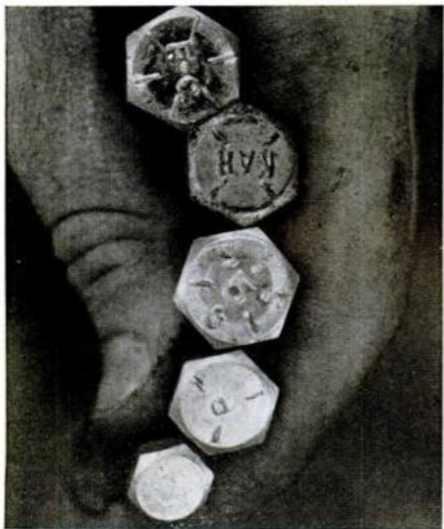
HEAD MARKINGS indicate strength of fastenings from grade 8 at the top to grade 2 at the bottom
