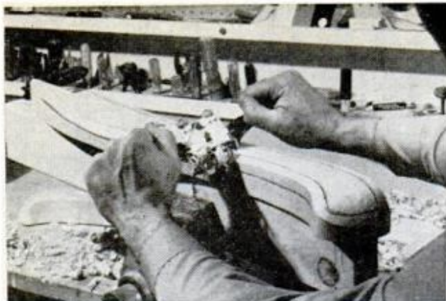
SPOKESHAVE will let you do a slick carving job on the armrests. Various contours are shown at the right
