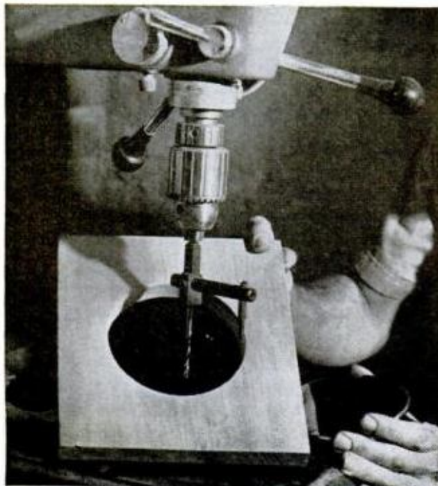
MIRROR CUTOUT in rear panel is made with circle cutter chucked in drill press or with a sabre saw 140
