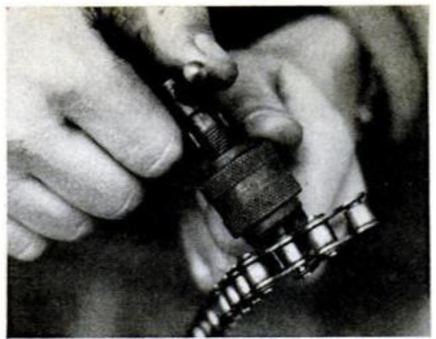
CHAIN BREAKER being used on a chain. Without this tool, disassembling a riveted chain is tough job
