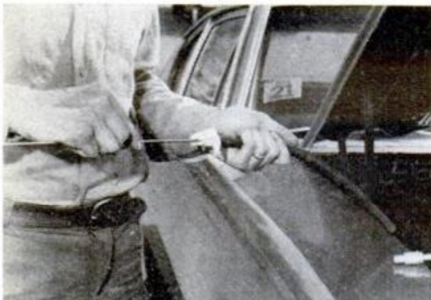
VENTILATOR HOSE of your emission system can be cleaned on the inside using a rod and piece of cloth
