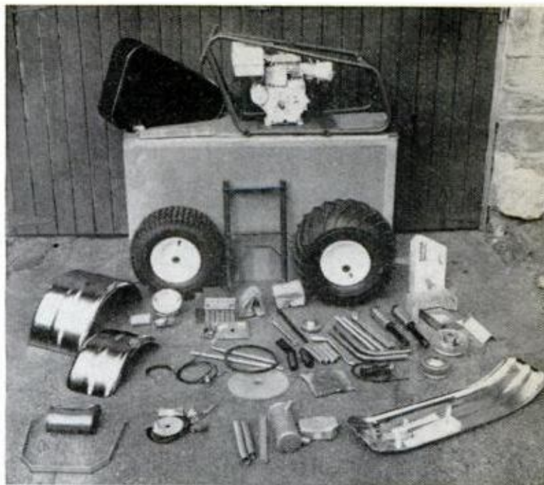
SHIPPING CARTON becomes a handy workstand for making adjustments on partly assembled Heald bike above. At right is kit of parts prior to assembly. Snow ski, lights and special spark-arresting muffler are accessory items. The Super Bronc, with a 7-hp engine, is most powerful of three kit bikes tested
