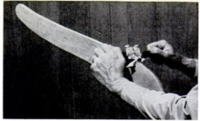
RIPPLES made by bandsaw blade can be smoothed out with spokeshave as shown or plane and sander
