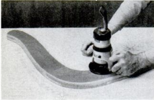
ROUTER with \frac{1}{4} -round bit will cut round edges on side panels. Don't shape where armrest meets panel
