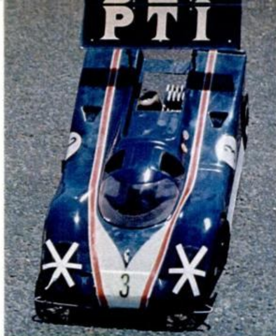
HEATHKIT'S SPECTRE R/C car body ($46.95) includes coil spring suspension and 5.5:1 gear ratio. The engine and radio-control unit must be purchased separately. Model (right) is a Can Am (Group 7) racer
