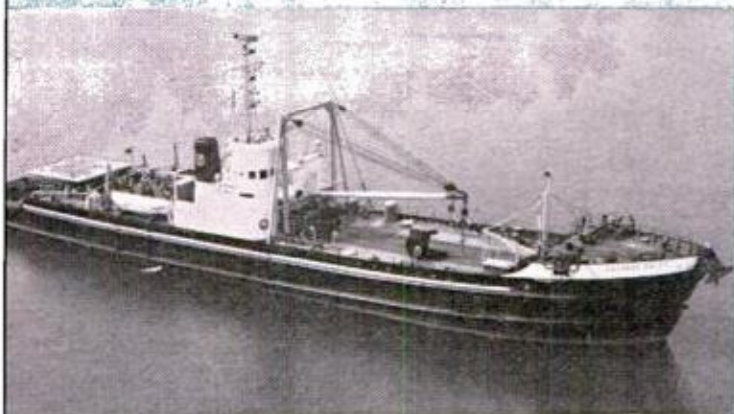
POWERED BY TWIN 1800-hp diesels, the Salvage Chief , a 192-foot converted LSM, is all "muscle"
