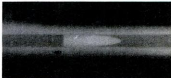
Traveling down the barrel. The next X ray shows the bullet moving down the barrel at approximately 1900 feet per second. By relating the position of the bullet to a chamber pressure and time, Remington engineers get a better understanding of the dynamics of the firing cycle. This type of research leads to more uniform performance by the combination of primer, propellant and bullet—and hence better accuracy for the hunter.
