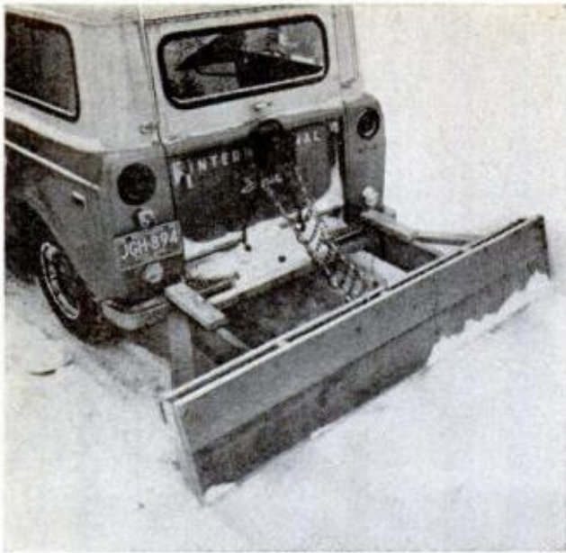
PLOW is attached to the vehicle by chains wrapped around bumper, then hooked over projecting nailhead
