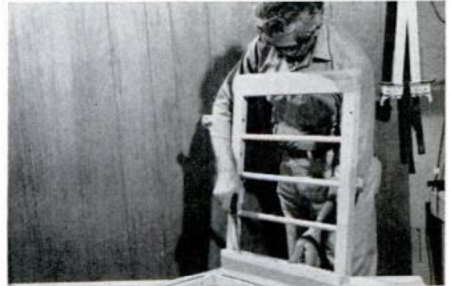
BACK is joined to bottom frame with screws, glue. Using damp cloth, wipe off excess glue before it sets
