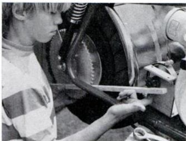
LIKE OTHER BIKES , Heald model has an adjustable jackshaft, here being checked for proper alignment with large drive-chain sprocket on the rear wheel
