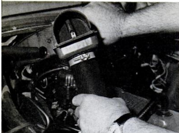
DAMPER VALVE is closed when engine is cold; air for combustion is picked up at hot exhaust manifold
