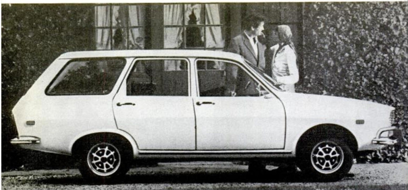
RENAULT 12 STATION WAGON has top-hinged tailgate and 58 cu. ft. of cargo space with rear seat folded. In profile, wedge shape is approached by downward slope of hood and high degree of rake of windshield
