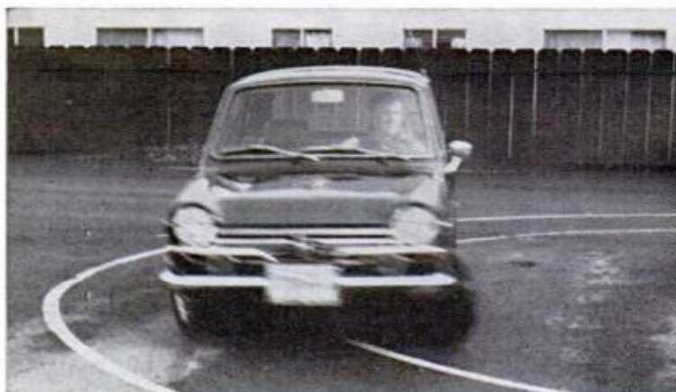
FRONT-WHEEL DRIVE , quick rack-and-pinion steering put Honda's handling on par with some sports cars 96
