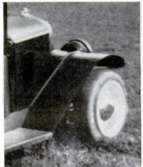
TOURING-CAR TOP of fiberglass fits over a frame of electrical conduit. Side curtains, with sliding plexiglass windows, keep out weather. Fenders were shaped from 55-gallon oil drums
