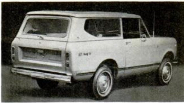
SCOUT II stands lower, longer; gets re-engineered suspension for a greater on or off-highway comfort
