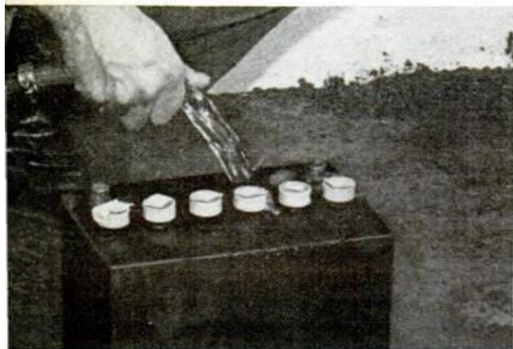
FLUSH BATTERY with clear water; make sure that your cleaning solution is thoroughly washed away
