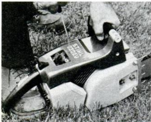
FOR SAFE STARTING hold handle at balance, put right foot in rear handle before pulling the cord
