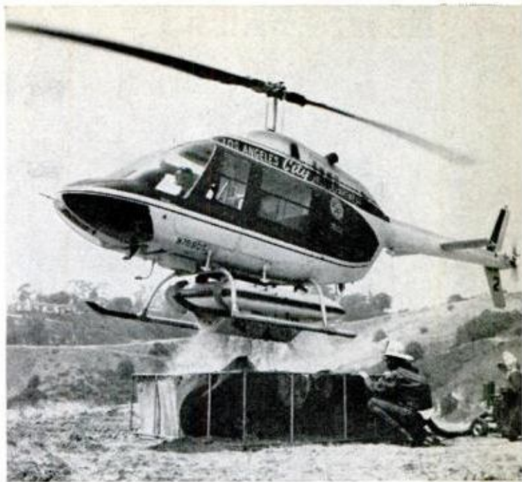
FLYING FIRE ENGINES with belly tanks water-bomb brush fires on remote Los Angeles mountain peaks
