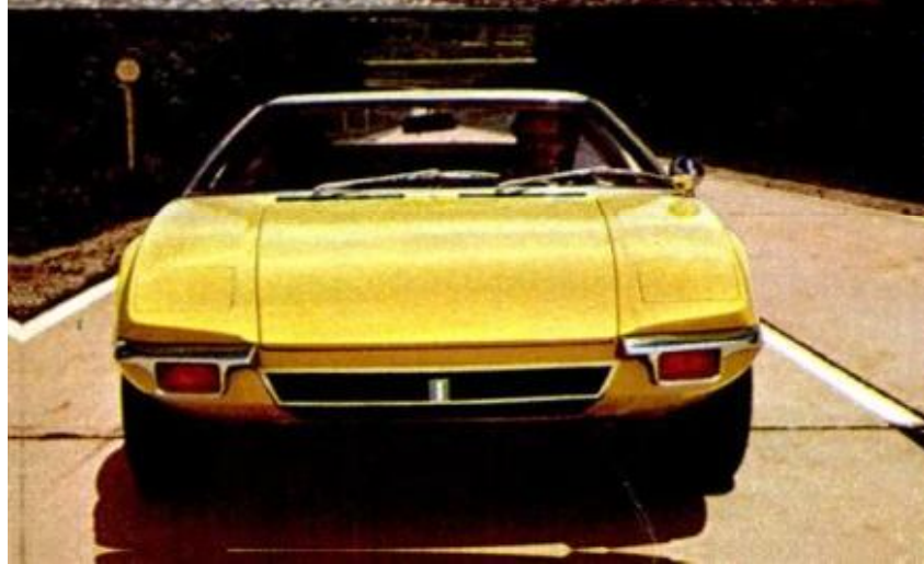
DE TOMASO PANTERA, a low, sleek, two-seater, mid-engine sports car, is distributed by Lincoln-Mercury. Built by deTomaso Automobili in Italy, the Pantera (Italian for Panther) is powered by Ford's 351-cu.-in., four-barrel V8. The powerful domestic engine combined with styling and coachwork executed by Ghia Studios in Italy, result in an exotic sports car that's easily serviced
