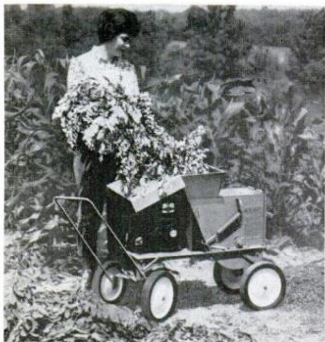
UNIFORM MULCH is produced by the Kemp Suburbanite Shredder through its rotation of 42 steel teeth at 3400 rpm by a 3-hp Briggs & Stratton gasoline engine or 1-hp electric motor. Price is about $250
