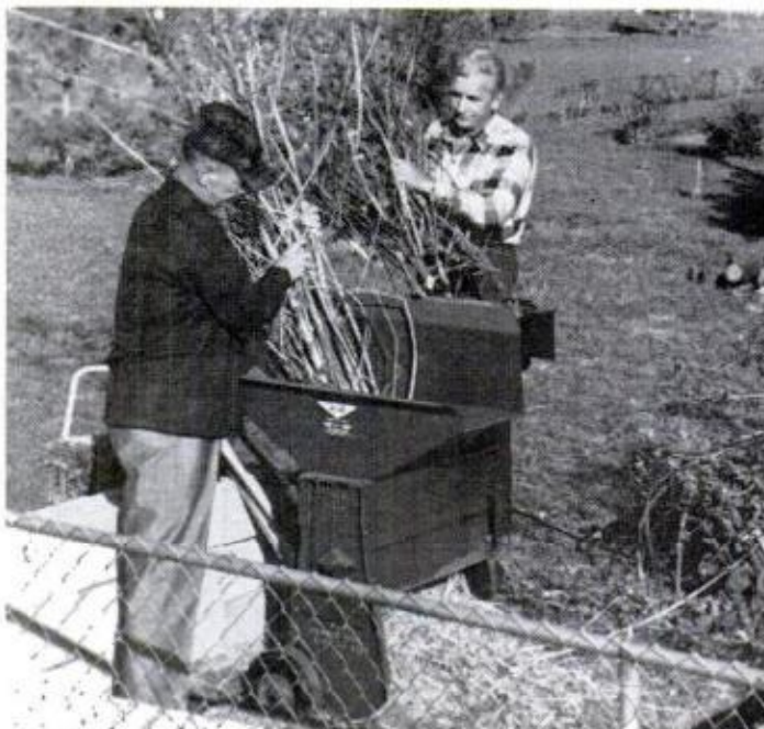
LIGHT BRUSH is also handled by W-W's Model 66-G. Twenty-four curved hammers, rotating at 2500 rpm, flail garden waste. Powered by a 7-hp, electric-start gasoline engine or a 1-hp motor, it costs about $260
