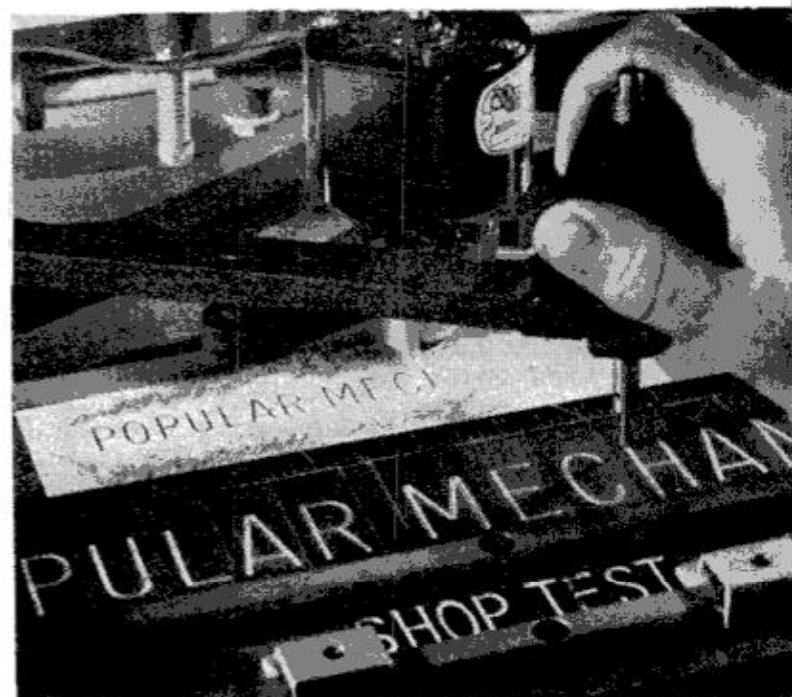
LITTLE MECHANICAL KNOW-HOW is said to be needed when using this machine to make engraved signs
