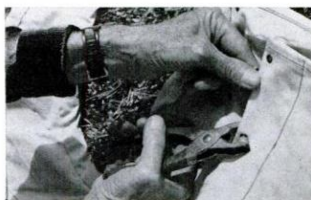
SPACE GROMMETS EVENLY to obtain the maximum strength from nylon or other long-lasting lacing
