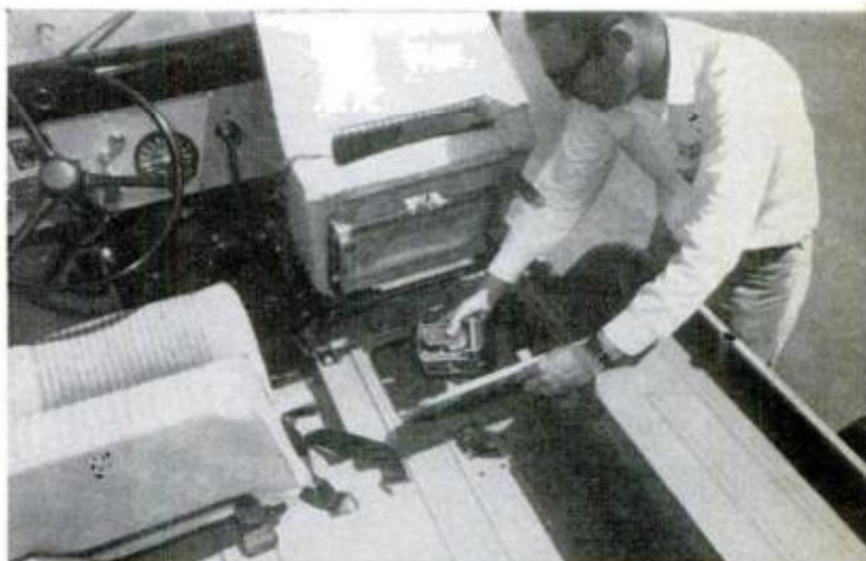
LOCKABLE STORAGE BIN under the passenger's seat hold valuables. Firm, comfortable buckets place occupants above most cars. Jeep's ride is bouncy
