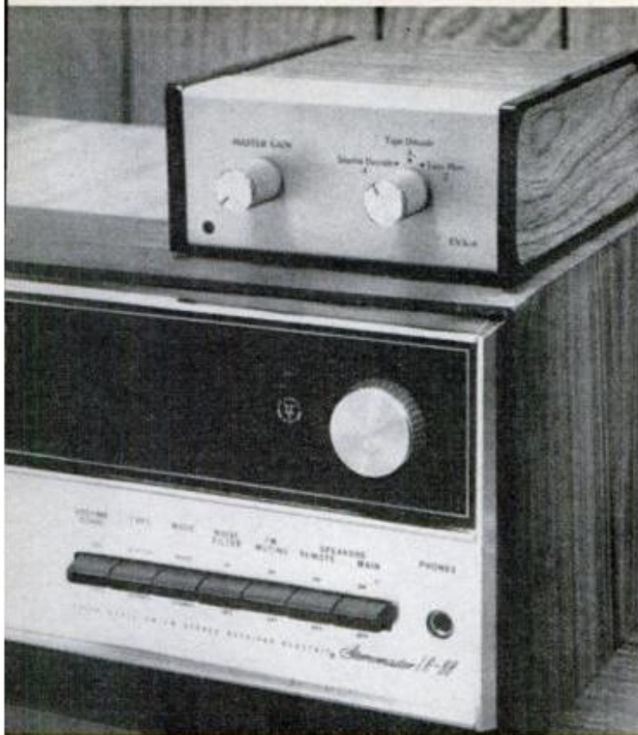
SMALL ELECTRO-VOICE DECODER , shown on top of receiver above, provides four-channel output from two- or four-channel sources, is priced at $59.95. Diagram on facing page shows hookup requiring second stereo amplifier as well as existing one. Photo below shows various connections on back of decoder
