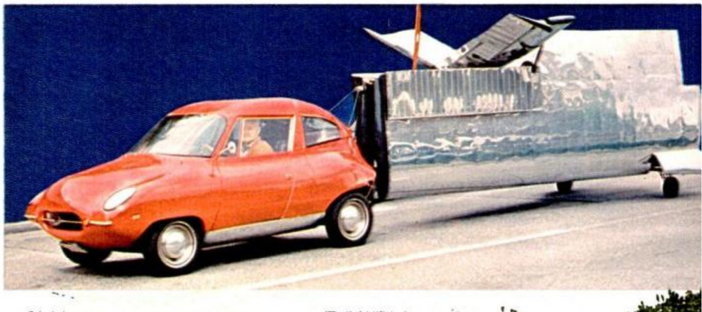
THE FLYING AUTOMOBILE attracts startled glances in downtown traffic. It handles easily even when towing the flight trailer. A special pylon is said to keep the trailer steady up to 70 mph and in 40-mph crosswinds
