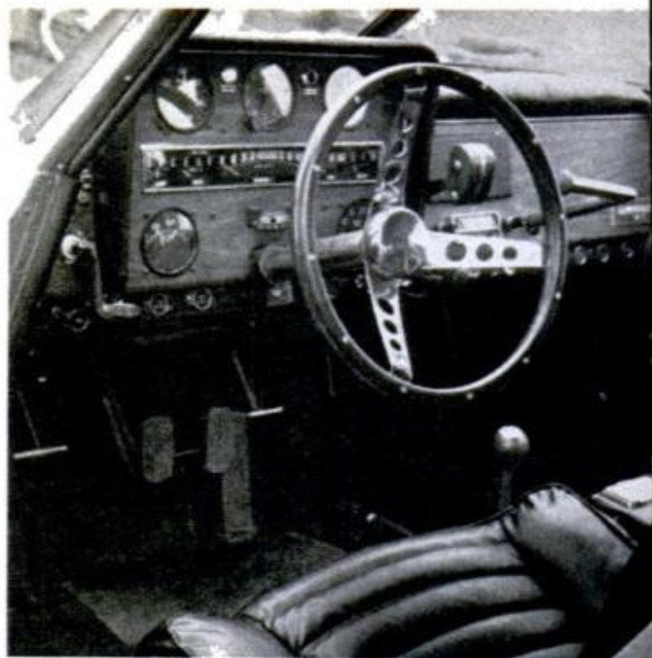
HANDSOME DASH holds car and plane instruments. Rudder pedals are outboard of clutch, accelerator
