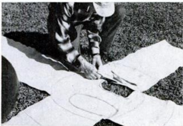
CUT OUT MARKED AREA NEATLY , being sure to go through both pieces of the overlapping canvas
