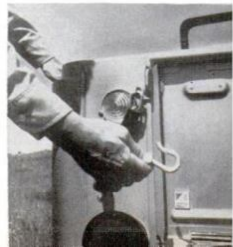
BASIC CJ JEEP has no doors to rattle, yet tailgate does; un-insulated body amplifies sound
