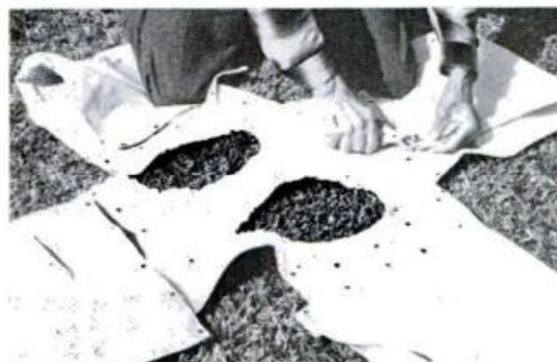
LACE INNER TUBE IN CANVAS and your instant boat is done. Try variations on this basic design
