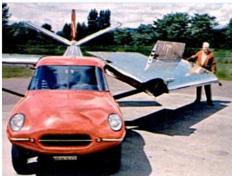
BUG BECOMES BIRD as two pins are driven in place to secure flight component and wings unfold for takeoff
