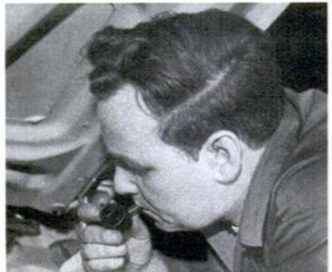
VACUUM CHECK VALVE is easy to test: Blow into it and then draw out through it. (See text for details)
