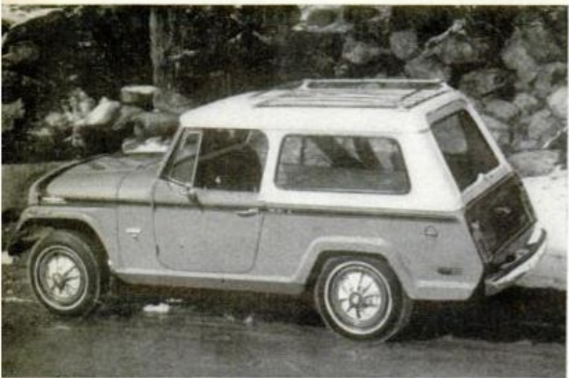
JEEPSTER COMMANDO has same ruggedness and 4wd as Universal, can be made as wagon, roadster or pickup; uses same F-head 4 or V6 as regular Jeep
