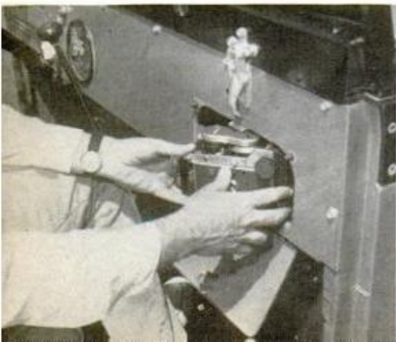
GLOVEBOX has more room than most, also has lock. Hasp above it secures the folding windshield
