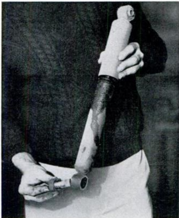
DOUBLE TROUBLE with this shock includes ruptured seals and well-worn bushing that caused "clunking"
