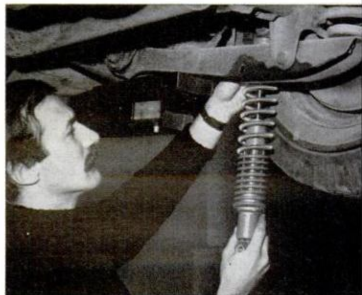
LOTS OF LEVERAGE may be needed getting off old shocks (left). New replacement (right) for rear shock of this station wagon is heavy-duty stabilizer type intended for carrying heavy loads and for safer towing
