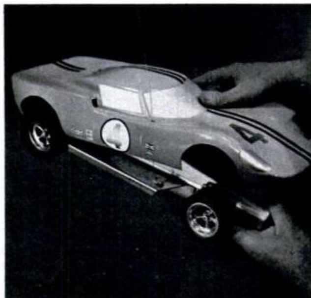
PLASTIC BODY quickly snaps on and off chassis with no other fastening. This enables you to get inside easily to start the engine and make adjustments
