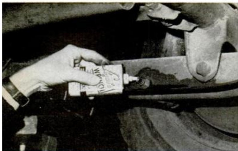
REAR SHOCK is secured at bottom end to the axle-carrying control arm. Use "nut-buster" if necessary
