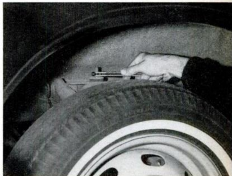
TOP END of front shock absorber on this car can be reached in wheel well without removing the wheel
