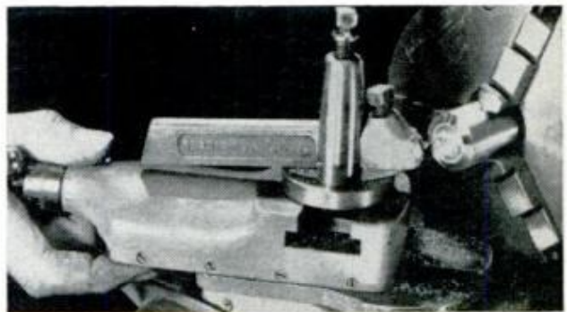
TO GENERATE CONCAVE CHAMFER on 1-in. brass rod, swinging compound slide is brought into play
