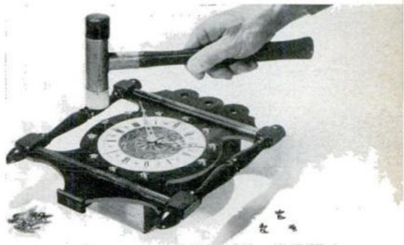
STARS AROUND DIAL are lightly tapped into pre-drilled holes located on 6½-in.-dia. penciled circle
