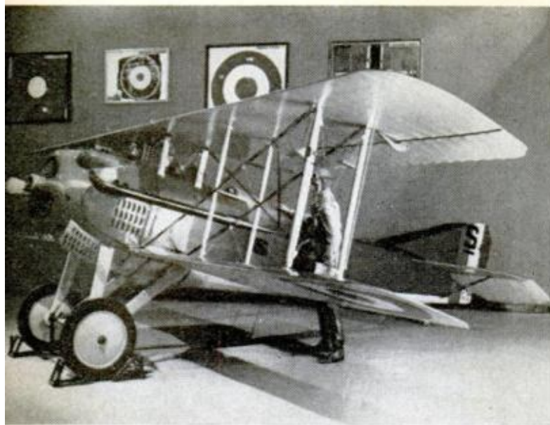
S.P.A.D. VII was one of the best of World War I. With U.S. designs lagging, pilots like Rickenbacker flew it. Its gun was synchronized, it did 130 mph, climbed to 22,000 and stayed together in dives
