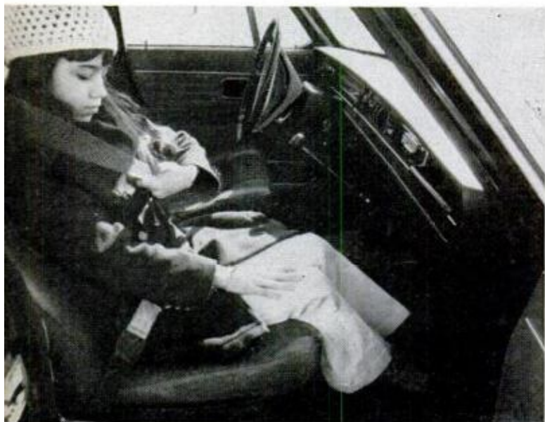
ADULT SHOULDER BELT and combination lap belt (always wear both; never the shoulder belt without the lap belt) cannot be worn by children until they reach a height of about 55 inches. Seven-year old (above) is 47 inches tall and too small. Girl 12 years old and 59 inches (below) checks strap for tightness
