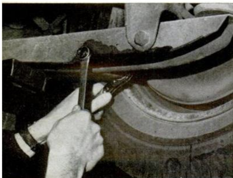
LOTS OF LEVERAGE may be needed getting off old shocks (left). New replacement (right) for rear shock of this station wagon is heavy-duty stabilizer type intended for carrying heavy loads and for safer towing
