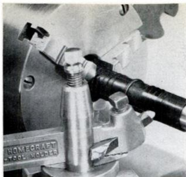
PLASTIC COUPLING of type used to join flexible plastic pipe is softer than PVC, but still machinable
