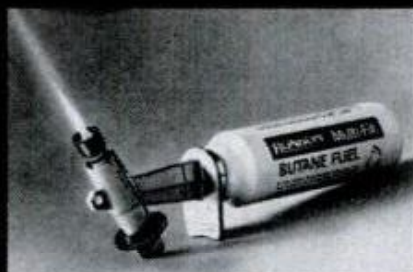
STANDS ITSELF: Place torch on flat working surface. Tripod formed by torch head and Multi-Fill provides firm three-point stand, leaving both hands free for holding, bending and turning operations.
