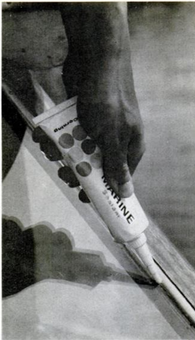
SILICONE RUBBER SEALANT is often used to seal windshield joints because it adheres so well to glass
