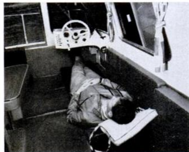
INSTRUMENT PANEL and steering wheel are adequately mounted for most people, though as usual, author had some difficulty with his 6-foot-3 frame. Skipper's seat (right) folds down to make the boat's seventh bed
