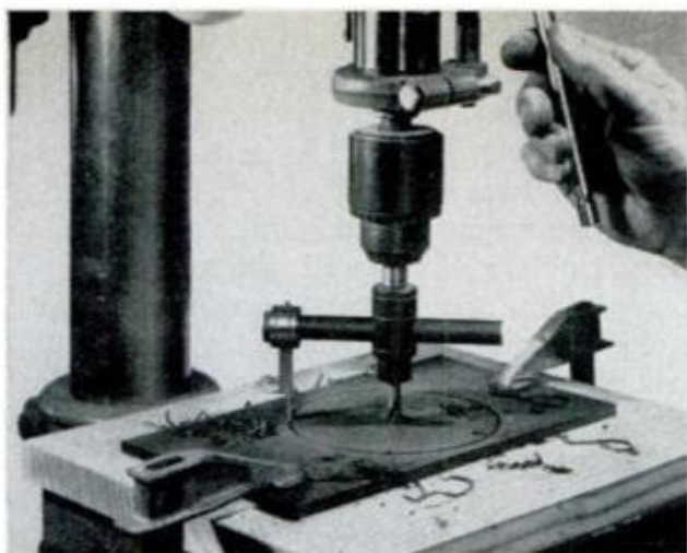
CUT CAM BLANKS from tempered hardboard with a circle cutter in drill press. To play safe, clamp work
