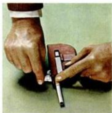
6. Hold the paper tube. Push the lever. Pull the lever back, let go of the tube, push again. The cigarette will fall free of the machine.
