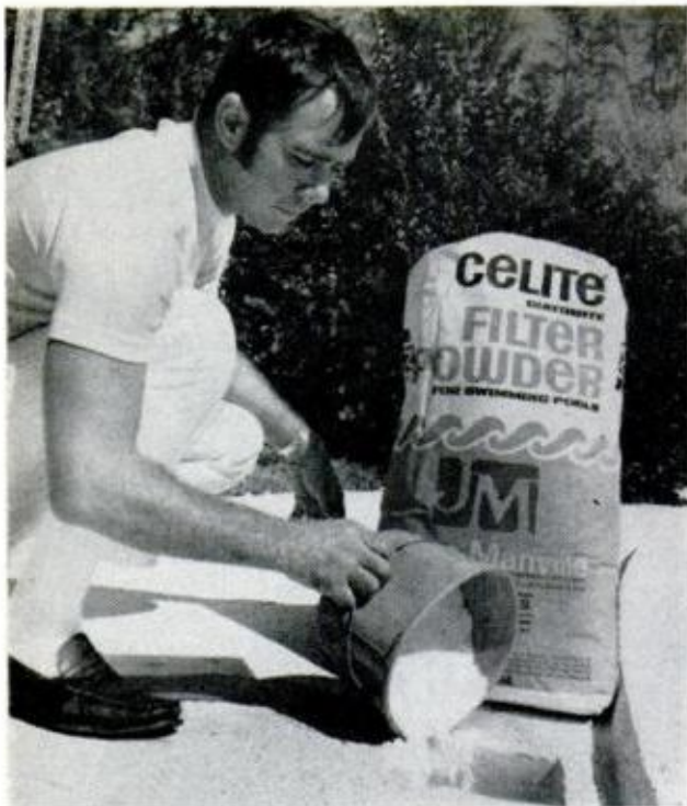
FILTRATION IS IMPORTANT in preparing your pool for the season. Here, a powdered filter aid is added
