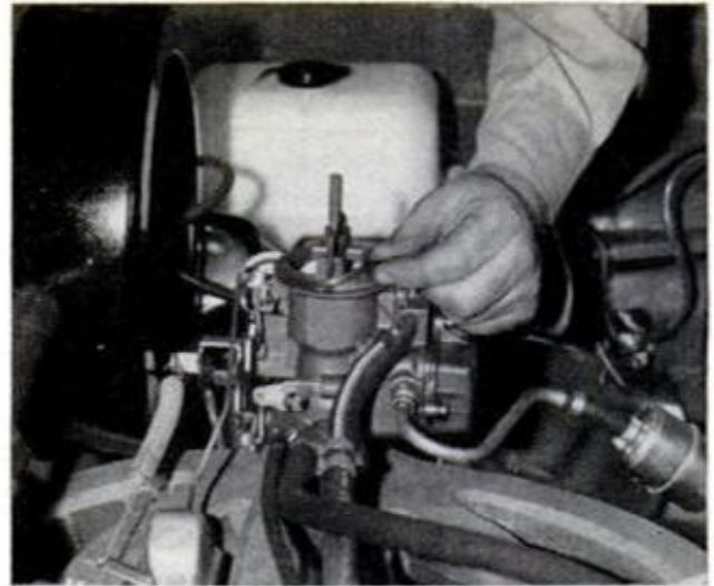
CHECK GASKET under the air filter on the air horn. Replace it if it is in less than perfect condition
