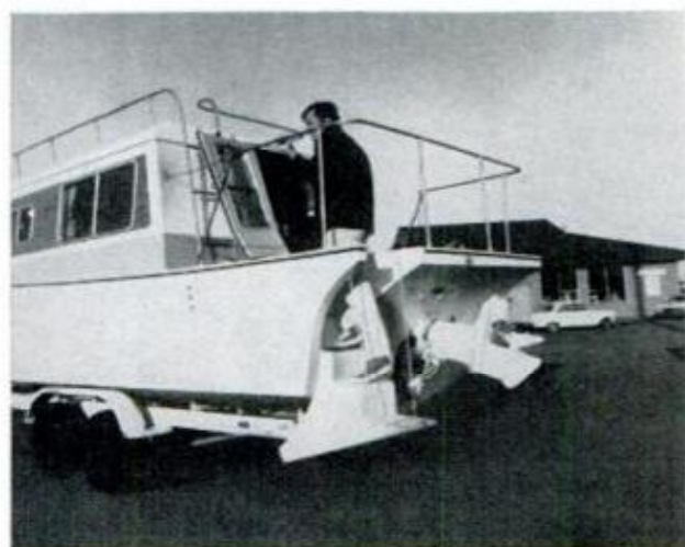
FOLDWAY STEPS prove designers' intention to see this boat used as a genuine camping vehicle ashore JUNE 1971
