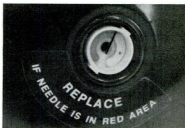
SOME TYPES have an indicator located at top of cylinder to show when the pressure is inadequate
