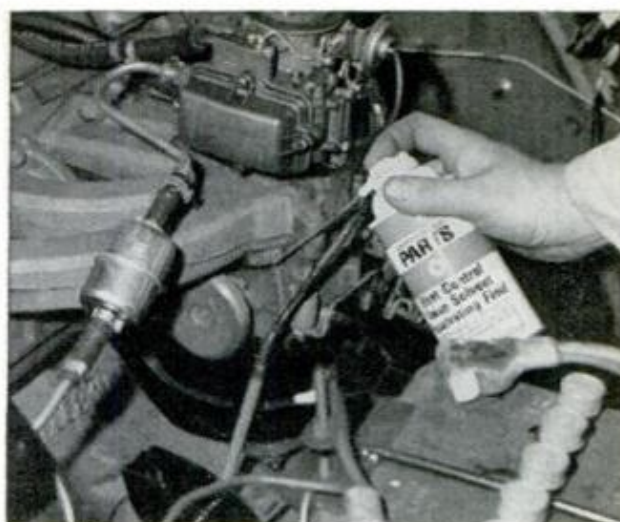
MANIFOLD HEAT-CONTROL VALVE , often neglected, must move freely. If stuck, use solvent to free it
