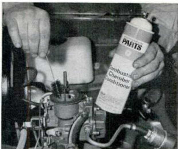
VENTURI WALLS accumulate deposits that affect fuel consumption. Clean them until smooth, shiny again
