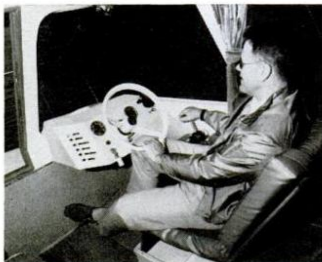
INSTRUMENT PANEL and steering wheel are adequately mounted for most people, though as usual, author had some difficulty with his 6-foot-3 frame. Skipper's seat (right) folds down to make the boat's seventh bed
