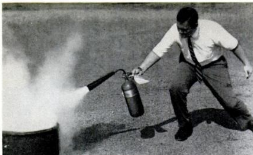
CARBON DIOXIDE is used in B-C extinguishers. This type requires that you get close to the fire and direct spray at base of the flame
