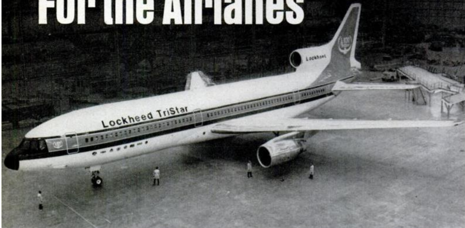
LOCKHEED'S L-1011 TRISTAR is a wide-body jetliner powered by three Rolls-Royce turbofan engines
