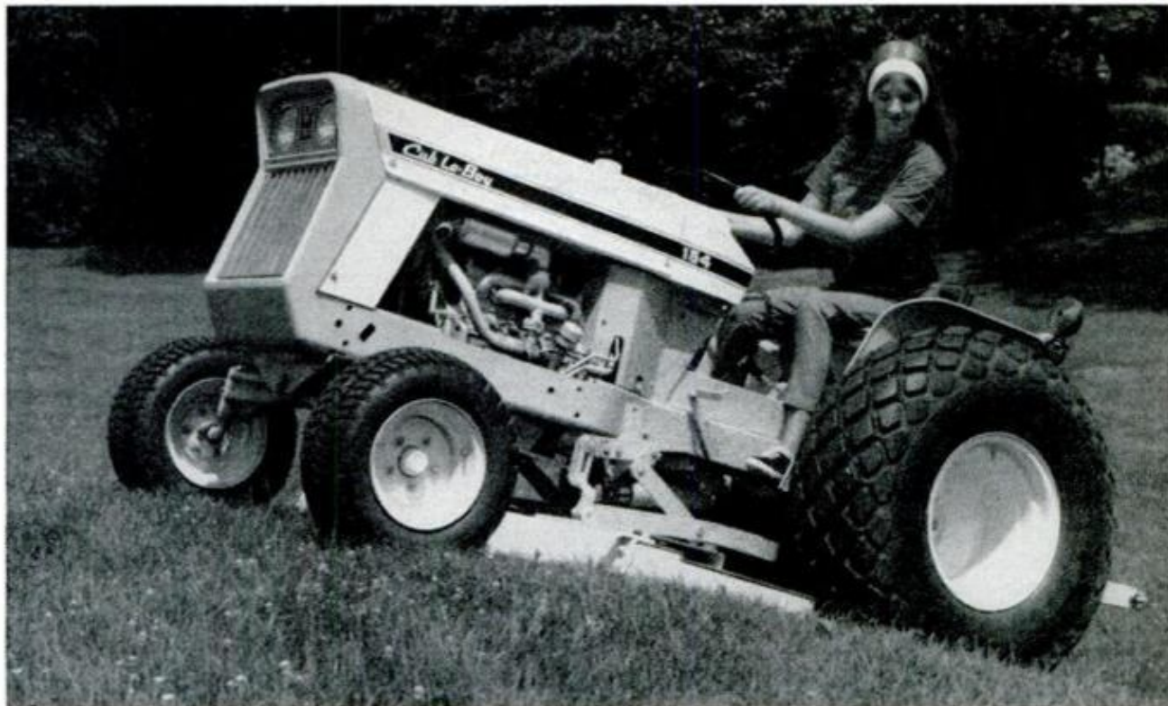
INTERNATIONAL 154 CUB LO-BOY has four-cylinder water-cooled engine of 15 hp. It weighs 1350 lbs.
