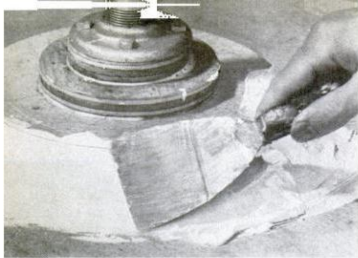
FIRST STEP in molding gracefully curved pedestal is to fill in "steps" using plaster of paris
