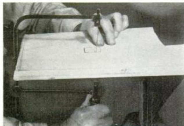
OPENING can be cut in the center of a large piece of work by first drilling pilot holes at four corners
