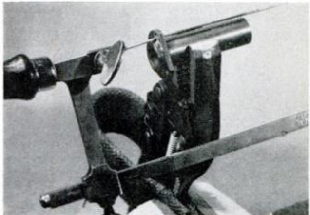
COPPER WIRE installed in frame can be used as lap for smoothing, increases clearance in small grooves
