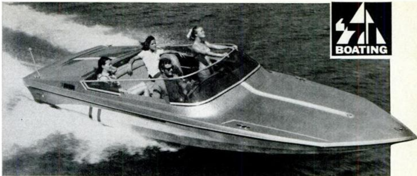
GLASTRON/CARLSON'S NEW CV-21 powered with 350-cu.-in., 265-hp jet engine moves at more than 50 mph
