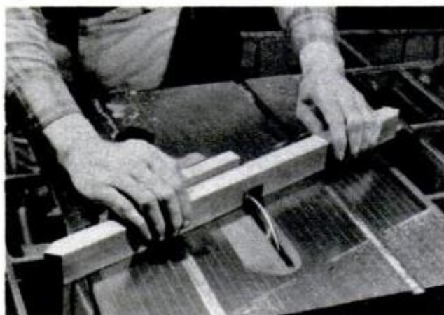
PLASTIC INSERTS are labeled for reassembly identity. GE Silicone Seal keeps the pieces from shifting
