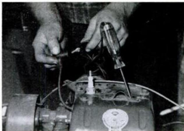
BREAKERLESS IGNITION SYSTEM must be tested with a spark intensity tester connected to the plug lead
