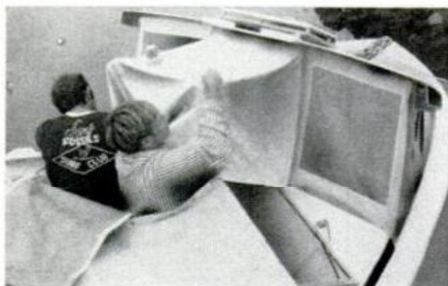
"CORRIDOR CANOPY" snaps around mast light to provide weatherproof passage from cabin to cockpit
