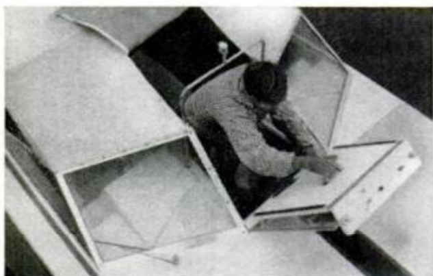
FIRST STEPS in "popping" camper top for the night are to unhook hatch and ease it over onto foredeck
