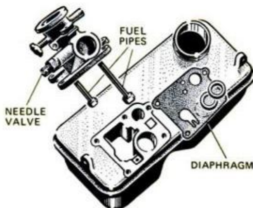
DIAPHRAGM-TYPE CARBURETOR is directly coupled to the fuel tank. When fuel stoppage seems to be the cause of trouble, check screens in the fuel pipes
