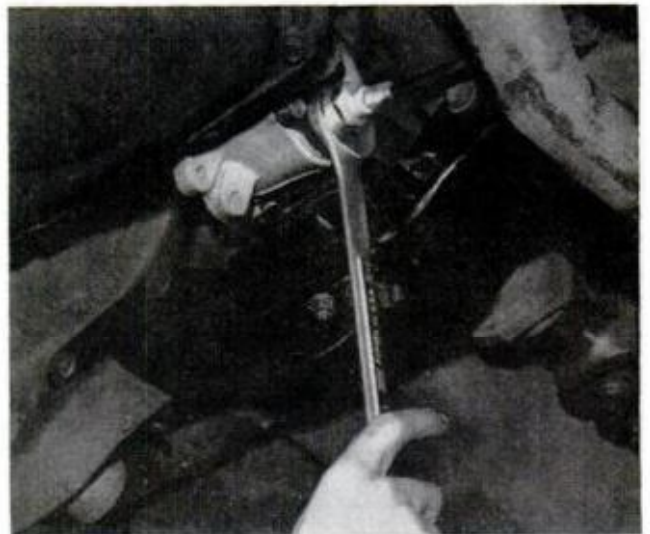
TO REMOVE SNAPPED CABLE you must detach cable housing from the pinion gear at the transmission
