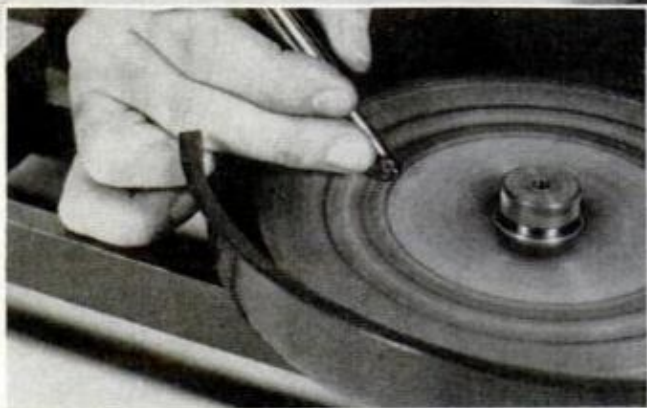
LAP PLATE can be of copper, tin or plastic, depending on faceting step. Pie tin acts as splash guard
