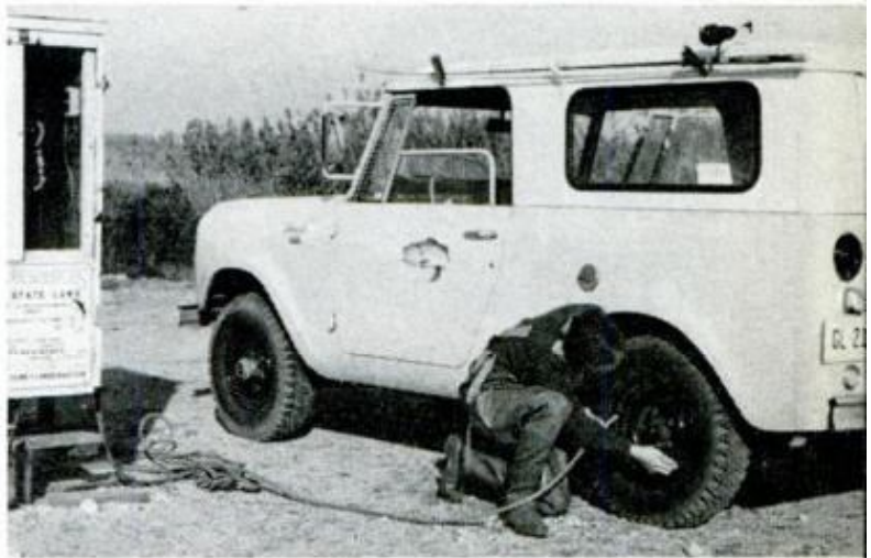
SOON AFTER LEAVING BEACH, reinflate your tires to save unnecessary wear driving over paved roads
