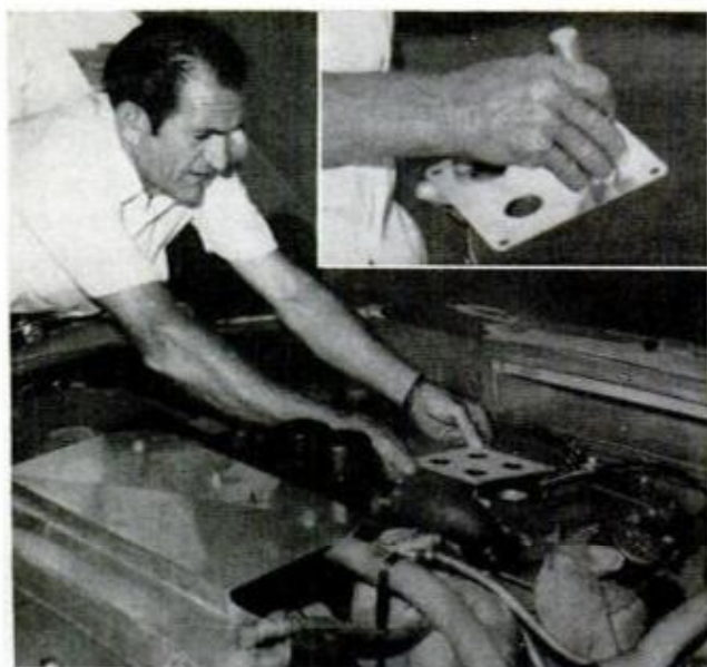
CARBURETOR PLATE must be installed on 426 Hemis, 429 Fords. The 1¼-in. venturi, being checked with go/no-go gauge, restricts fuel/air flow to cylinders
