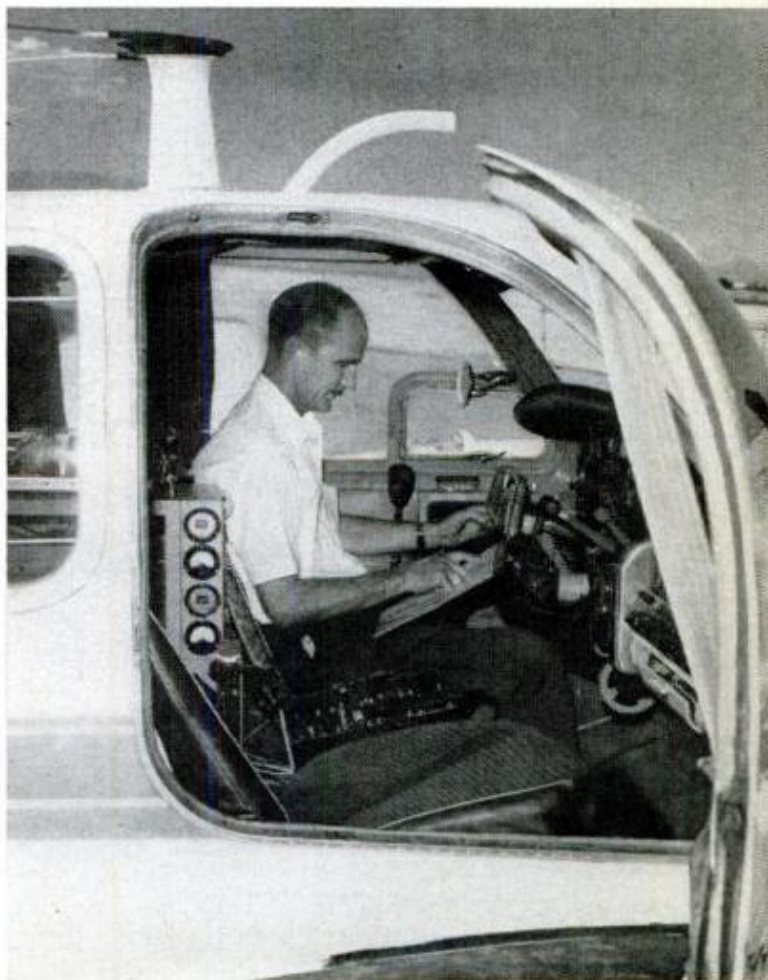
BATTERY OF SENSITIVE DETECTORS on plane can pinpoint radioactive sources hundreds of feet below
