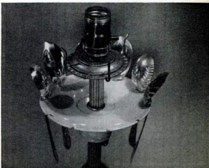
HOLDER is sandwiched between glass knob and tubing. Socket is then tightened to hold it firmly in place
