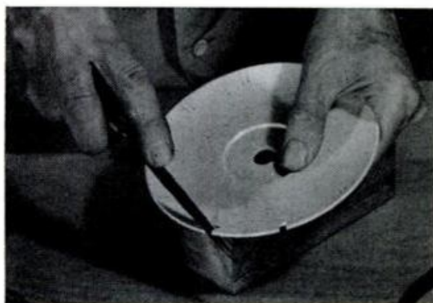
SPOON HANDLE NOTCHES are roughed out with drill and saw. A file is used to shape and smooth the cuts
