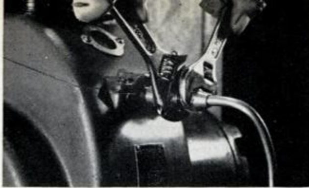
DON'T OVERTIGHTEN flare fittings or you'll strip the threads. If joint leaks, inspect tube's flare
