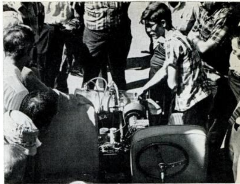
STEAM GENERATOR or boiler operation is explained to crowd by Philip Barrett (above), who with his father built the steam car on an old Triumph chassis. Condenser that converts supersaturated steam back to water is mounted on front end of car (below)
