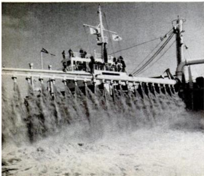
SHELL'S SAND-SINK METHOD is run through test (below) off the Netherlands coast. Sand treated to attract oil is sprayed on slick. As they sink, the sand particles carry oil with them to bottom
