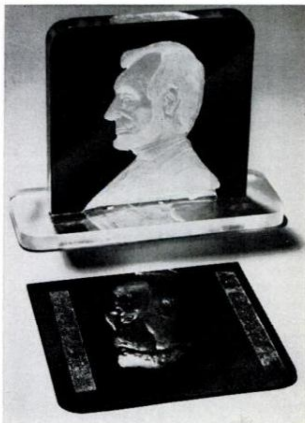
BACK VIEW of carving shows varying depths of cut. When the carving is finished, a colored sheet plastic (right) is affixed to it by means of double-faced tape. If preferred, the carving can be painted
