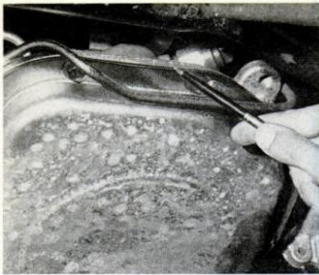
TRANSMISSION MODEL NUMBER , found on casing, may be necessary to tell if car can be push started
