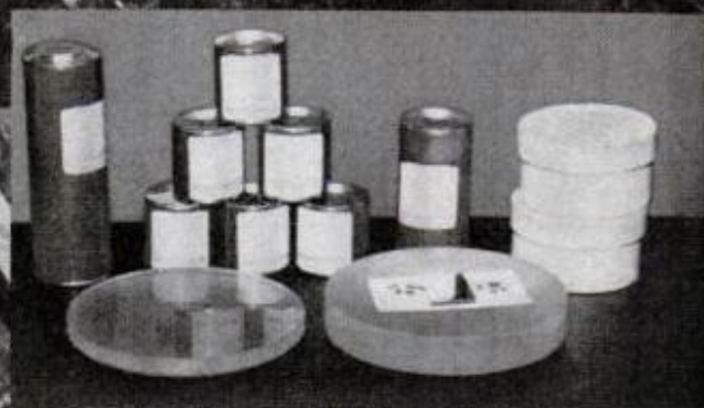
MIRROR-MAKING KIT consists of two glass discs, a diagonal mirror, two eyepiece lenses, seven grades (called grits) of grinding compound, rouge and pitch
