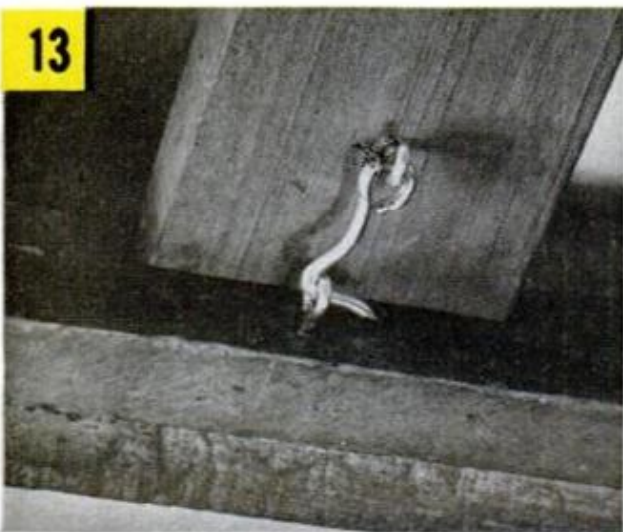
13 SPRING-SUPPORTING BED SLATS will be prevented from falling out if you drive eyescrews into the ledger strips along the bed rails as shown. Then, simply fasten a hook to the ends of each slat to secure
