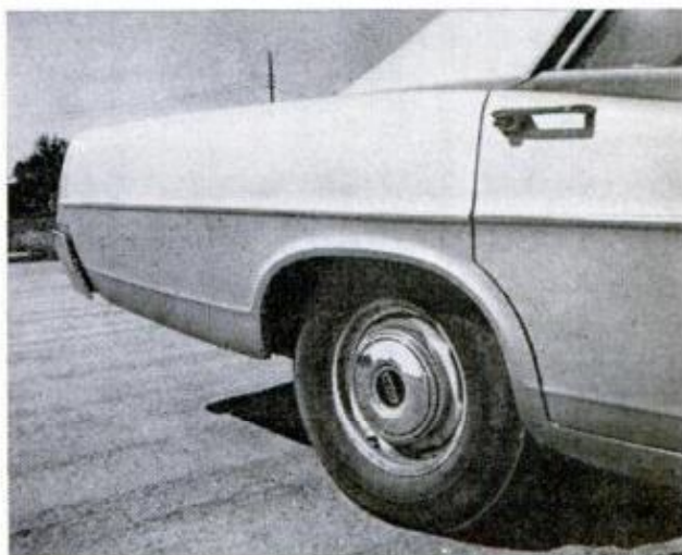
FINISHED JOB after sanding, painting and new molding looks like new. Whole job was done by one man
