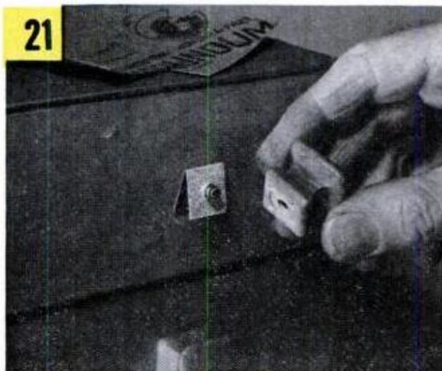
21 A SANDPAPER "WASHER," if cut and installed on the knob-holding screw as shown, can be used to hold the loosest wood knob securely in place. When knob is tightened, abrasive grabs and holds it fast
