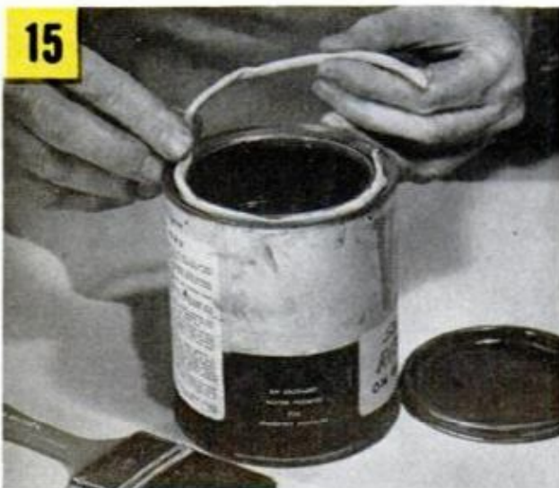
15 KEEP PAINT-CAN RIM free of paint slop that occurs whenever a brush is wiped across the rim by filling it with a bead of weatherstrip. When the strip is removed, the cover will again seat as it should
