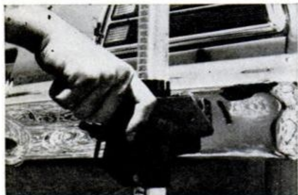
JACK HEAD fits in slot in Firebird's rear bumper, with similar slot up front. These help steady jack
