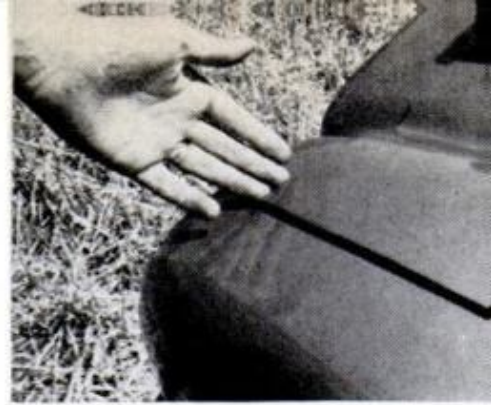
FIBERGLASS hood on Formula 400 fits poorly, has fake scoops
