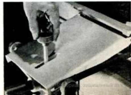
TO ADJUST FENCE crosswise, loosen knob and push guard along guide rod
