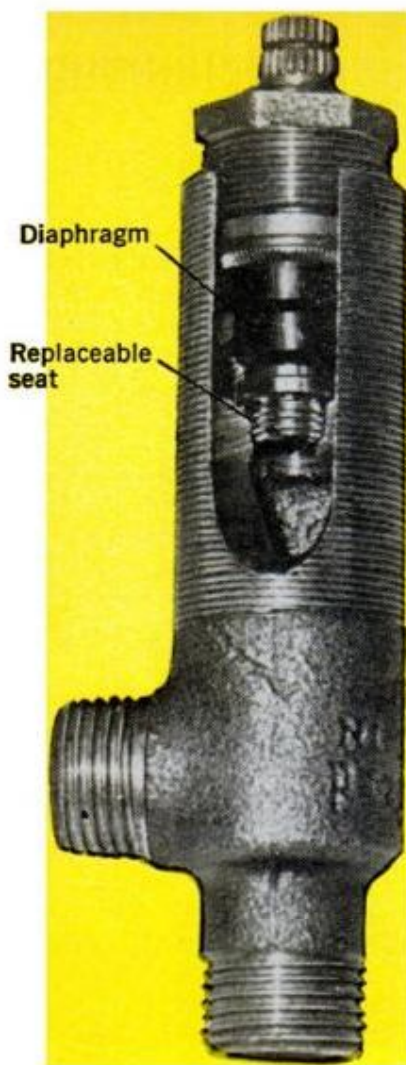
WASHERLESS FAUCET (above) eliminates seat washer and O-rings. Brim of diaphragm fits barrel, prevents spout leaks
