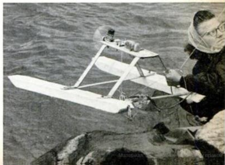
TWO FISHING LINES can be hooked up to the little airboat and taken out to midstream or up to the foot of the dam. Once the boat's on target, a sharp jerk on connecting line shuts off fuel supply to model-airplane motor and drops lines to bottom. Boat is then reeled in, clear of fishing area. Below: A wife waits for a launch signal from her husband
