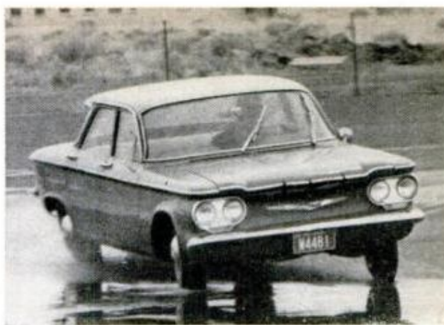
CORVAIR is one car at the school. Car is set up to understeer turning right, oversteer turning left
