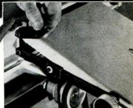
PIVOTING FINGER drops against positive stop to return fence to 90° position
