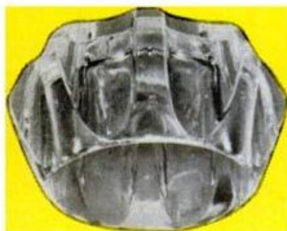
WASHERLESS FAUCET (above) eliminates seat washer and O-rings. Brim of diaphragm fits barrel, prevents spout leaks
