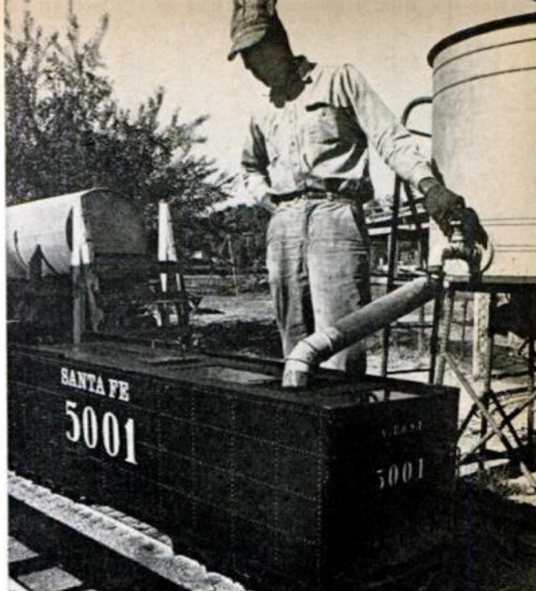
WATER TANK , like everything on the road, is built to scale. Tender holds 40 gallons of water
