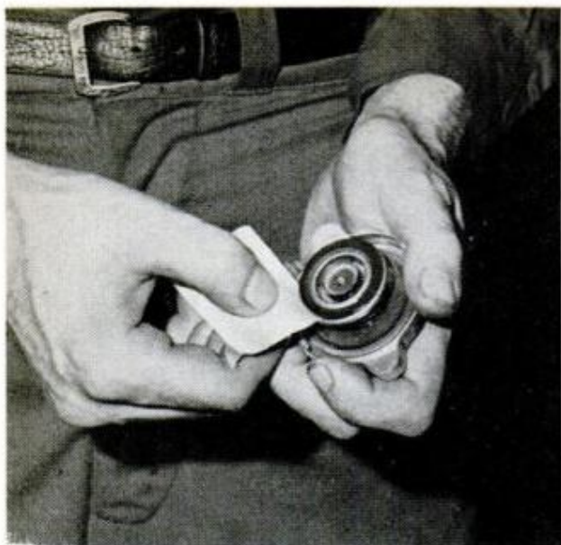
RUBBER SEAL on radiator cap should be inspected, and any dirt under it cleaned out with clean paper
