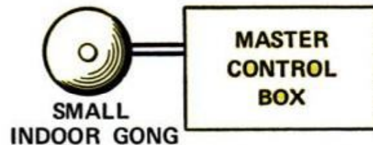
MASTER CONTROL BOX can be hidden in closet, pantry or utility room. Powered by two 12-volt batteries, it has a test switch for making checks on system. Next to it is a small indoor fire gong
