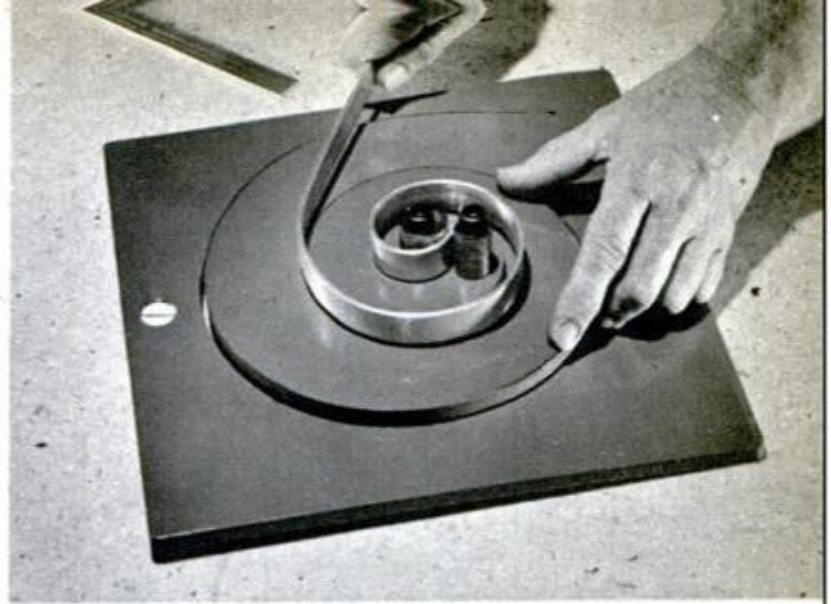
HEAVY-DUTY BENCH SCROLLER forms decorative scrolls quickly. Each scroll requires a 28½-in. metal strip
