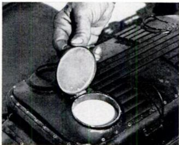
SAND BINS are duplicates of the real thing. Sand is dropped in front of drive wheels when starting
