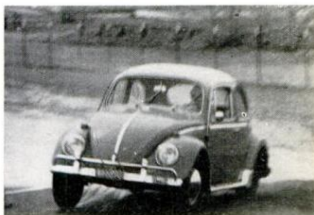
VOLKSWAGEN oversteers and reacts very quickly. All cars run on bald tires, pavement is wetted down
