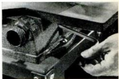
POINTER-FITTED LEVER sets depth of cut; maximum is 3/8 in. Knob locks setting.
