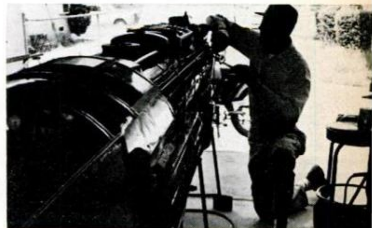
REPAIR WORK is done in garage shop where Mann made all parts on lathe from new and scrap stock
