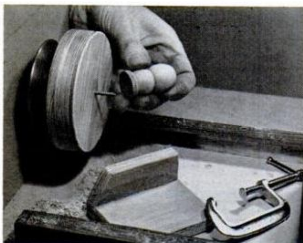
CENTER SCREW through the faceplate held this knob for turning. Auxiliary rest in the foreground was used
