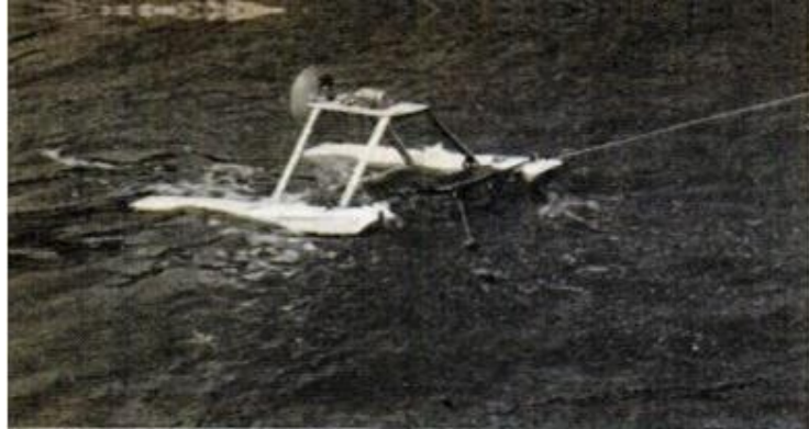
CATAMARAN DESIGN enables boat to ride well over rough water, carry considerable weight behind motor
