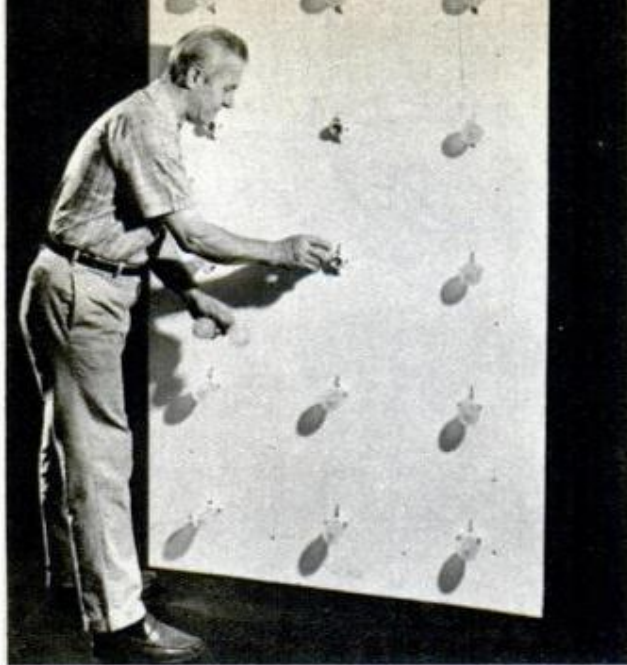
PONY-TYPE SOCKETS , bolted to back panel and wired from rear, are fitted with 25-watt incandescent lamps
