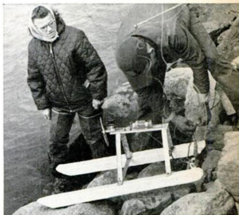
TWO FISHING LINES can be hooked up to the little airboat and taken out to midstream or up to the foot of the dam. Once the boat's on target, a sharp jerk on connecting line shuts off fuel supply to model-airplane motor and drops lines to bottom. Boat is then reeled in, clear of fishing area. Below: A wife waits for a launch signal from her husband
