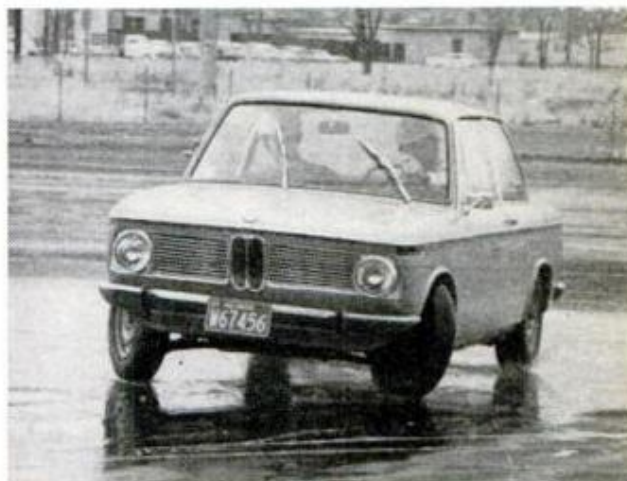
BMW 1600 has basically neutral steering characteristics, but weight is added in trunk to change that
