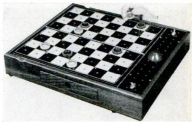
EACH CHECKER IS A SWITCH which sets off a horn on making contact with metal plate in hidden board
