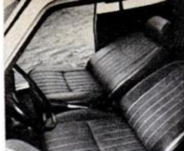
ROOMY TRUNK ACTUALLY HOLDS TWO SUITCASES. Datsun gets 69 hp out of high-revving, short-stroke OHC 4. Front bucket seats adjust to a reclining position; rear seats fold down for extra luggage space
