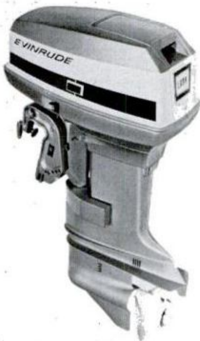
BRITISH SEAGULL 6-hp Silver Century Plus (top) and Evinrude 50-hp loop-charged Lark with tuned exhaust
