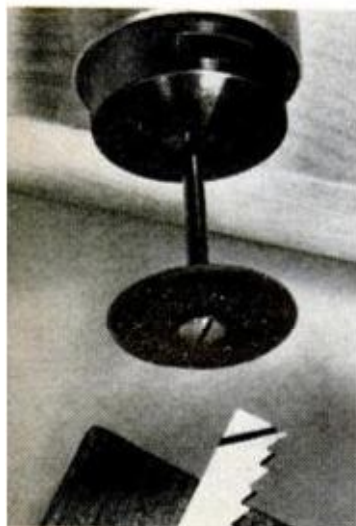
100 TEMPLATES AT ONE SHOT can be cut through pad with a chisel blade in the standard Stanley saw
