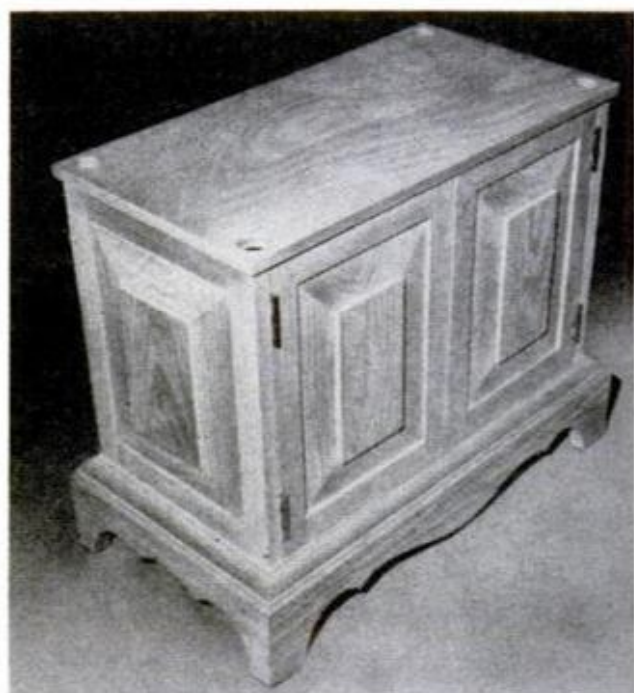
COMPLETED CABINET BASE is shown with scroll-cut bottom attached. Use brass butts to hinge the doors
