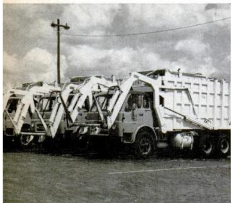
LPG FUEL TANK is visible under one of the trucks in this fleet, one of many fleets converted to LPG
