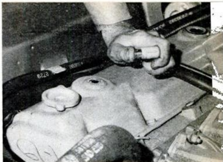
PCV VALVE in positive crankcase ventilation system is hard to clean and it must be replaced periodically
