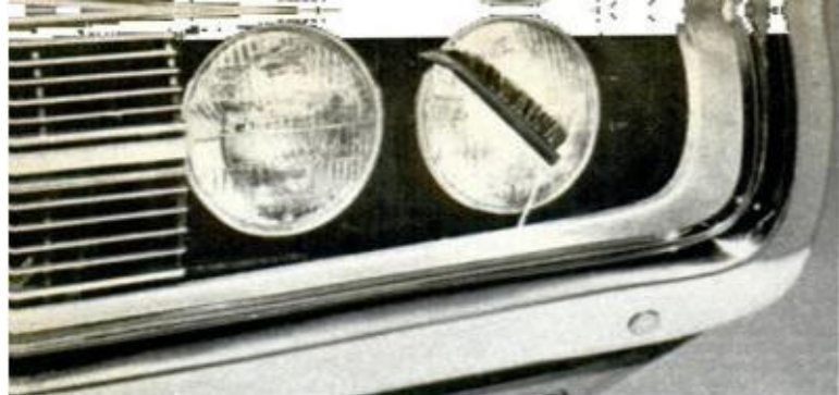
HEADLAMP WASHER SYSTEM includes nylon brushes, solenoid, actuators and washer reservoir with pump
