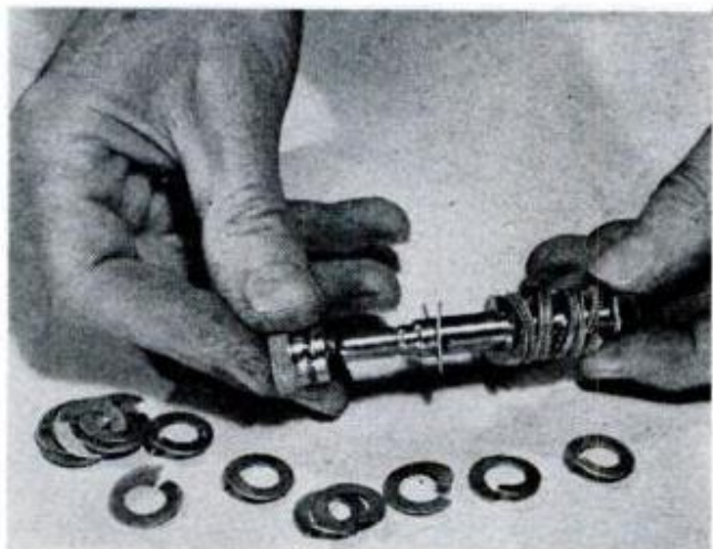
STORING WASHERS is one of many uses for push-pull nut; it's handy way to carry them in toolbox
