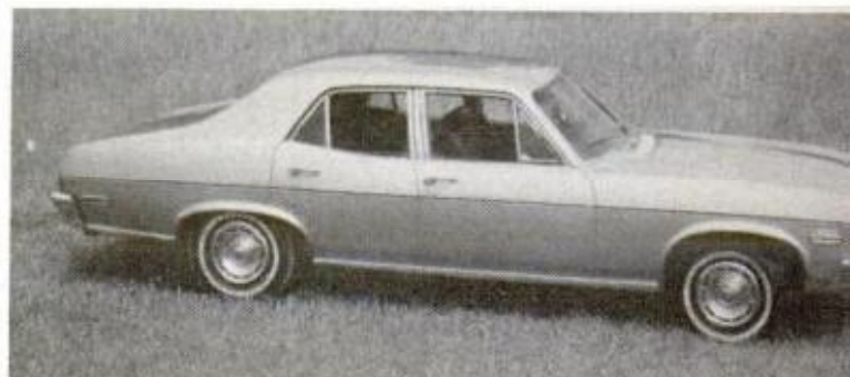
CHEVY NOVA new base engine is 145-hp, 250 c.i.d. Six
