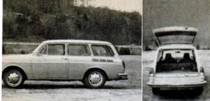
VOLKSWAGEN SQUAREBACK is only wagon with front trunk. Louvers help cool engine under floor in rear
