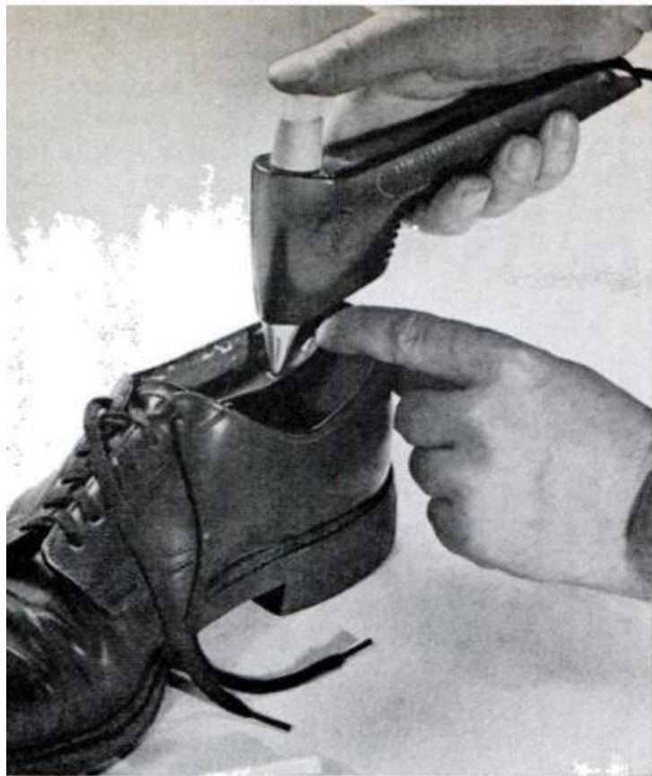
SQUIRT OF HOT-MELT GLUE permanently repairs shoes, leather goods such as chair seat (opposite)
