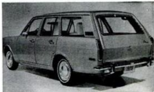
CORTINA from Ford of Britain has a 1600-cc engine with 71 hp, economy close to 30 mpg
