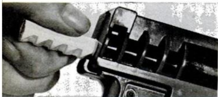
SPECIAL GLUE STICK for Swingline's Auto-Feed has a built-in ratchet; pawl mechanism feeds the sticks
