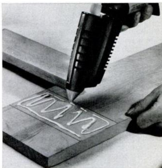
FAST WAY to make strong joints: Apply beads of hot glue and press the parts together within 20 seconds
