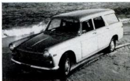
PEUGEOT 404 has a 1.8-liter engine, dual carburetion, ZF automatic transmission option
