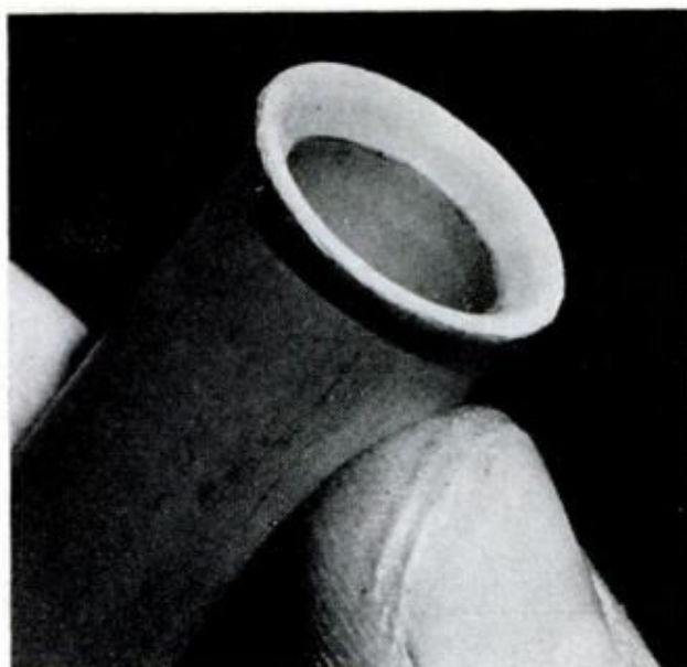
FLARING is frequently useful in water-heater hook-ups; connection is made using standard flare nut
