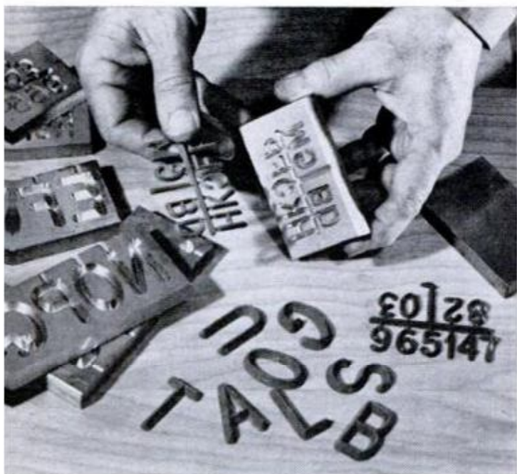
MOLDED LETTERS AND NUMERALS are lifted from mold either singly or in groups, depending on size. Sets of alphabet molds come in \frac{3}{8} and 1\frac{1}{2} -in. letters SEPTEMBER 1970
