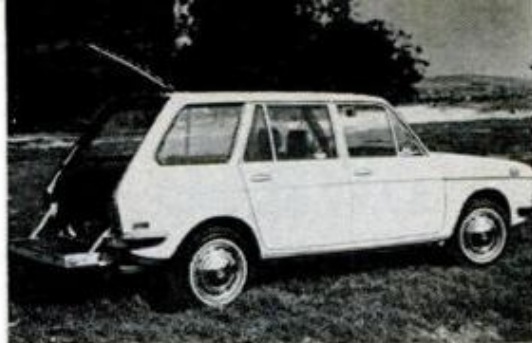
SUBARU STAR has horizontally opposed, four-cylinder, water-cooled engine, top speed of 90
