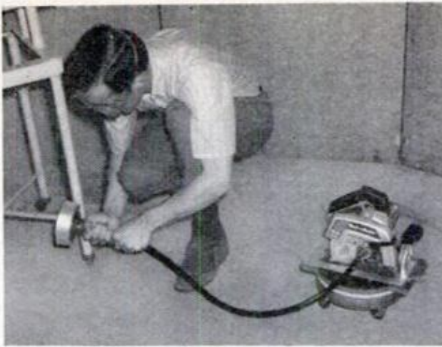
OPERATIONS NEAR FLOOR , such as grinding welds, are a snap because liftoff turntable rolls on casters
