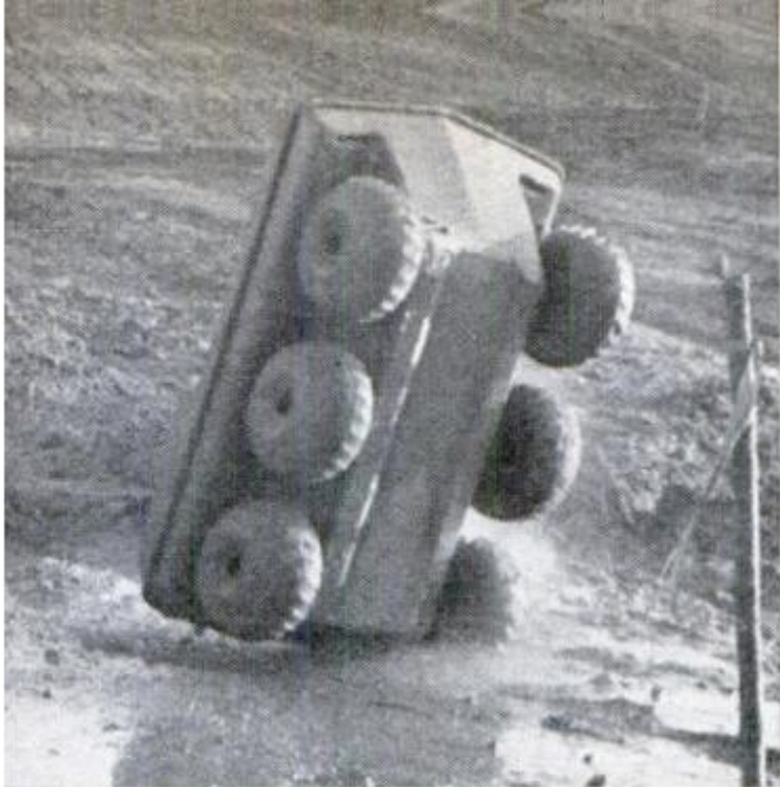
THAT'S US going over on our ear. Unbelted, we flew out unharmed. If belt is worn, roll bar is a must
