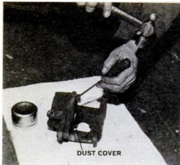
6. AFTER SINGLE-PISTON CALIPER is removed, remove the metal-rimmed dust cover by prying it off
