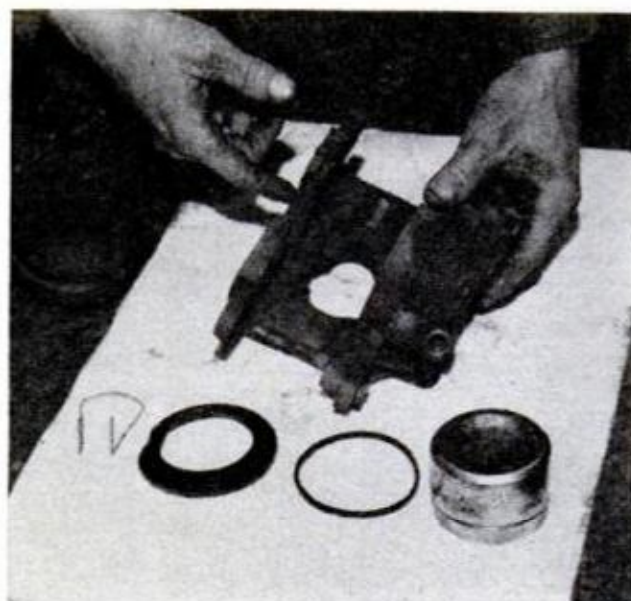
8. PISTON RETAINER, dust cover, O-ring, piston are removed. Rebuild kit has new dust cover, O-ring
