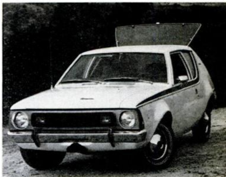
INTERCHANGEABILITY APPROACH is used in Gremlin's sharing basically the same front end as Hornet
