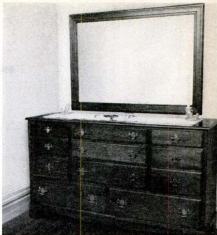
TWO PULLS ARE USED on long drawers, one on short ones. Early American hardware suits finish
