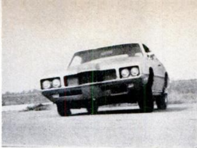
STANDARD RADIAL-PLY TIRES help softly sprung 'Bird corner; there's still understeer and tire scrub
