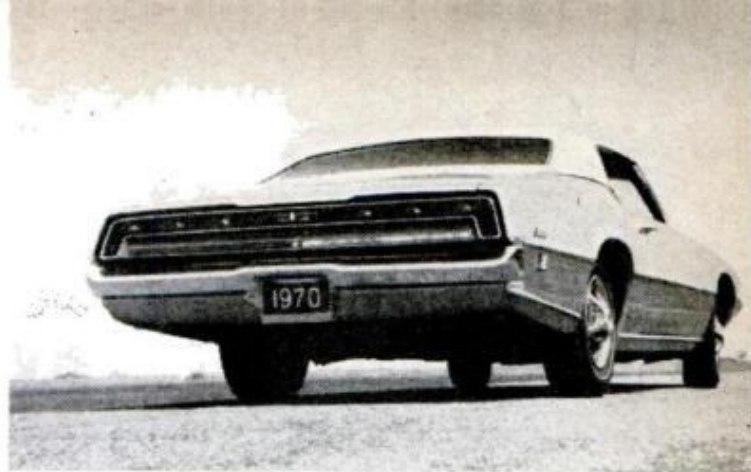
WALL-TO-WALL TAILLIGHTS house sequential turn signals. Backup light is hidden behind center emblem
