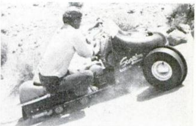
THROWING WEIGHT to the uphill side keeps machine balanced and is the best way to turn up an incline
