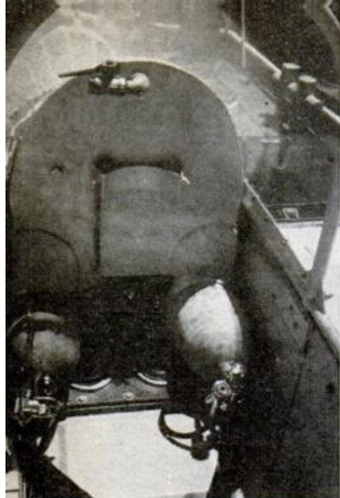
SCUBA TANKS AFT (left) purge wing tanks with compressed air for quick ascent. Joystick and rudder pedals (center) enhance "pilot's" sensation of flying underwater. Through-hull fittings (right) connect the batteries
