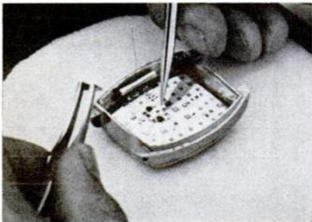
SPECK-SIZED INTEGRATED CIRCUITS are so tiny they must be handled by tweezers under microscope
