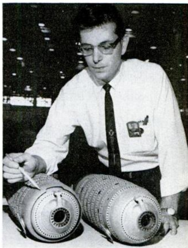
PRATT & WHITNEY ENGINEER indicates annular scoop added to the old combustion chamber (right)
