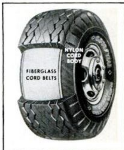
Nyloglas tire: Four nylon cord body plies and two fiberglass belts that extend around the tire to help hold the tread firm and fight squirm.
