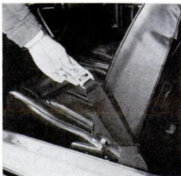
INERTIA CATCH in seatbelt doesn't always reel end back properly, so it catches in door or seat. The seatback release is placed awkwardly near floor
