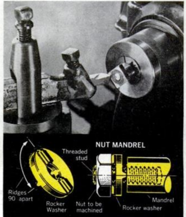
NUT MANDREL can be made of a short length of steel rod with threaded stud at one end to hold nut
