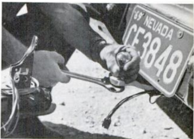
IF YOU WON'T BE USING your trailer ball awhile, best remove it to avoid damage or possible theft
