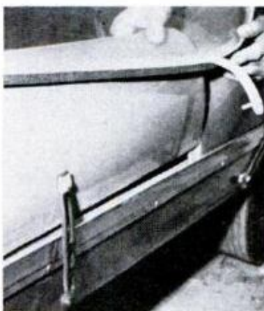
SIDE GLASS is secured in place by aluminum brackets. Several rubber hold-down straps secure front and rear fiberglass panels to unshortened VW chassis
