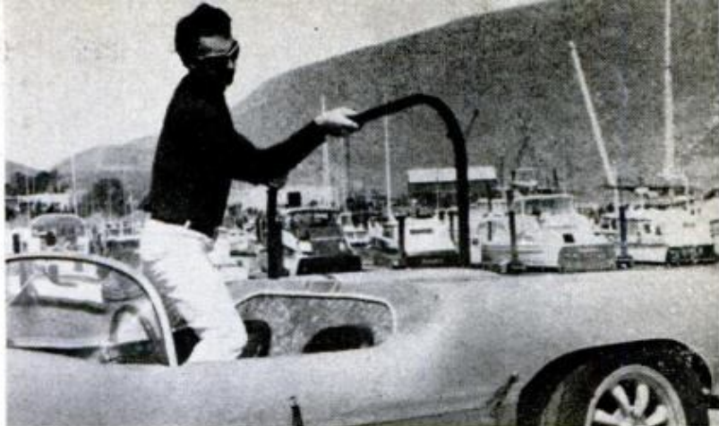
RAGTOP SUPPORT BAR slips through two holes in the rear body panel, can be removed when the top is off
