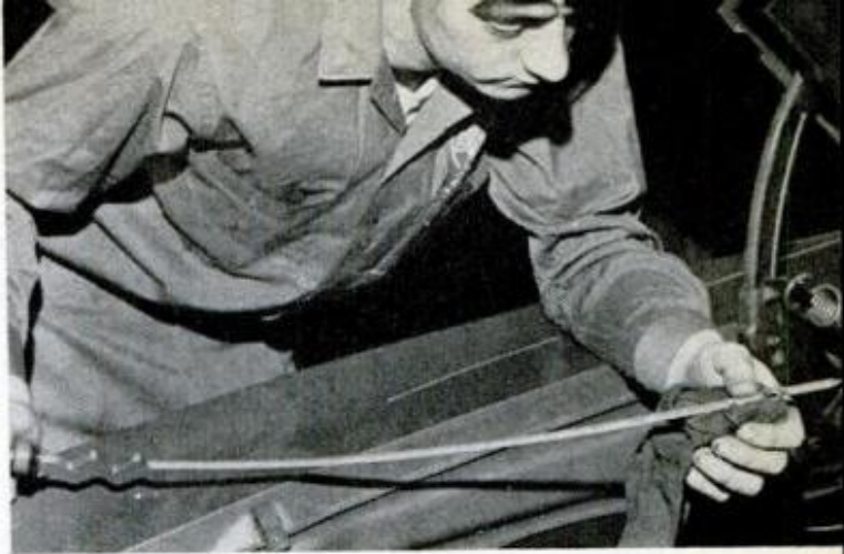
TRANSMISSION FLUID LEVEL is first thing to check. Read dipstick with unit at operating temperature
