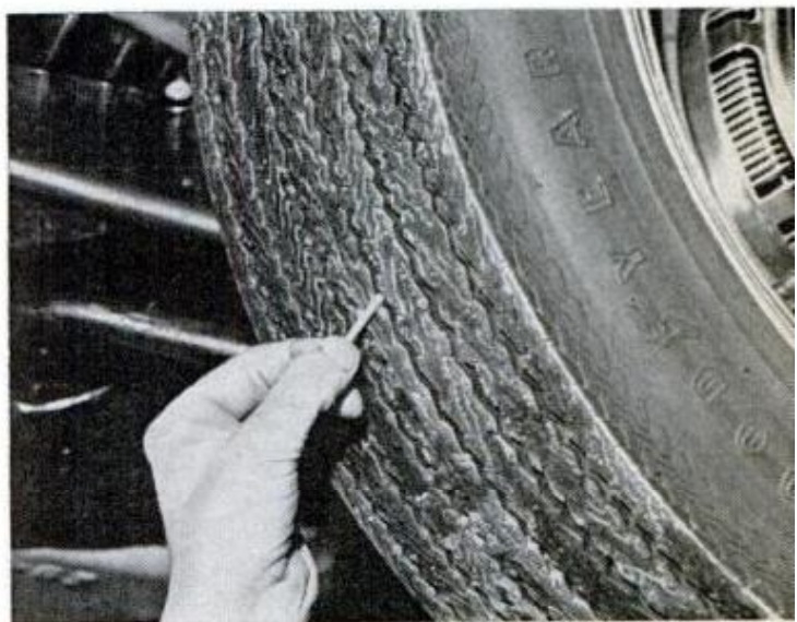
CHECK TREAD for at least \frac{1}{16} -inch remaining; don't wait for tires to go bald. Half a match head is \frac{1}{16} inch
