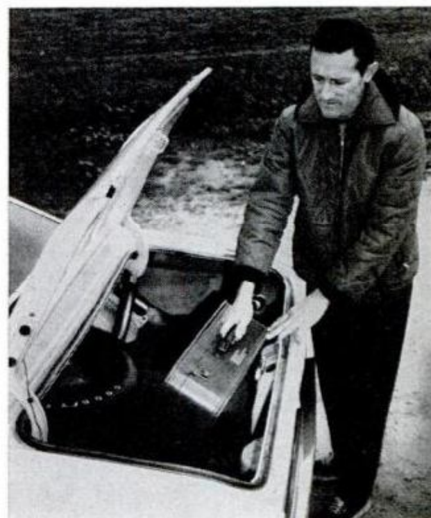
LIKE 'CUDA , Challenger's trunk suffers from gas-fill pipe and spare taking up most of usable space
