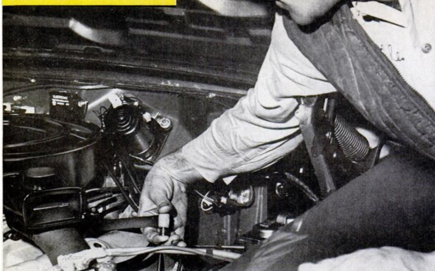
EXHAUST EMISSION VALVE is seated in the engine valve cover of some engines, in the intake manifold or hose lines of others. Pull out the valve, test for adequate vacuum and check condition of the hoses
