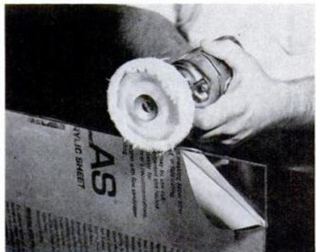
POLISHING. To produce a transparent edge, continue sanding with grits up to 400; buff with compound-coated muslin wheel, later with cotton-flannel wheel
