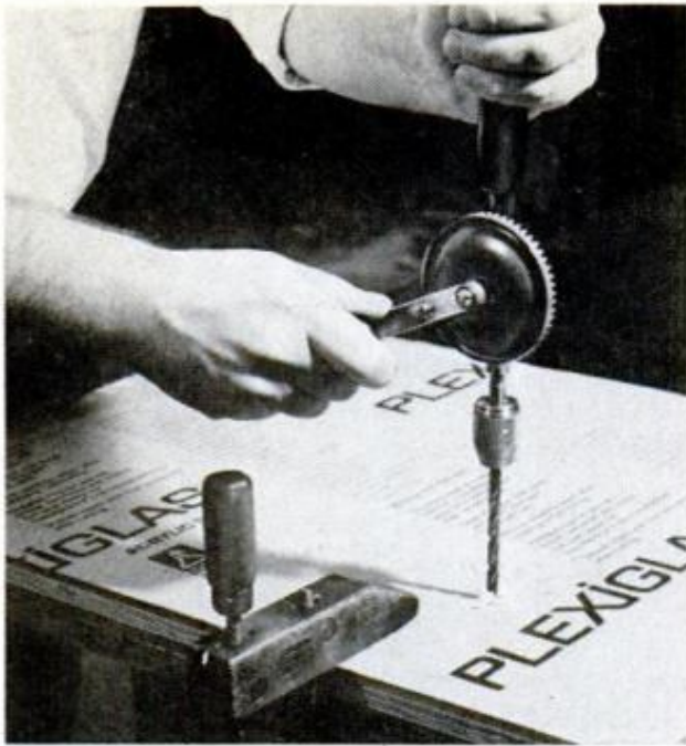
DRILLING. Use regular twist drill, press lightly. Back up work with wood block and clamp. Turn drill slowly to prevent chipping. Don't remove protective paper
