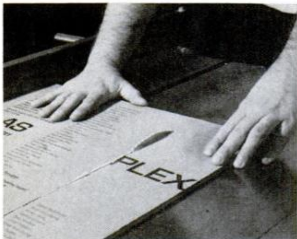
CIRCULAR SAWING. Use fine-tooth "plywood" blade and set blade a little higher than thickness of plastic. Hold work down firmly; push slowly through saw
