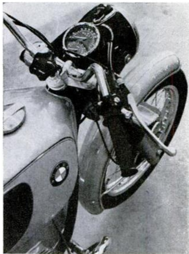
IGNITION SWITCH is in headlight. Instrument cluster includes tach, oil pressure, battery charge lights
