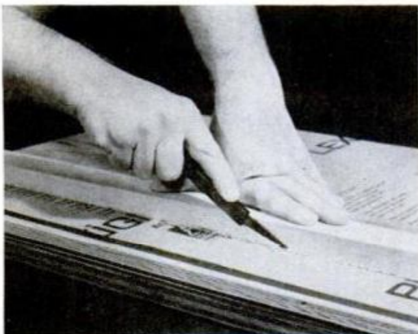
SCRIBING. Plastic up to \frac{1}{8} in. thick can be cut by scoring with pointed tool. Make the score along a straightedge and four or five times through paper
