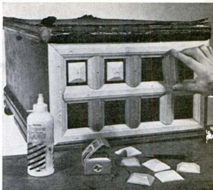
MOLDINGS AT CORNERS are miter-joined; horizontals and verticals inside have 45° bevel undercut
