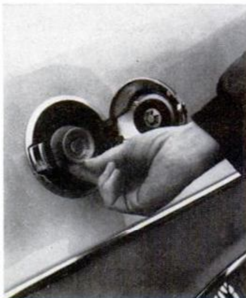
WITHOUT OPTIONAL LOCKING PLUG , gas filler cap can be stolen. Owners also would like cap moved to rear or driver's side
