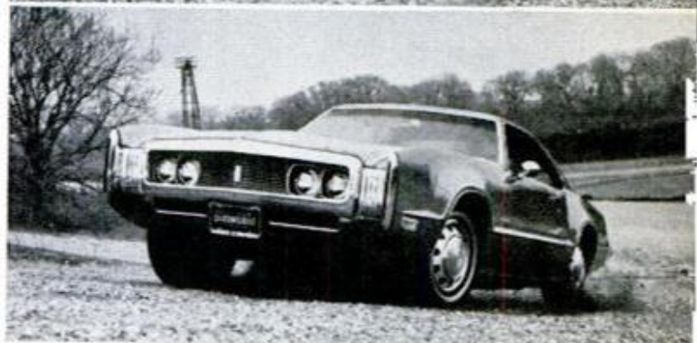
TORONADO'S FRONT DRIVE gets excellent traction due to weight over wheels. Weight transfer going uphill frontwards, though, makes tires spin on gravel
