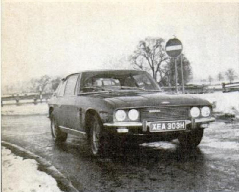
JENSEN INTERCEPTOR , also using Chrysler 383 engine, is two-wheel drive sister-in-skin to the FF
