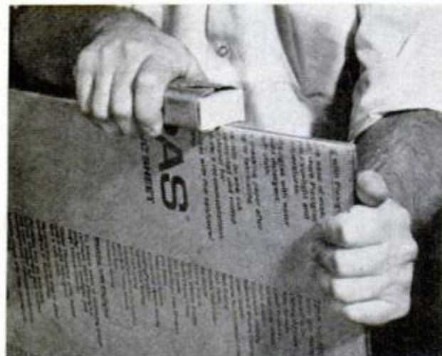
EDGE FINISHING. Saw marks are removed from edges by scraping with knife or by sanding with 60 to 80-grit paper, followed with 150-grit "wet or dry" paper
