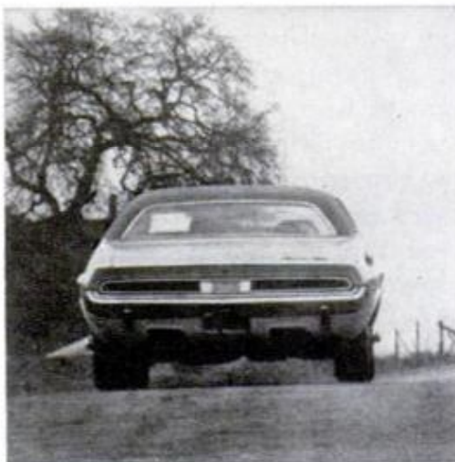
CHALLENGER REAR FENDERS are invisible to short drivers, and many complain of thick A-pillars making backing hazardous
