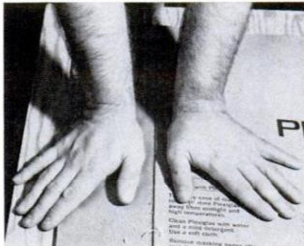
BREAKING. Position score, face up, directly over \frac{3}{4} -in. dowel. Hold sheet with one hand, press down with other. Work along score as breaking continues
