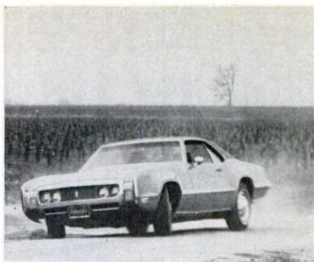
TORONADO PLOWS , understeers, especially if you back off gas; otherwise general handling is good
