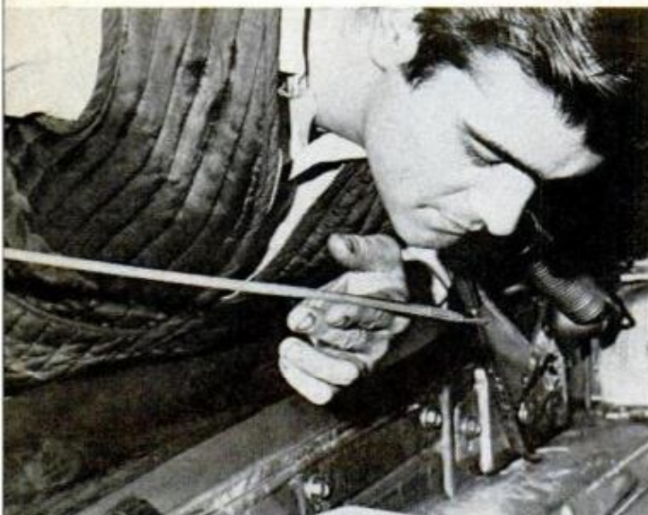
TRANSMISSION DIPSTICK pulls up sample of fluid: a varnish smell or discoloring indicates trouble
