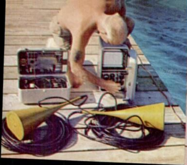
UNDERWATER MAGNETOMETER that is trolled (left) has yellow heads that are dragged in the water. They're attached (by black cables) to the recorder and the power source aboard boat. (Right) Dr. Harold Edgerton with his invention, the "Pinger" sonar, that enabled author to locate two of Columbus's ships. Hand-held underwater magnetometer (below) is used by diver after a wreck has been located to pinpoint metal objects. Previous to its invention, artifacts hidden under just a few inches of sand were generally missed
