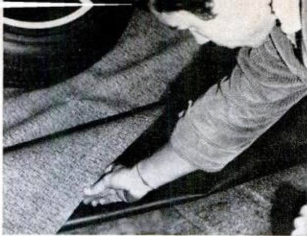
LOOK UNDER MATS for signs of leaks and rust out. Water spots under this one indicate a leaky trunk
