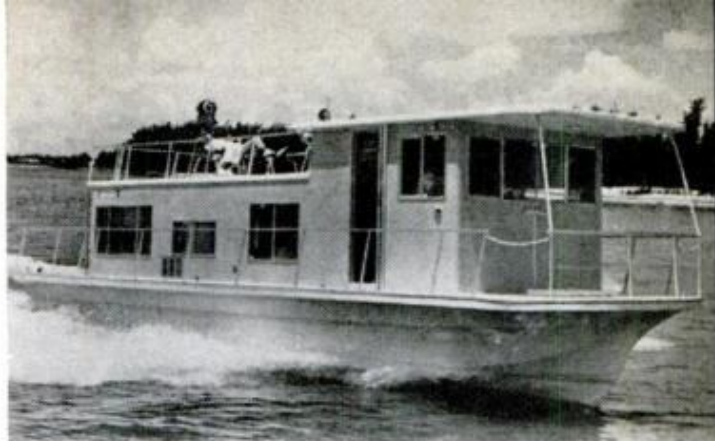
DESPITE ENGINE WEIGHT AFT , most houseboats carry enough weight forward to plane at flat angle
