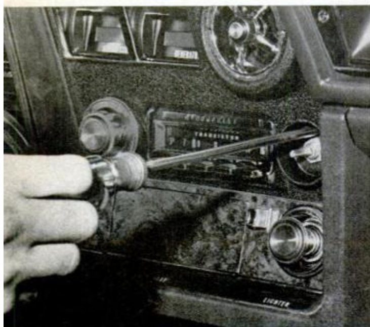
WINDSHIELD ANTENNA , barely visible above, is fast becoming standard equipment. The trimmer adjustment screw is in the radio. On the '70 Olds, it's behind the dial knob. See text for tuning procedure
