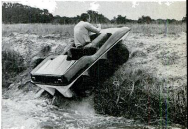
IMAGINE TRYING TO RUN this bank from deep water with family car! Note water draining from jet
