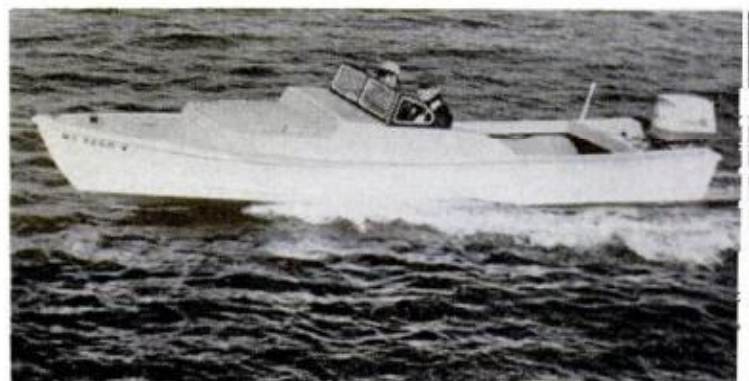
AUTHOR TESTING A BOAT with a relatively long, narrow hull designed to reduce pitching in choppy seas
