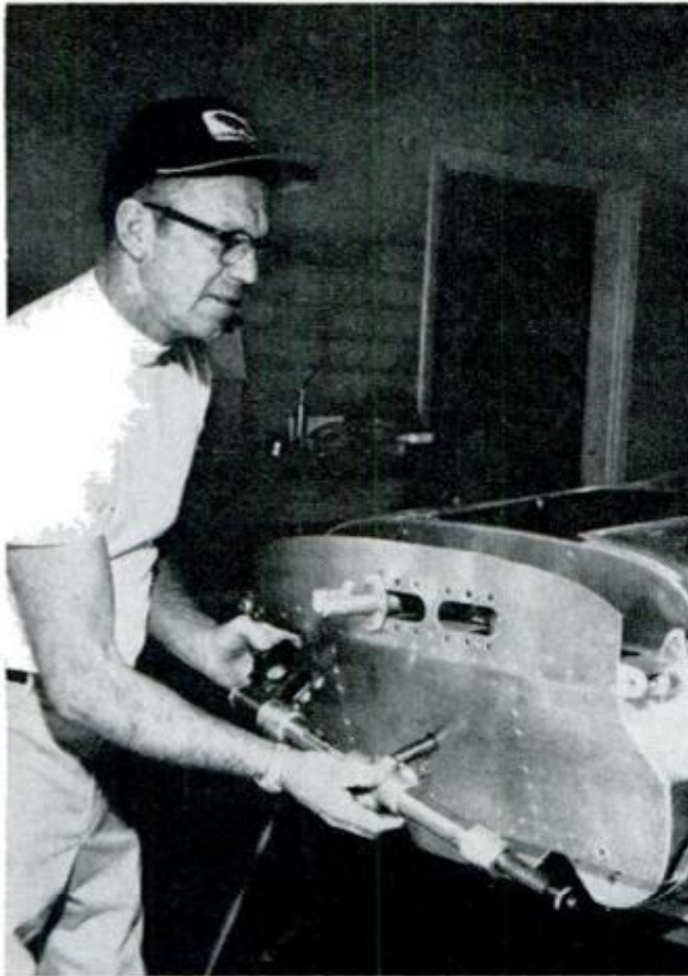
CAR BUILDER CLINT BRAWNER positions steering gear assembled from some of machined parts on workbench. Brawner built the '69 winner, was this far along on new monocoque chassis or "tub" earlier this year
