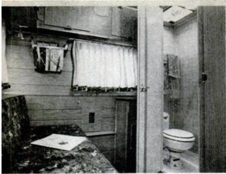
SIDE LOUNGE has colorful, stain-resistant fabric covering 5 inches of foam rubber. Bath has shower with an automatic water heater, marine-type toilet
