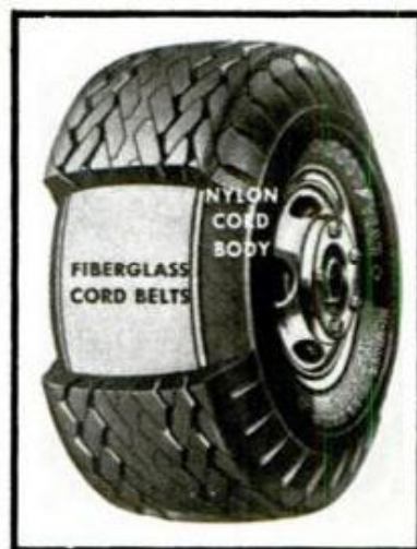
Nyloglas tire: Four nylon cord body plies and two fiberglass belts that extend around the tire to help hold the tread firm and fight squirm.
