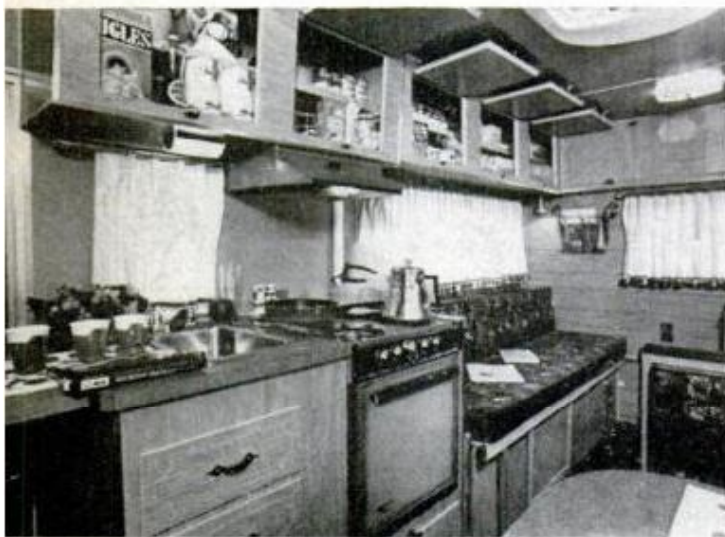
GENEROUS OVERHEAD STORAGE explains angular exterior design. If wall curved to roof line, half of storage would be lost. Magnetic catches hold doors
