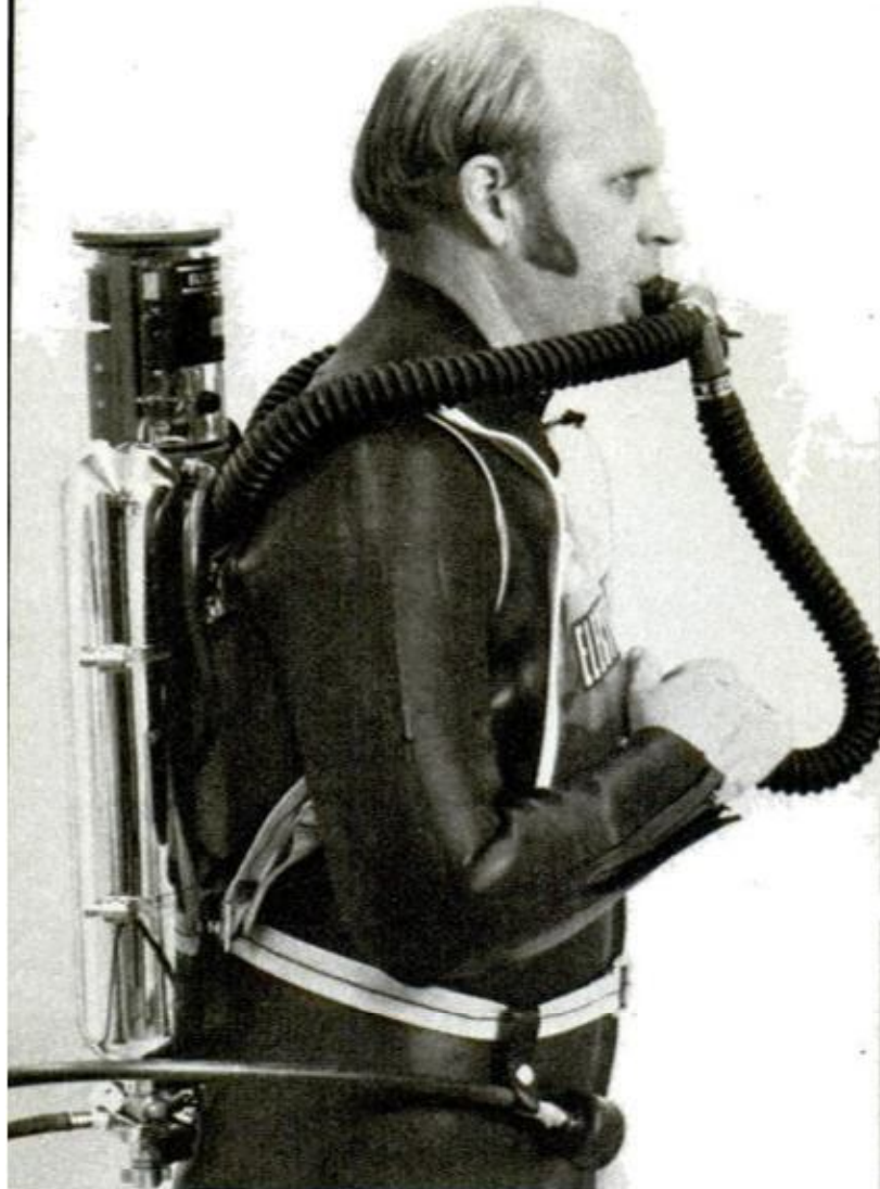
COMPACT, 35-POUND ELECTROLUNG uses gases very efficiently, permits six-hour dives regardless of depth
