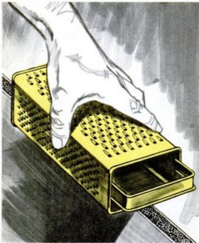
GYPSUM BOARD EDGES can be quickly smoothed or chamfered with the use of a discarded vegetable grater. The type shown has different degrees of coarseness and can be used to best suit the job.—Victor H. Lamoy
