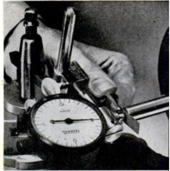
TO MEASURE FOR THICKNESS , contact point is equipped with a shop-made retractor clip made of tin-can material
