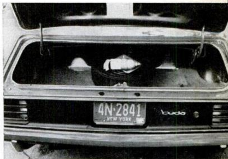
NO TRUNK , moan most owners—a situation not aided by spare being mid-mounted. Lip stands very high
