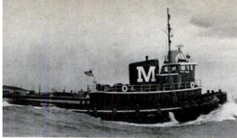
BIG WAKE AND WAVE under tug's stern creates suction on the hull that limits the boat's maximum speed
