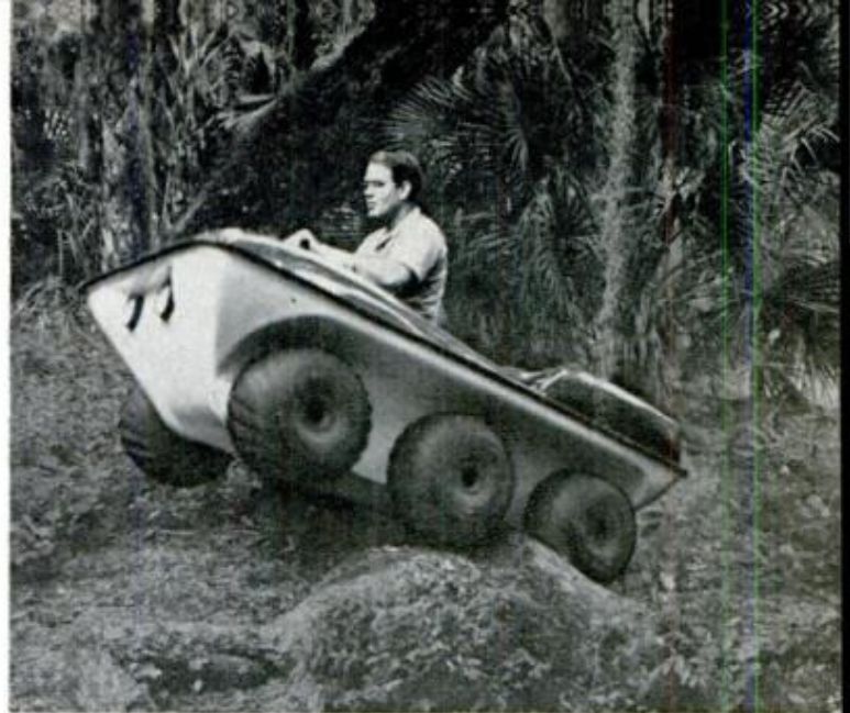
BALLOON TIRES with 1½ pounds air pressure never suffered a puncture in scrambling over rocks and logs
